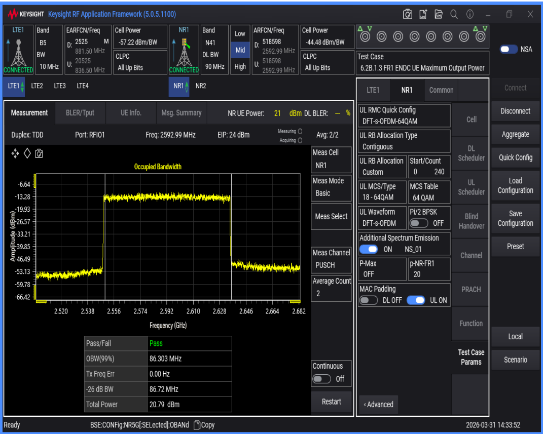
n41 SCS=30kHz DFT_QAM64 BW=50MHz Channel=518598 RB=128@0
