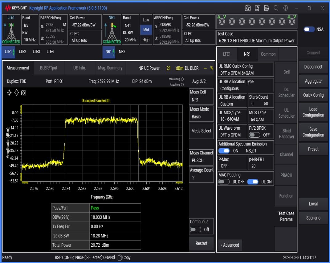
n41 SCS=30kHz DFT_QAM64 BW=100MHz Channel=518598 RB=270@0
