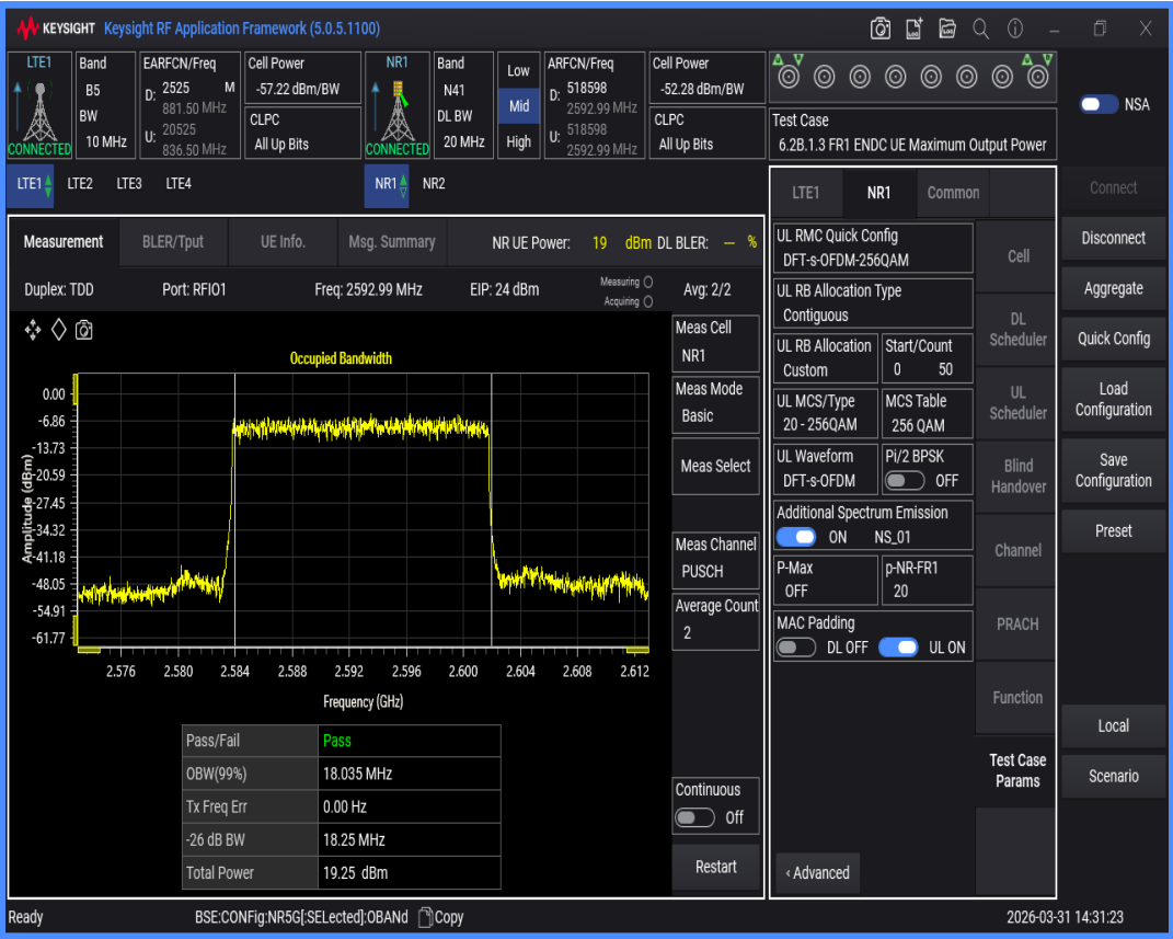
n41 SCS=30kHz DFT_QAM256 BW=90MHz Channel=518598 RB=240@0
