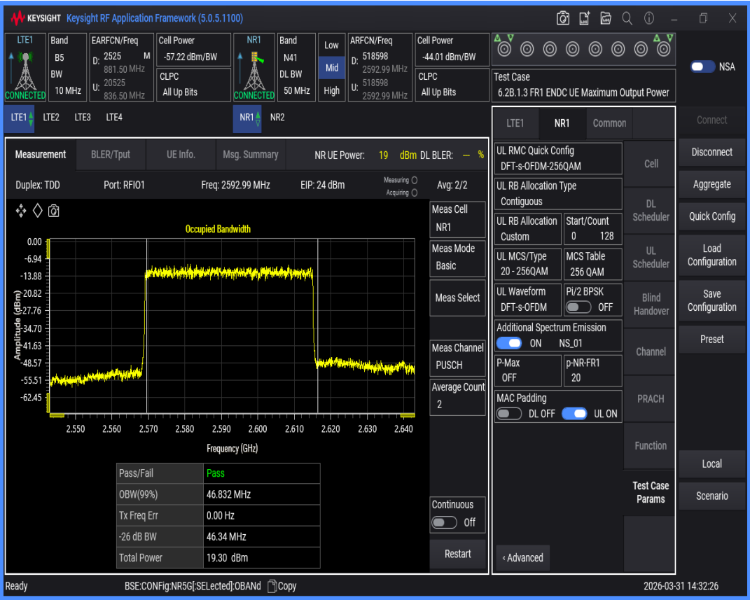
n41 SCS=30kHz DFT_QAM256 BW=100MHz Channel=518598 RB=270@0
