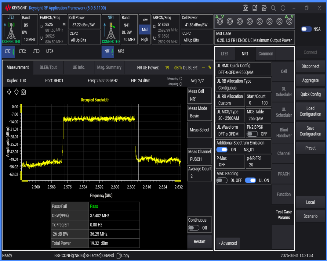
n41 SCS=30kHz DFT_QAM256 BW=50MHz Channel=518598 RB=128@0
