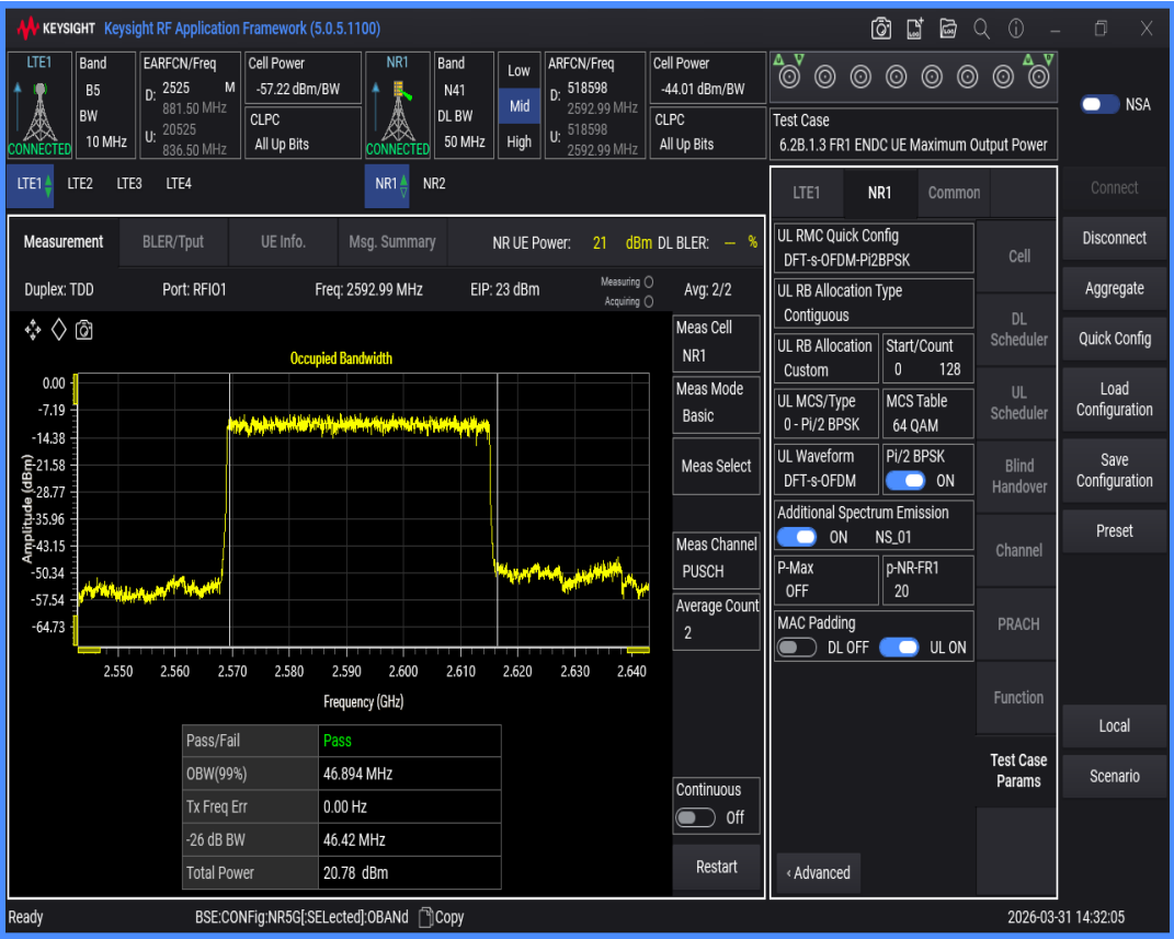
n41 SCS=30kHz DFT_BPSK BW=60MHz Channel=518598 RB=162@0
