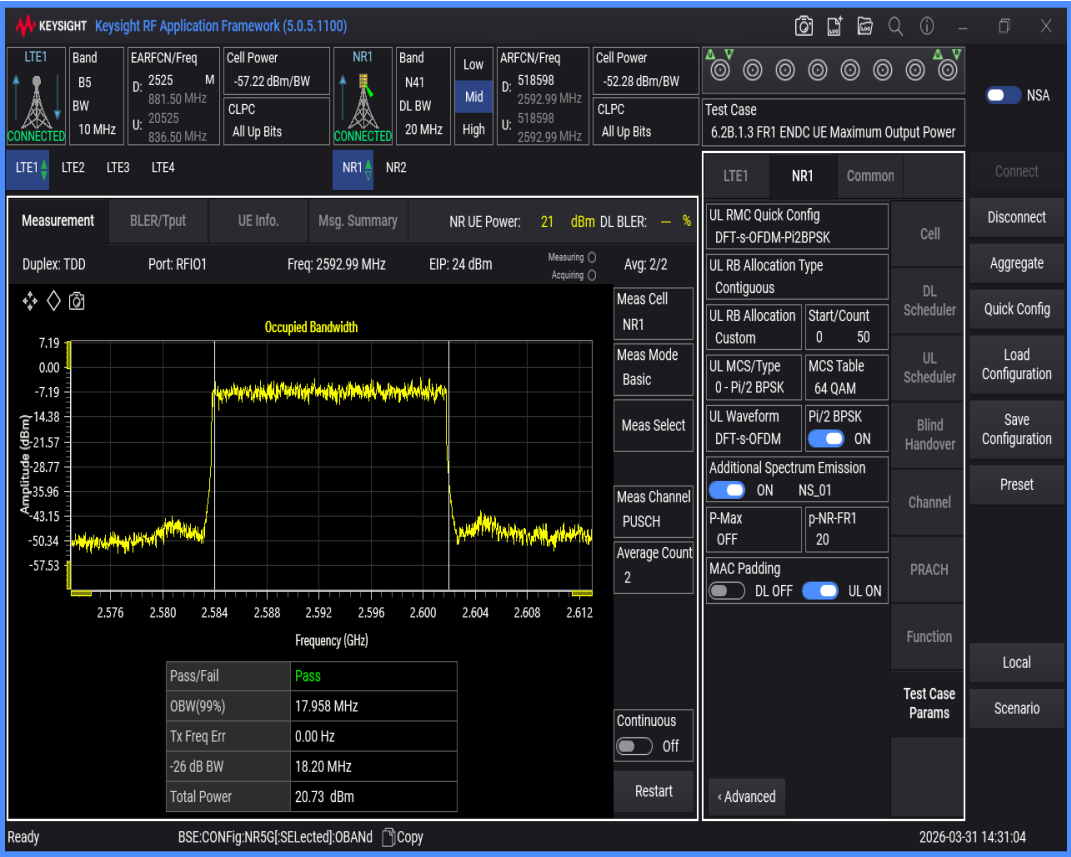
n41 SCS=30kHz DFT_BPSK BW=100MHz Channel=518598 RB=270@0
