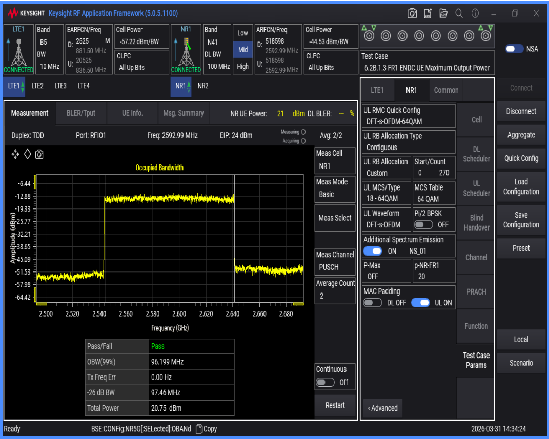
n41 SCS=30kHz DFT_QAM64 BW=80MHz Channel=518598 RB=216@0
