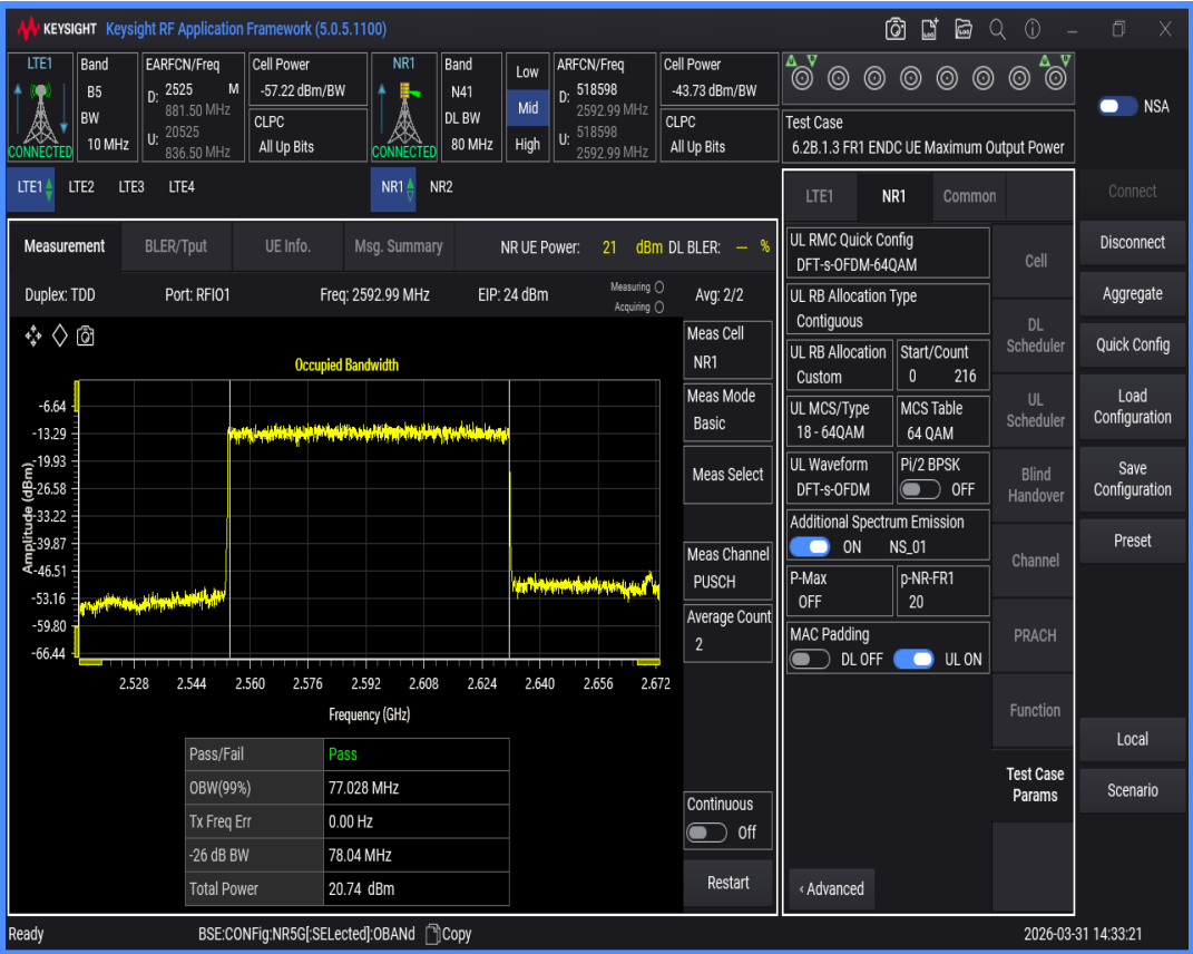
n41 SCS=30kHz DFT_QAM64 BW=90MHz Channel=518598 RB=240@0
