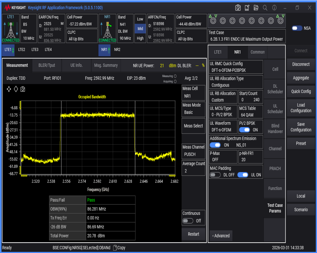
n41 SCS=30kHz DFT_BPSK BW=50MHz Channel=518598 RB=128@0
