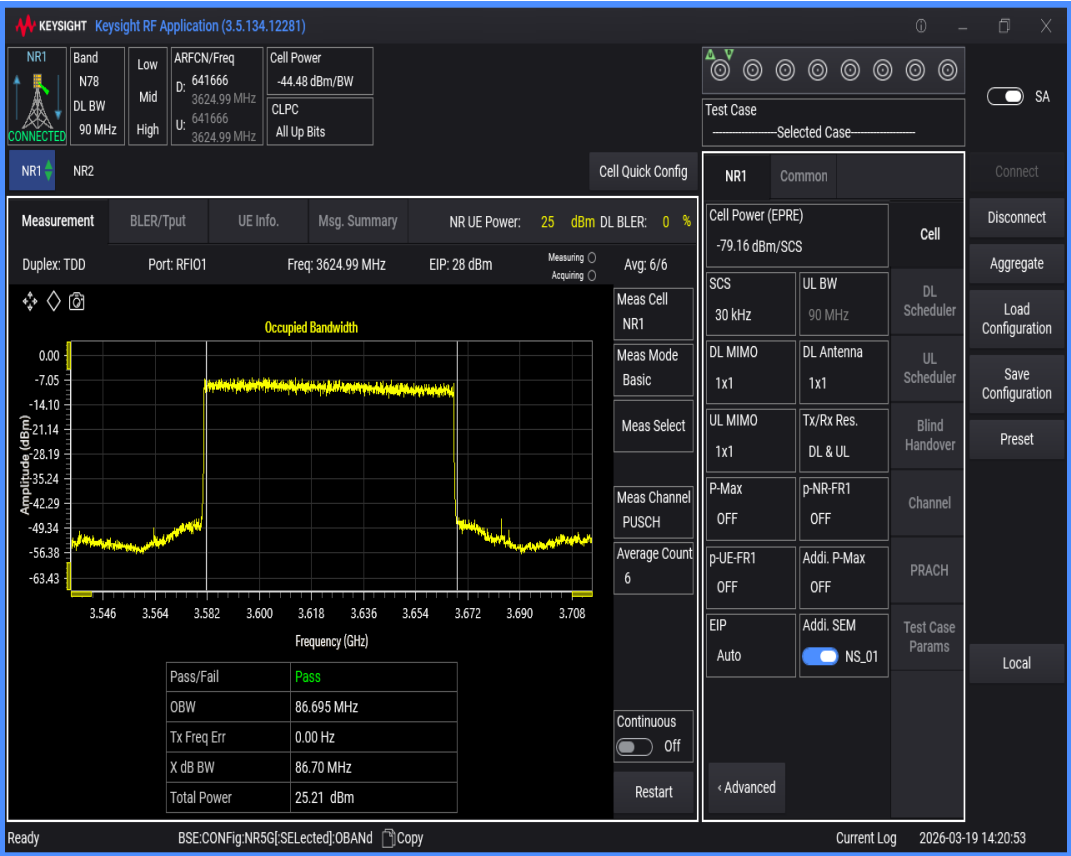
n78(3550-3700) SCS=30kHz DFT_QAM16 BW=100MHz Channel=641666 RB=270@0
