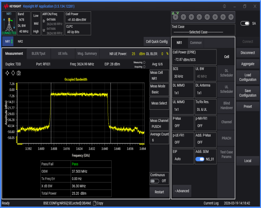
n78(3550-3700) SCS=30kHz DFT_BPSK BW=50MHz Channel=641666 RB=128@0
