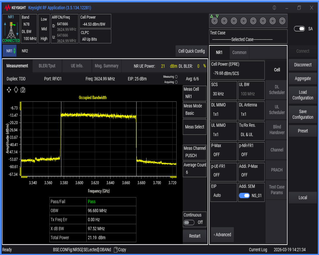
n78(3550-3700) SCS=30kHz DFT_QAM16 BW=90MHz Channel=641666 RB=240@0
