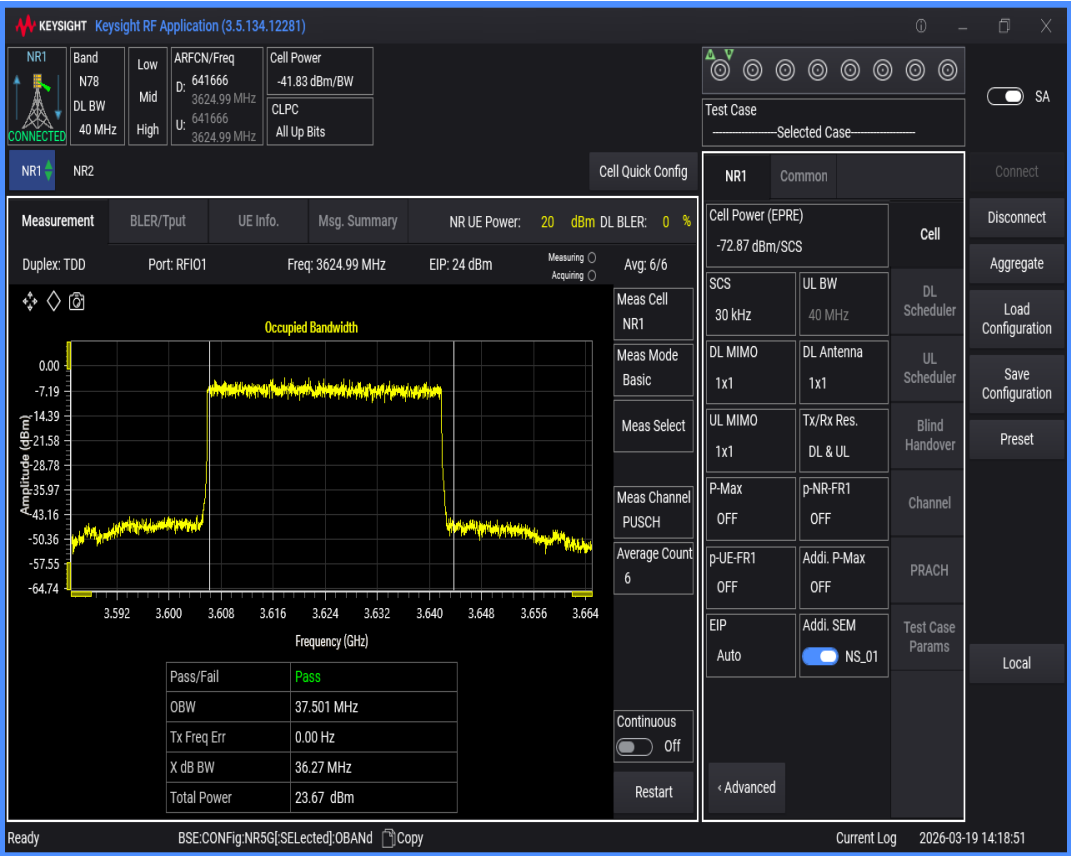
n78(3550-3700) SCS=30kHz DFT_QAM16 BW=60MHz Channel=641666 RB=162@0
