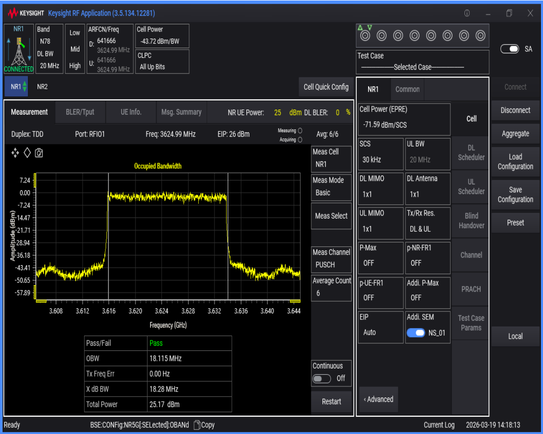
n78(3550-3700) SCS=30kHz DFT_BPSK BW=40MHz Channel=641666 RB=100@0
