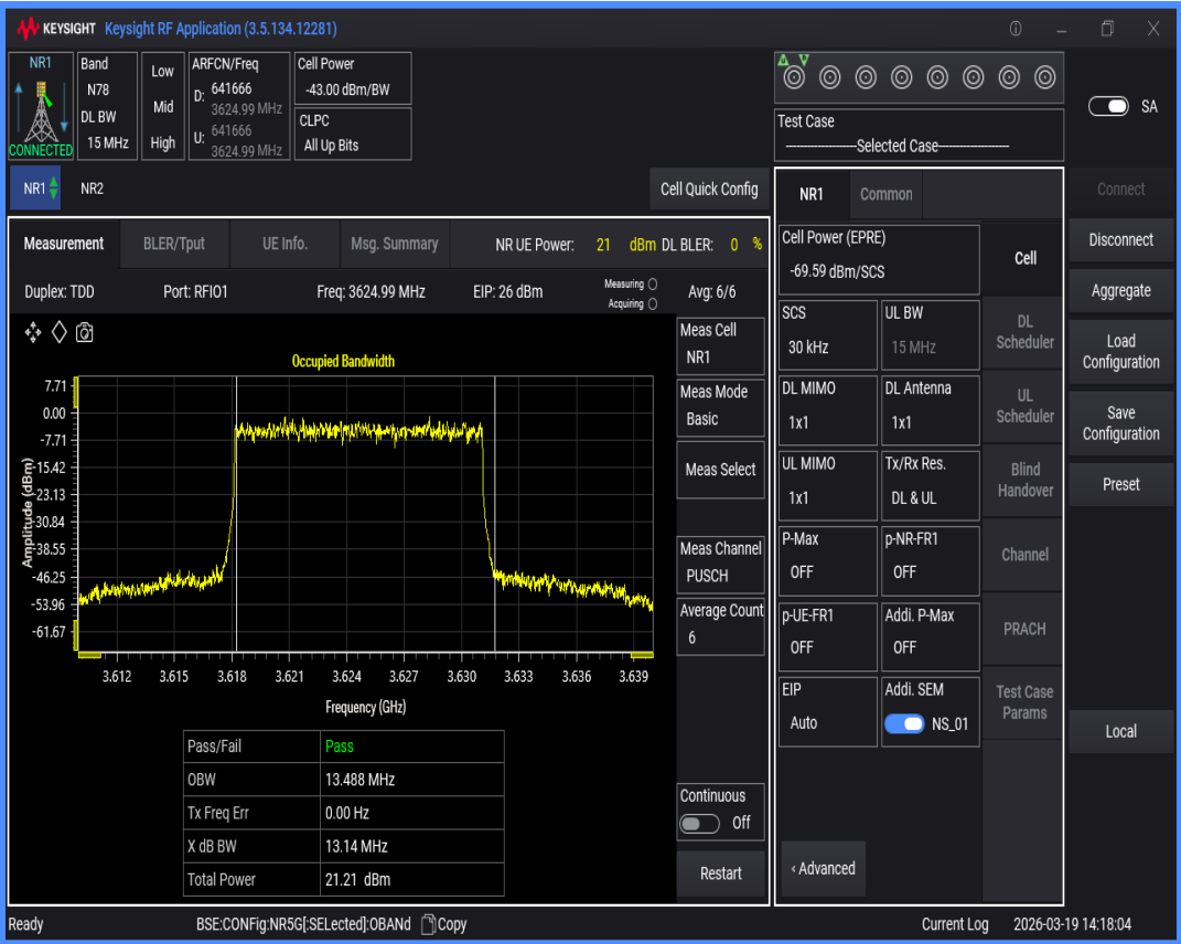
n78(3550-3700) SCS=30kHz DFT_QAM256 BW=50MHz Channel=641666 RB=128@0
