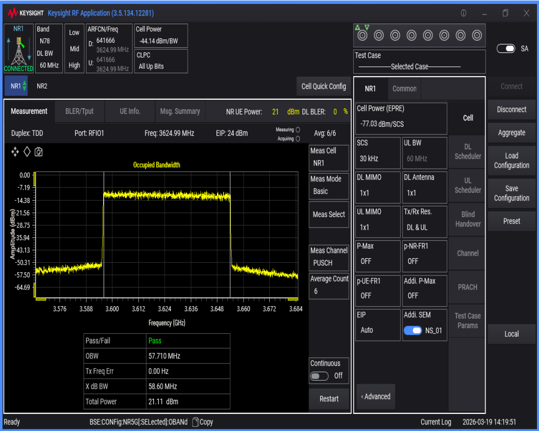
n78(3550-3700) SCS=30kHz DFT_QAM256 BW=80MHz Channel=641666 RB=216@0
