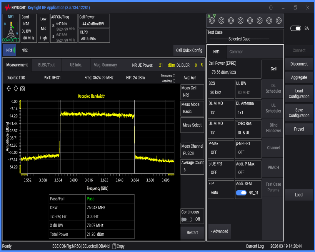
n78(3550-3700) SCS=30kHz DFT_QAM256 BW=90MHz Channel=641666 RB=240@0
