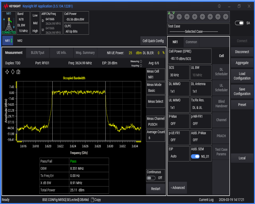
n78(3550-3700) SCS=30kHz DFT_BPSK BW=15MHz Channel=641666 RB=36@0
