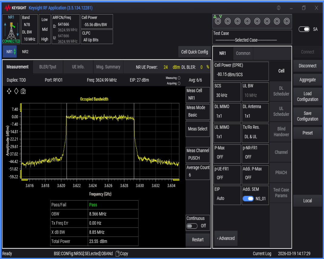
n78(3550-3700) SCS=30kHz DFT_QAM16 BW=15MHz Channel=641666 RB=36@0
