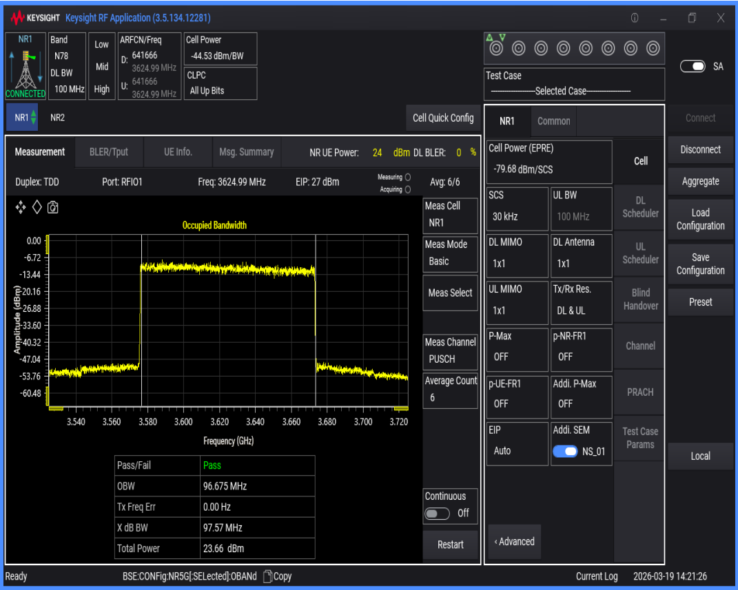
n78(3550-3700) SCS=30kHz DFT_QAM16 BW=10MHz Channel=641666 RB=24@0
