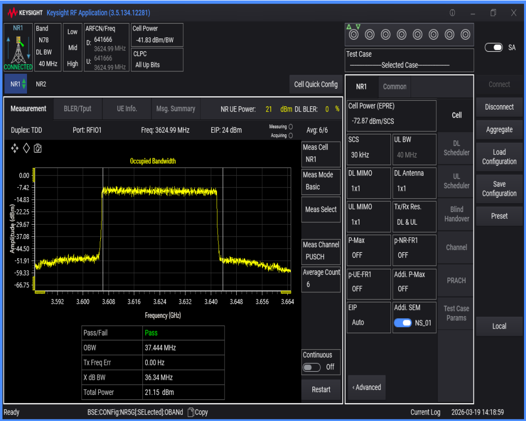
n78(3550-3700) SCS=30kHz DFT_QAM256 BW=70MHz Channel=641666 RB=180@0
