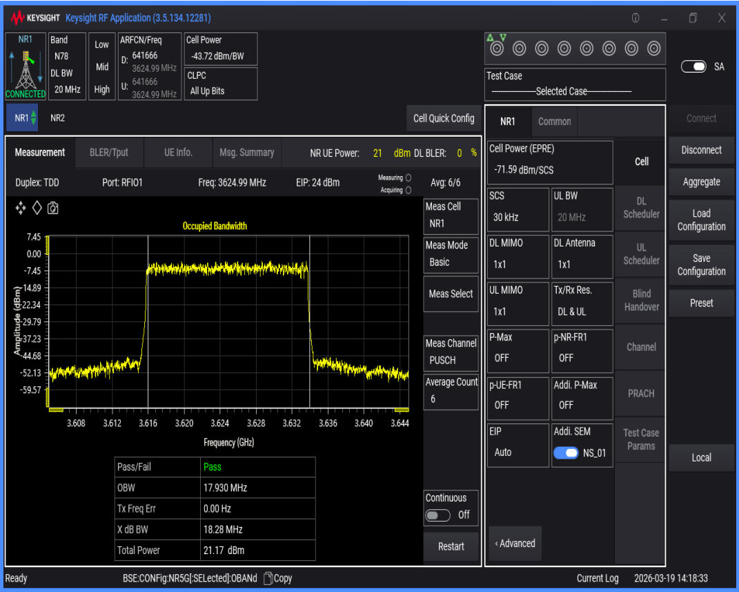
n78(3550-3700) SCS=30kHz DFT_QAM256 BW=15MHz Channel=641666 RB=36@0
