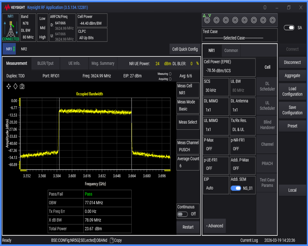
n78(3550-3700) SCS=30kHz DFT_QAM256 BW=100MHz Channel=641666 RB=270@0
