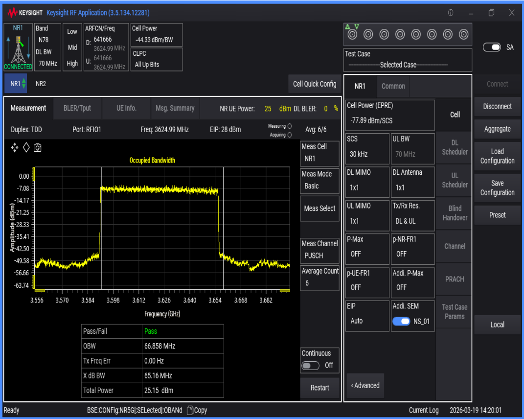
n78(3550-3700) SCS=30kHz DFT_BPSK BW=80MHz Channel=641666 RB=216@0
