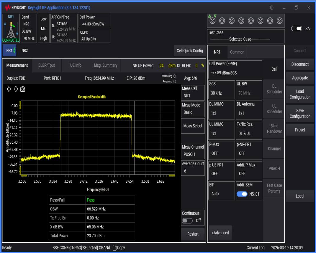
n78(3550-3700) SCS=30kHz DFT_QAM16 BW=80MHz Channel=641666 RB=216@0
