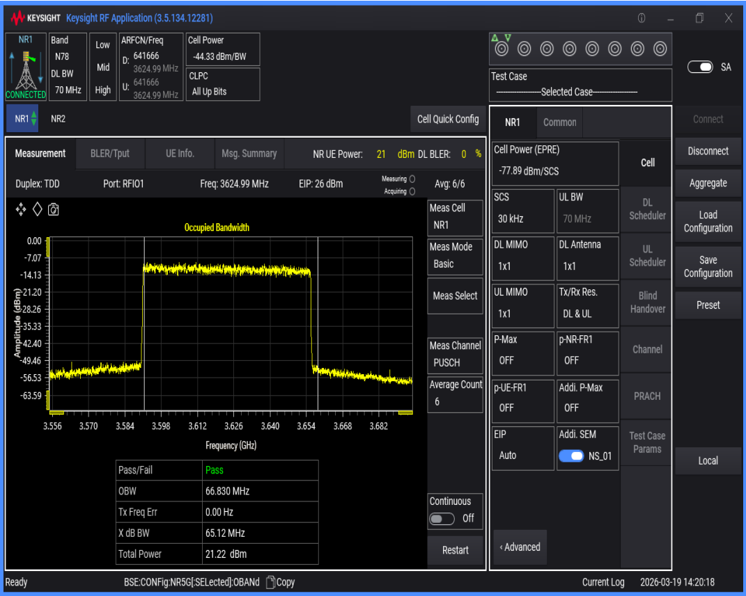
n78(3550-3700) SCS=30kHz DFT_QAM256 BW=60MHz Channel=641666 RB=162@0
