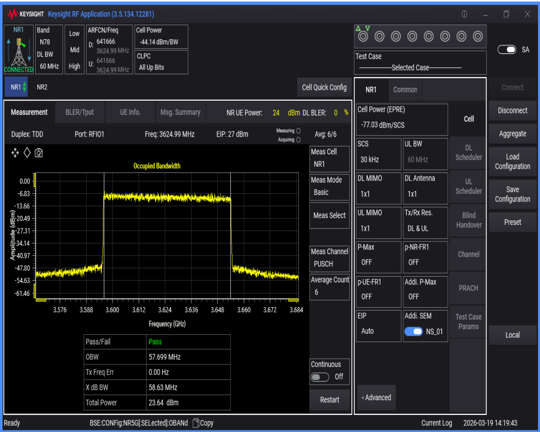
n78(3550-3700) SCS=30kHz DFT_QAM16 BW=70MHz Channel=641666 RB=180@0
