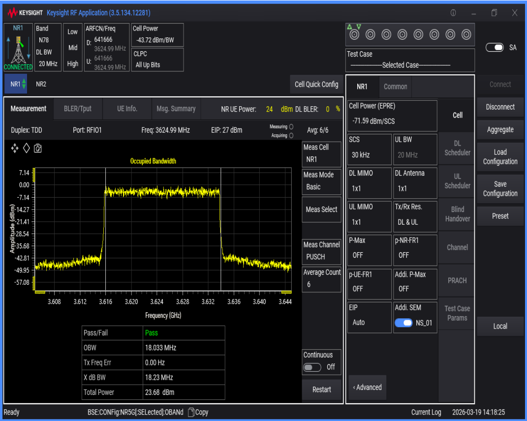
n78(3550-3700) SCS=30kHz DFT_QAM16 BW=50MHz Channel=641666 RB=128@0
