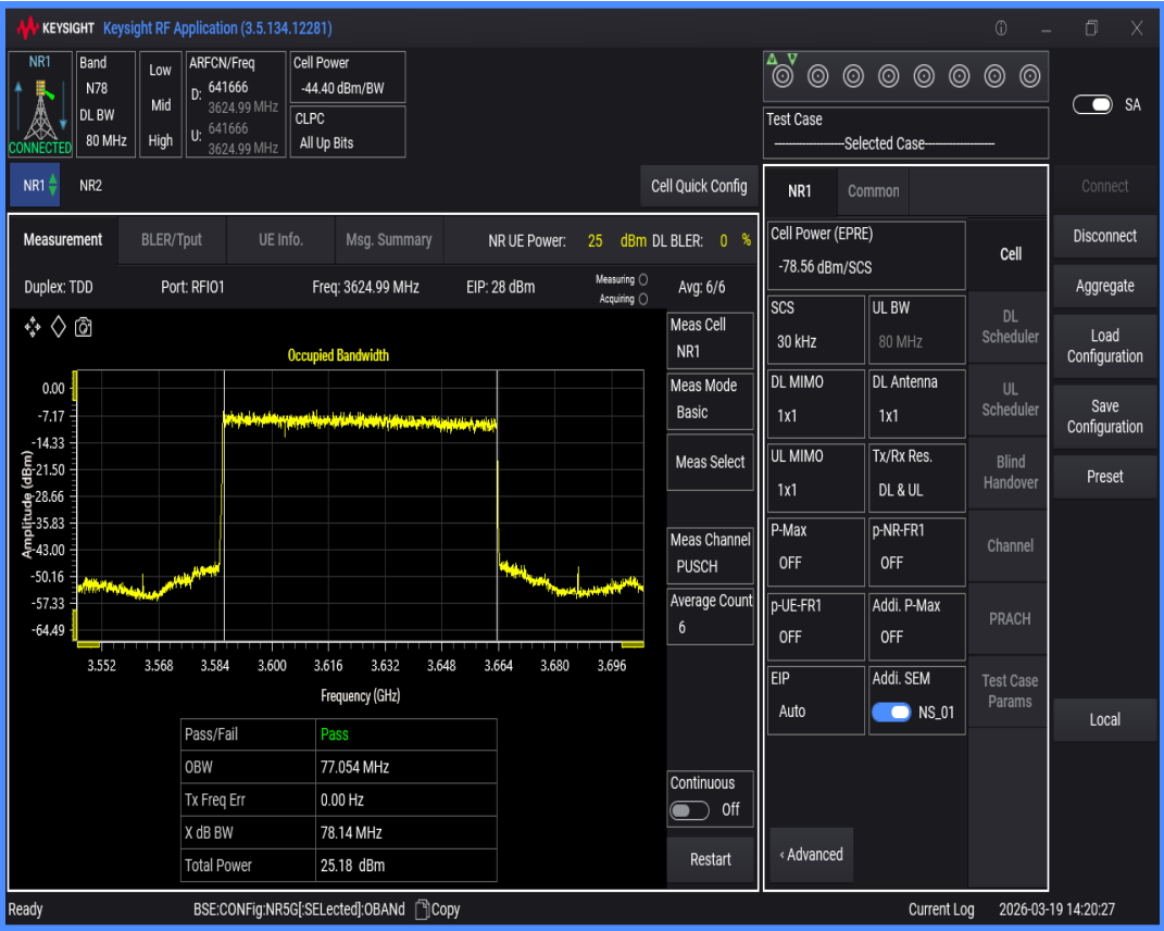
n78(3550-3700) SCS=30kHz DFT_BPSK BW=90MHz Channel=641666 RB=240@0
