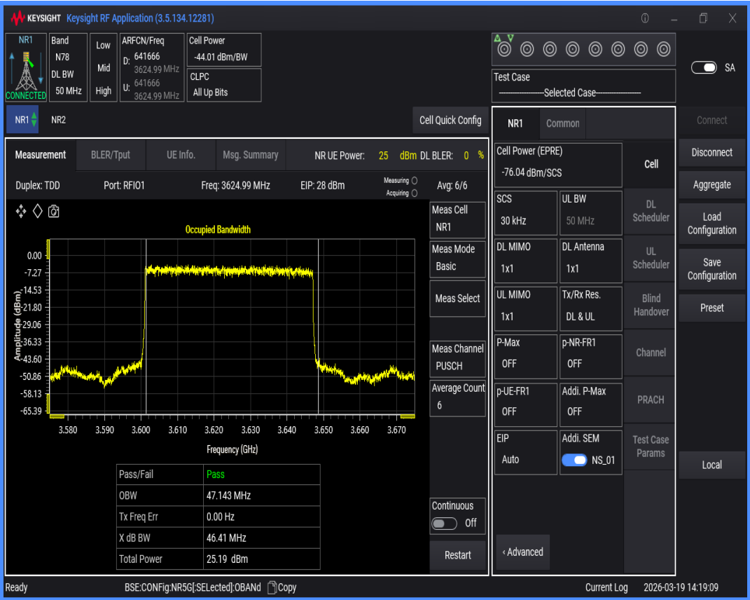
n78(3550-3700) SCS=30kHz DFT_BPSK BW=60MHz Channel=641666 RB=162@0
