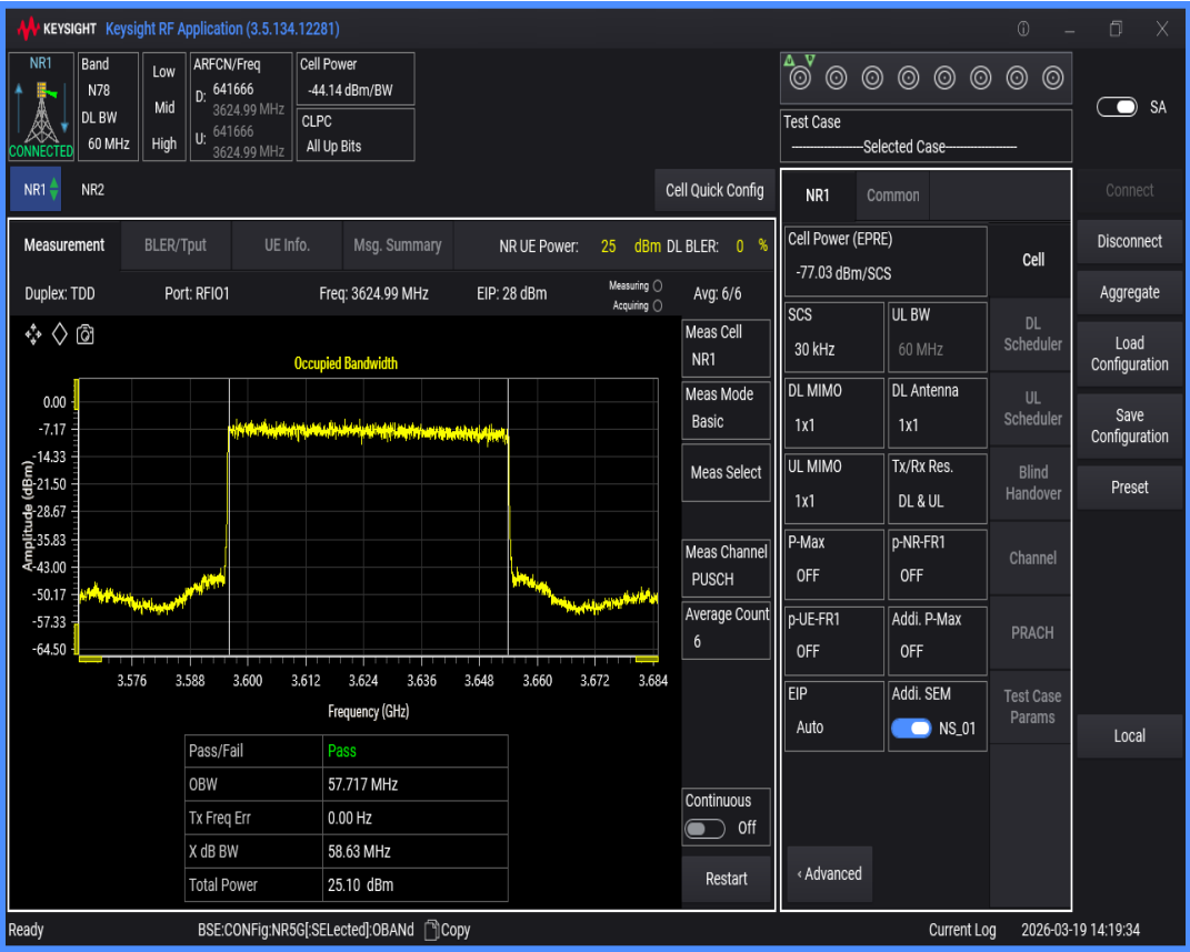
n78(3550-3700) SCS=30kHz DFT_BPSK BW=70MHz Channel=641666 RB=180@0
