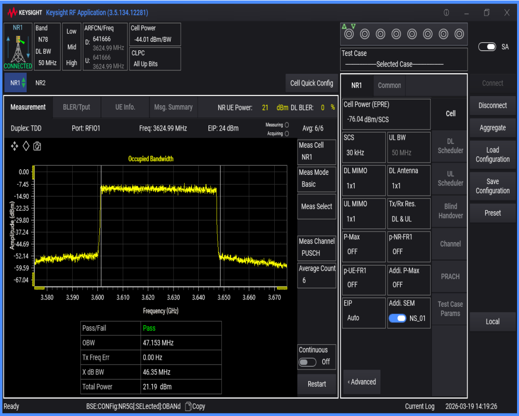
n78(3550-3700) SCS=30kHz DFT_QAM256 BW=40MHz Channel=641666 RB=100@0
