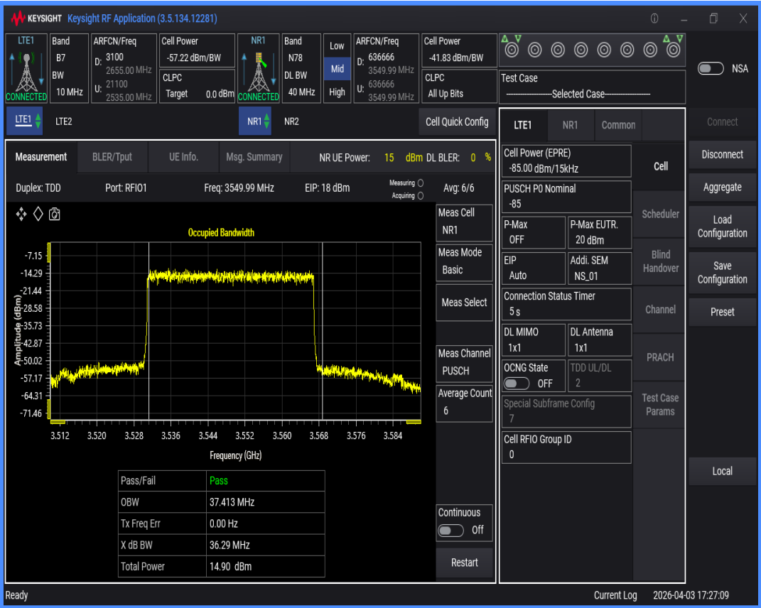
n78 SCS=30kHz DFT_QAM256 BW=90MHz Channel=636666 RB=240@0
