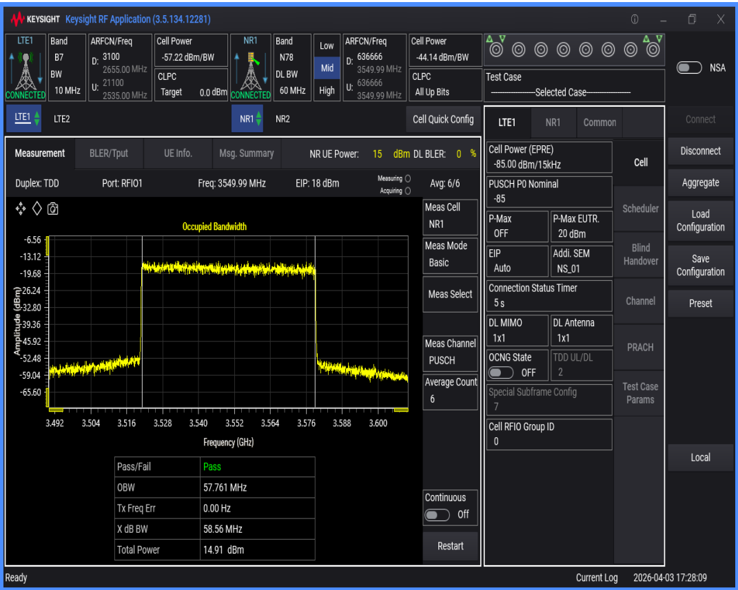
n78 SCS=30kHz DFT_QAM256 BW=80MHz Channel=636666 RB=216@0
