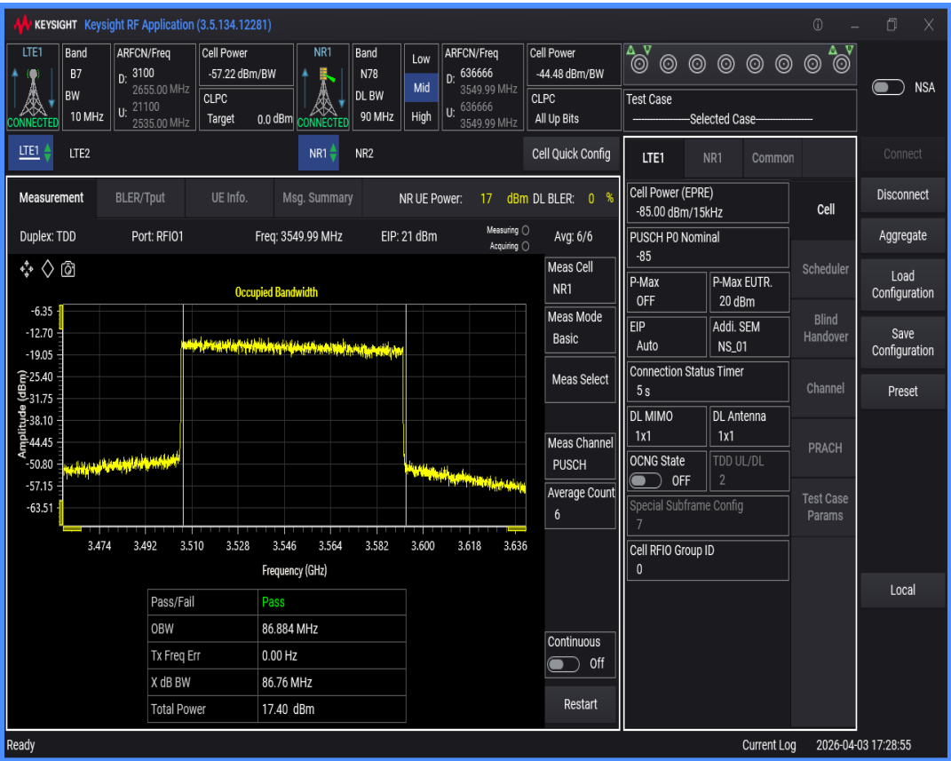
n78 SCS=30kHz DFT_QAM256 BW=100MHz Channel=636666 RB=270@0
