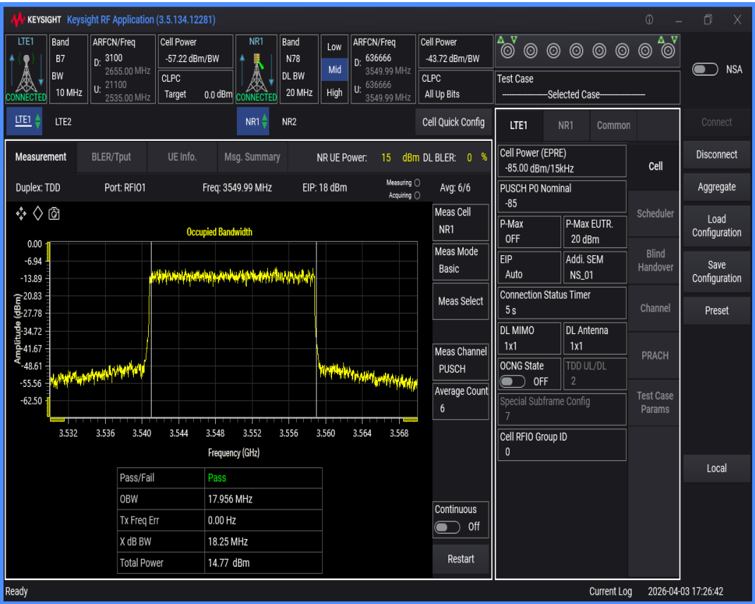
n78 SCS=30kHz DFT_QAM256 BW=10MHz Channel=636666 RB=24@0
