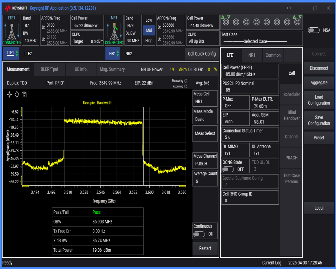
n78 SCS=30kHz DFT_QAM16 BW=15MHz Channel=636666 RB=36@0
