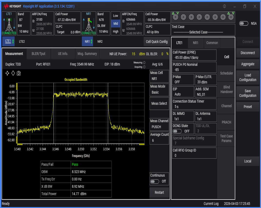
n78 SCS=30kHz DFT_QAM16 BW=90MHz Channel=636666 RB=240@0
