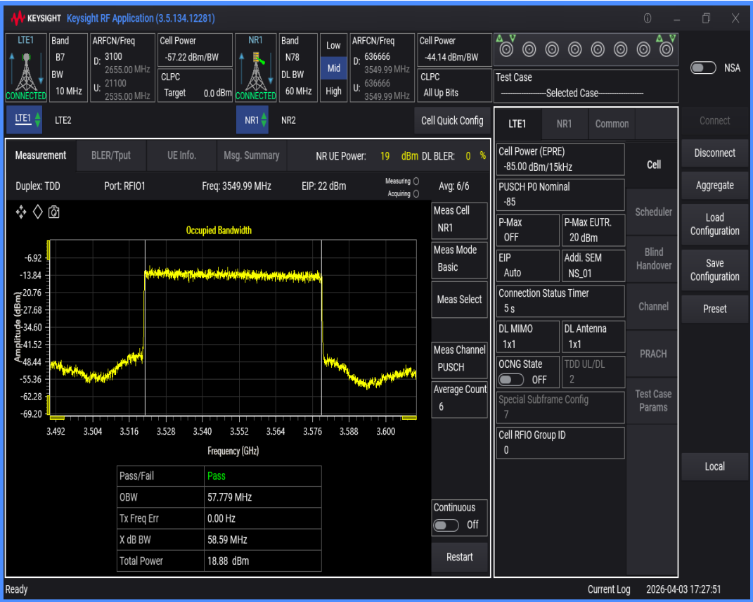
n78 SCS=30kHz DFT_BPSK BW=90MHz Channel=636666 RB=240@0
