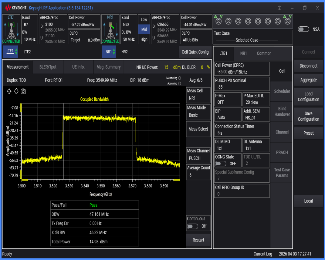
n78 SCS=30kHz DFT_QAM256 BW=40MHz Channel=636666 RB=100@0
