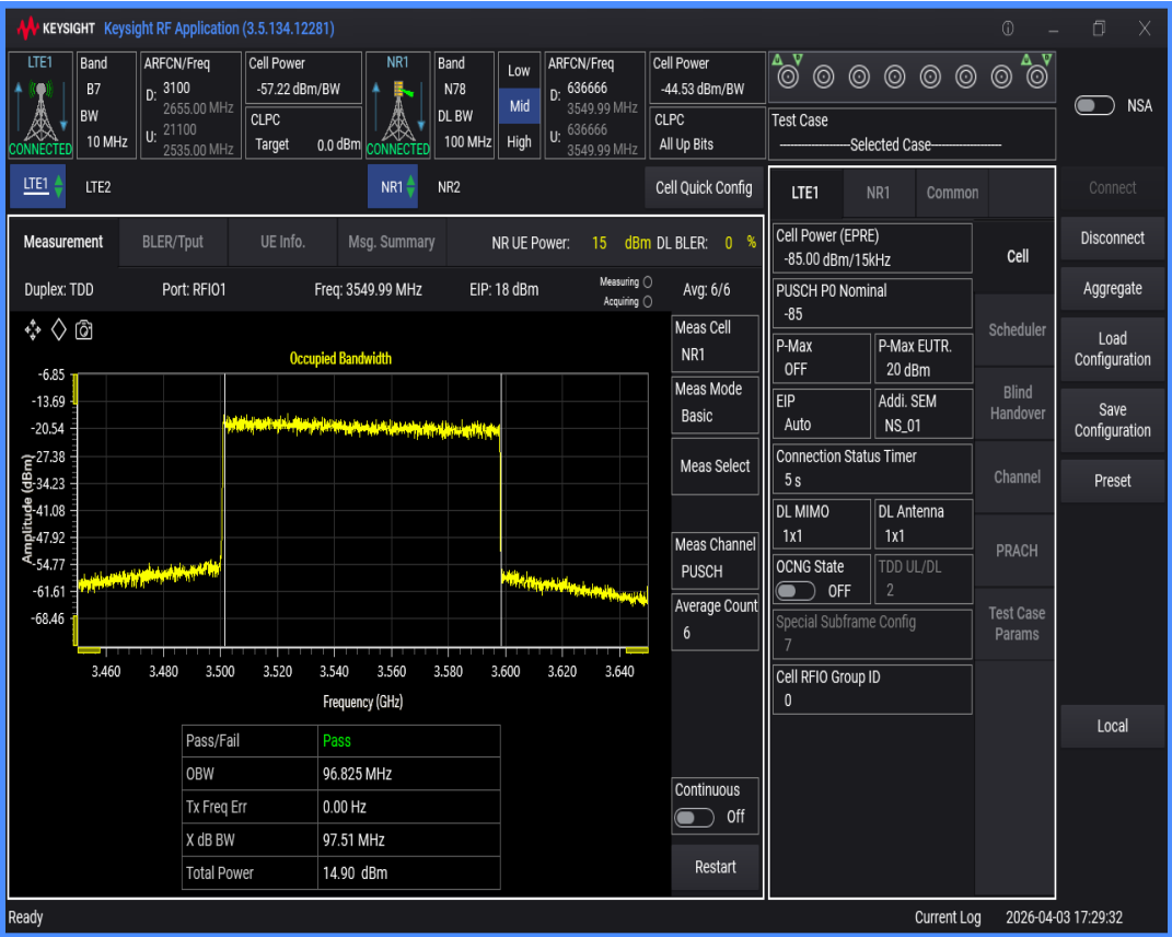
n78 SCS=30kHz DFT_QAM256 BW=50MHz Channel=636666 RB=128@0
