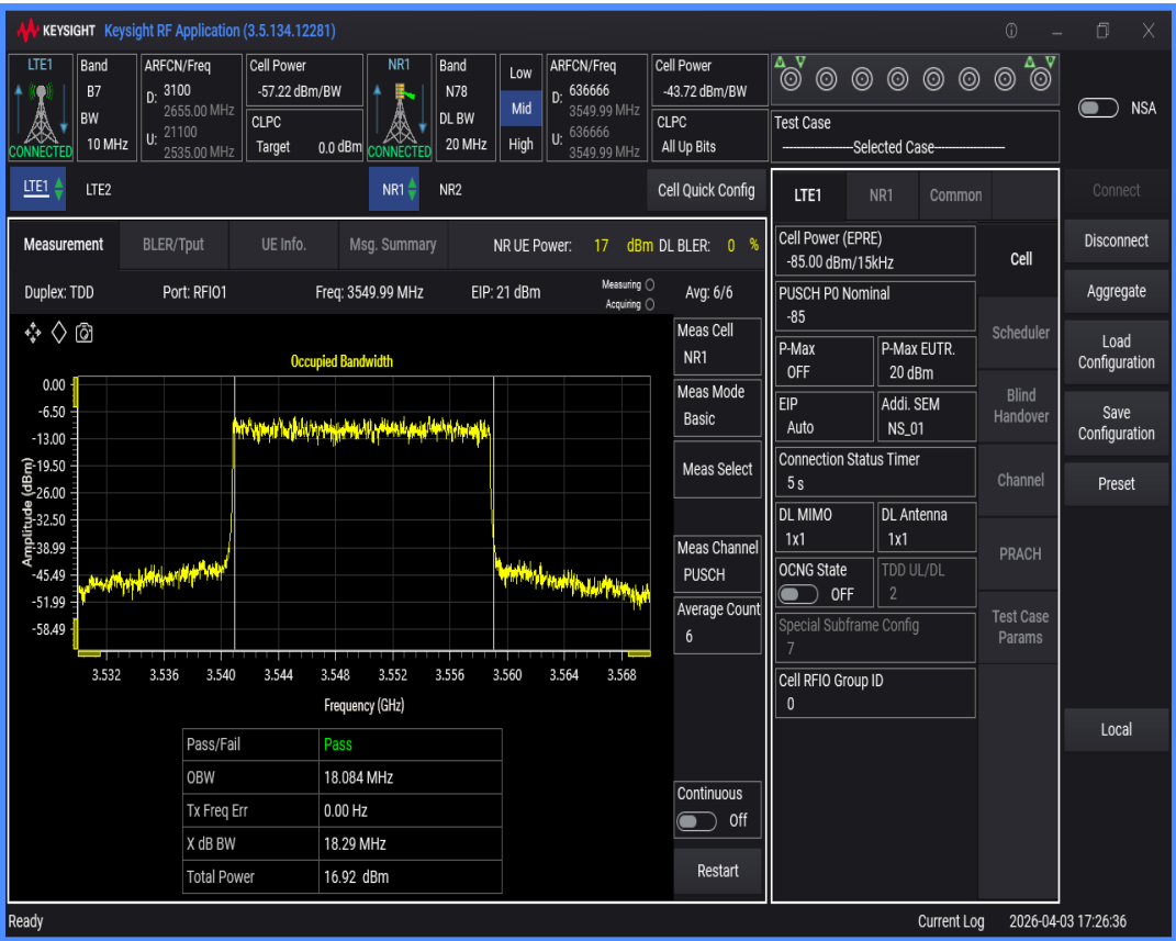
n78 SCS=30kHz DFT_QAM64 BW=10MHz Channel=636666 RB=24@0
