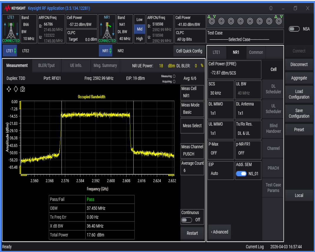
n41 SCS=30kHz DFT_QAM256 BW=90MHz Channel=518598 RB=240@0
