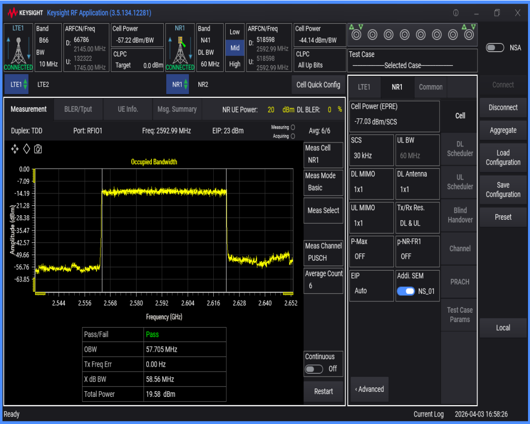
n41 SCS=30kHz DFT_BPSK BW=80MHz Channel=518598 RB=216@0
