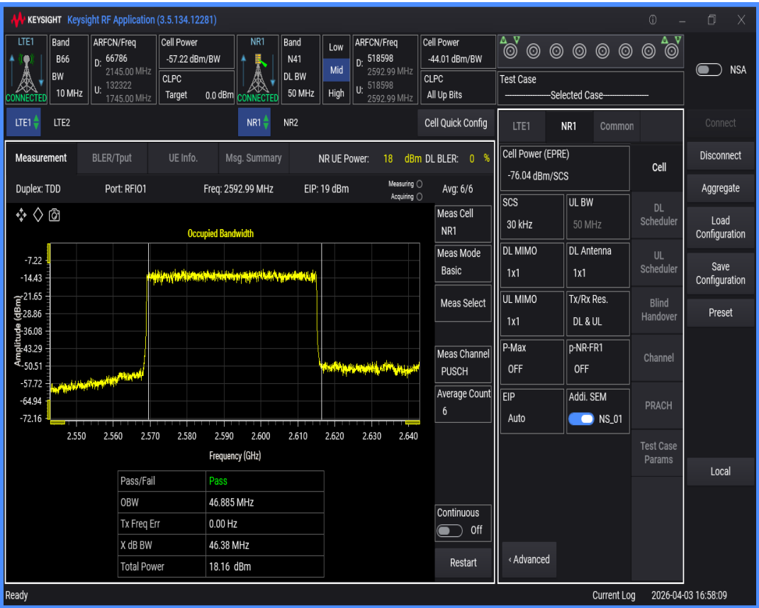
n41 SCS=30kHz DFT_QAM16 BW=60MHz Channel=518598 RB=162@0
