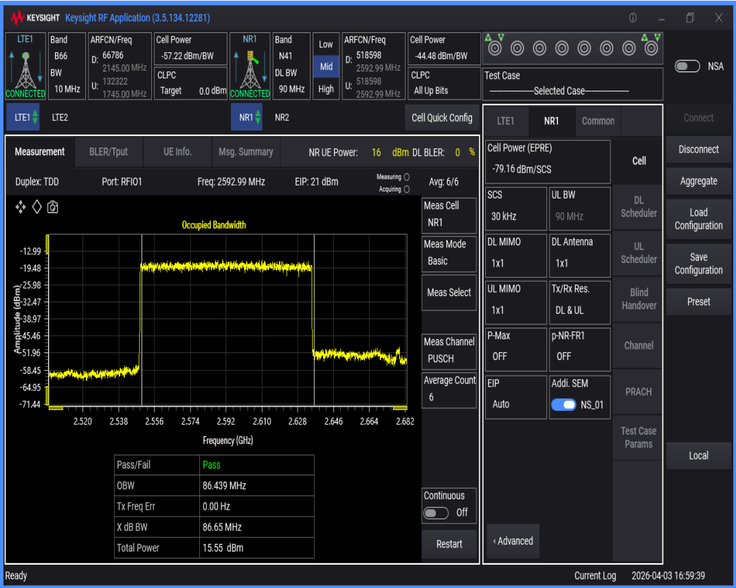
n41 SCS=30kHz DFT_QAM64 BW=100MHz Channel=518598 RB=270@0
