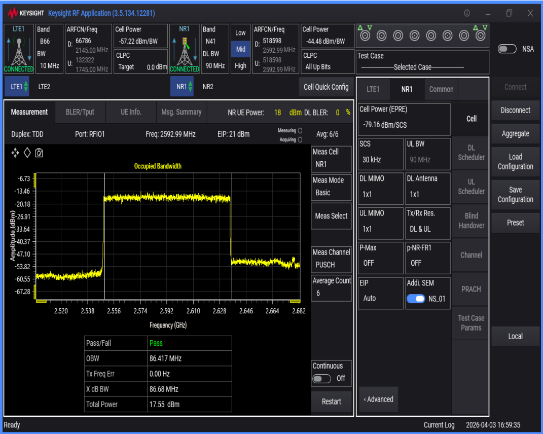
n41 SCS=30kHz DFT_QPSK BW=100MHz Channel=518598 RB=270@0
