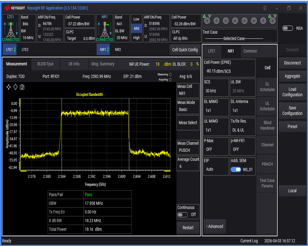
n41 SCS=30kHz DFT_QAM16 BW=40MHz Channel=518598 RB=100@0
