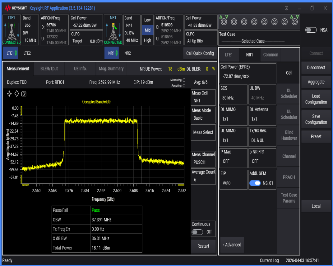
n41 SCS=30kHz DFT_BPSK BW=60MHz Channel=518598 RB=162@0
