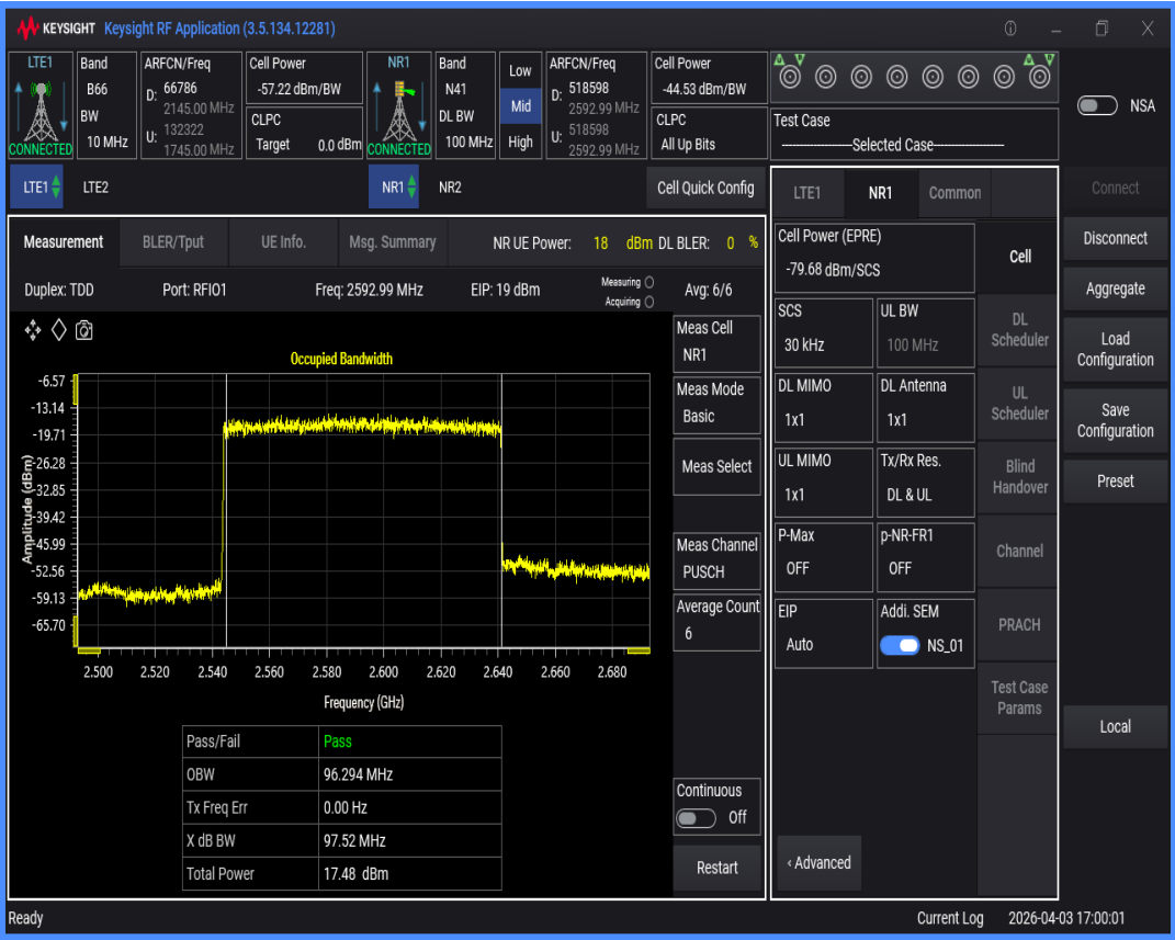
n41 SCS=30kHz DFT_QAM64 BW=90MHz Channel=518598 RB=240@0
