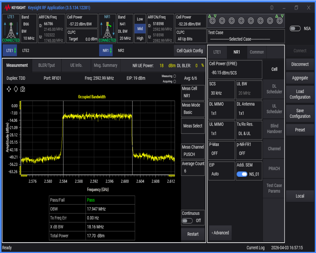
n41 SCS=30kHz DFT_QAM64 BW=40MHz Channel=518598 RB=100@0
