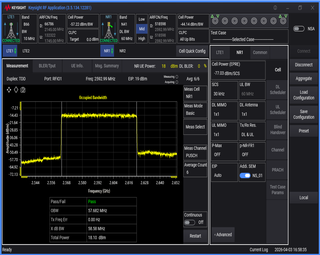
n41 SCS=30kHz DFT_QAM256 BW=60MHz Channel=518598 RB=162@0
