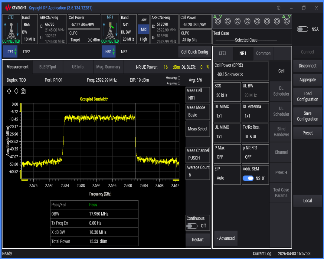
n41 SCS=30kHz DFT_QAM256 BW=40MHz Channel=518598 RB=100@0
