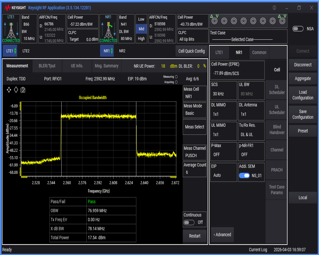
n41 SCS=30kHz DFT_QAM64 BW=50MHz Channel=518598 RB=128@0
