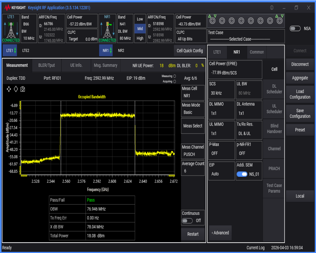
n41 SCS=30kHz DFT_QAM16 BW=50MHz Channel=518598 RB=128@0
