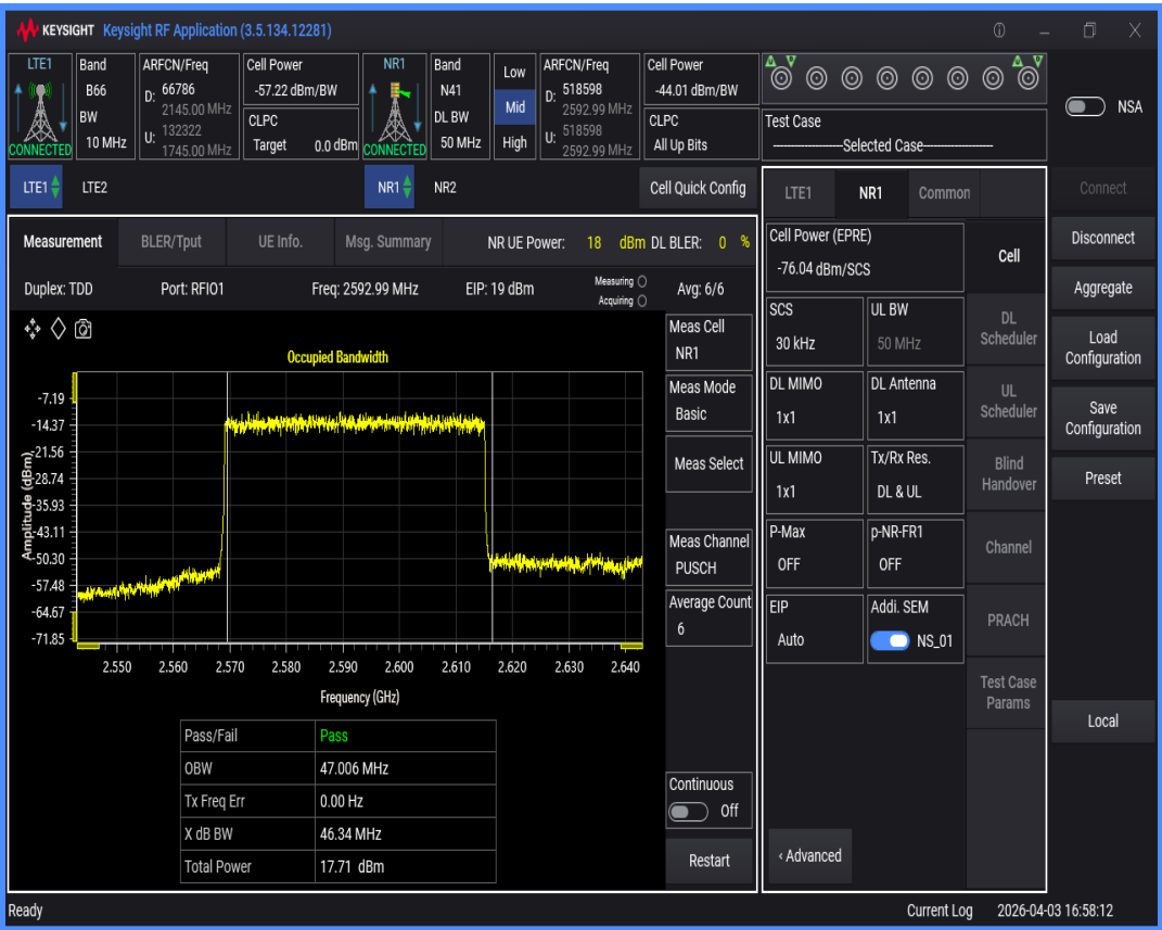
n41 SCS=30kHz DFT_QAM64 BW=60MHz Channel=518598 RB=162@0
