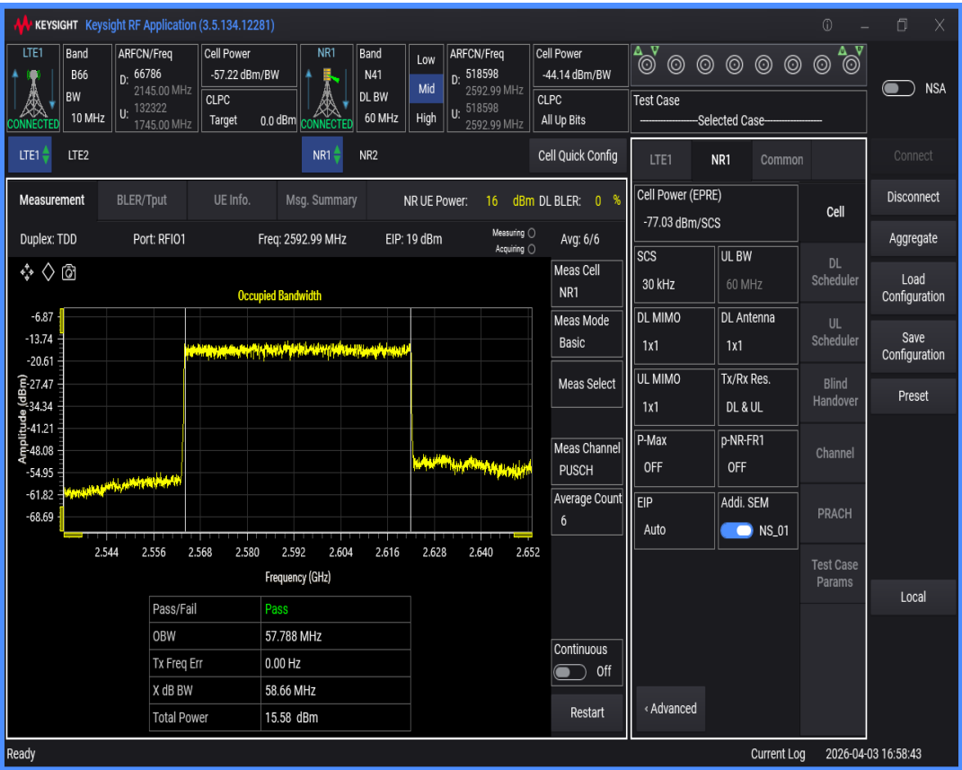
n41 SCS=30kHz DFT_QAM256 BW=80MHz Channel=518598 RB=216@0
