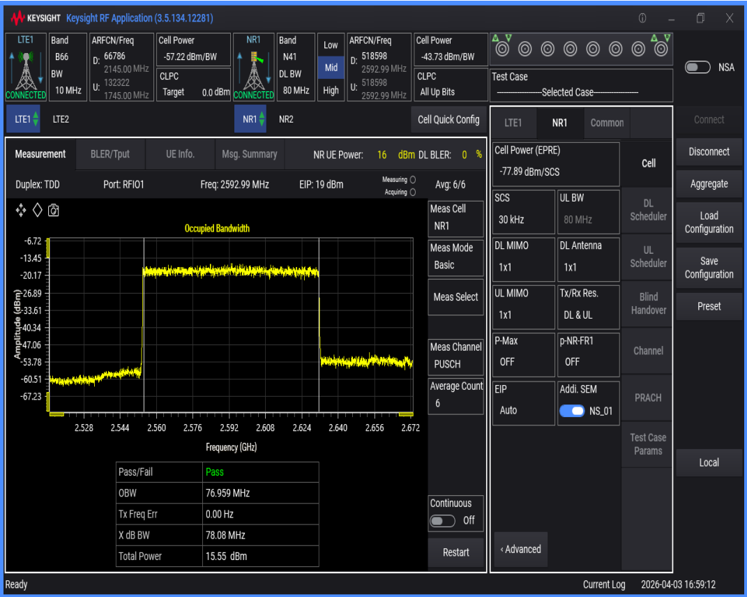
n41 SCS=30kHz DFT_QAM256 BW=50MHz Channel=518598 RB=128@0
