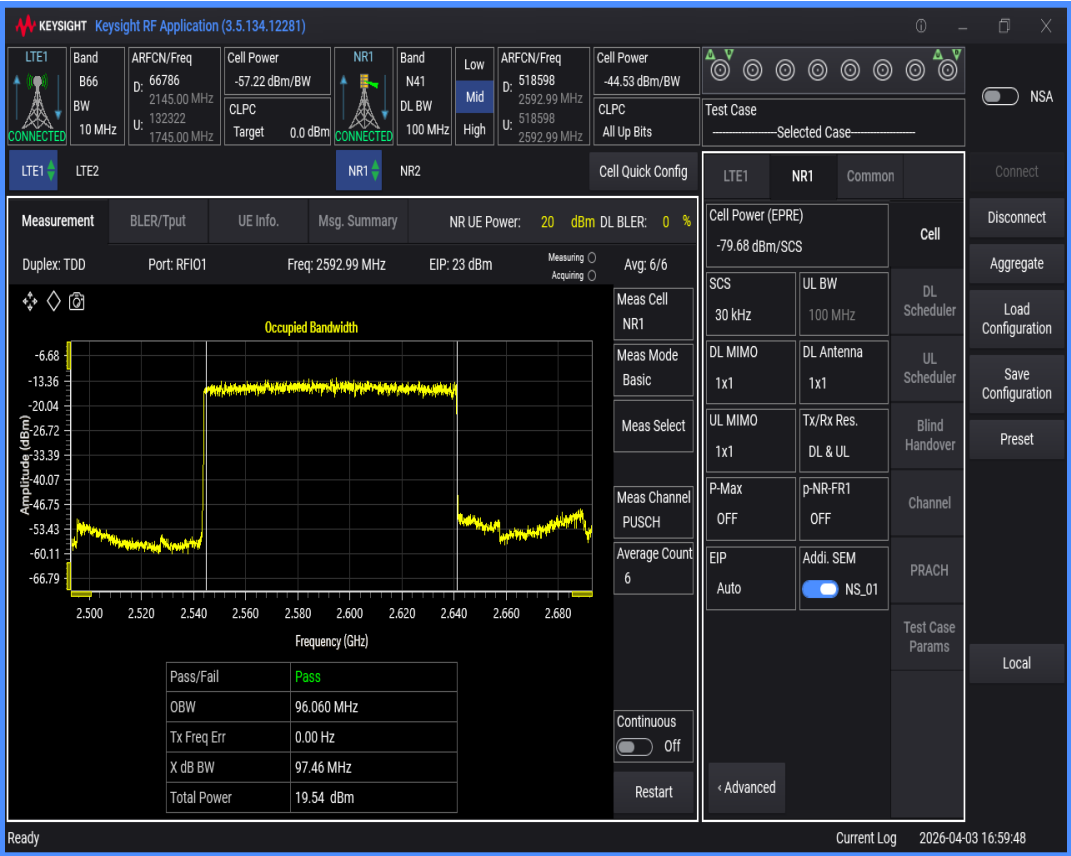
n41 SCS=30kHz DFT_BPSK BW=50MHz Channel=518598 RB=128@0
