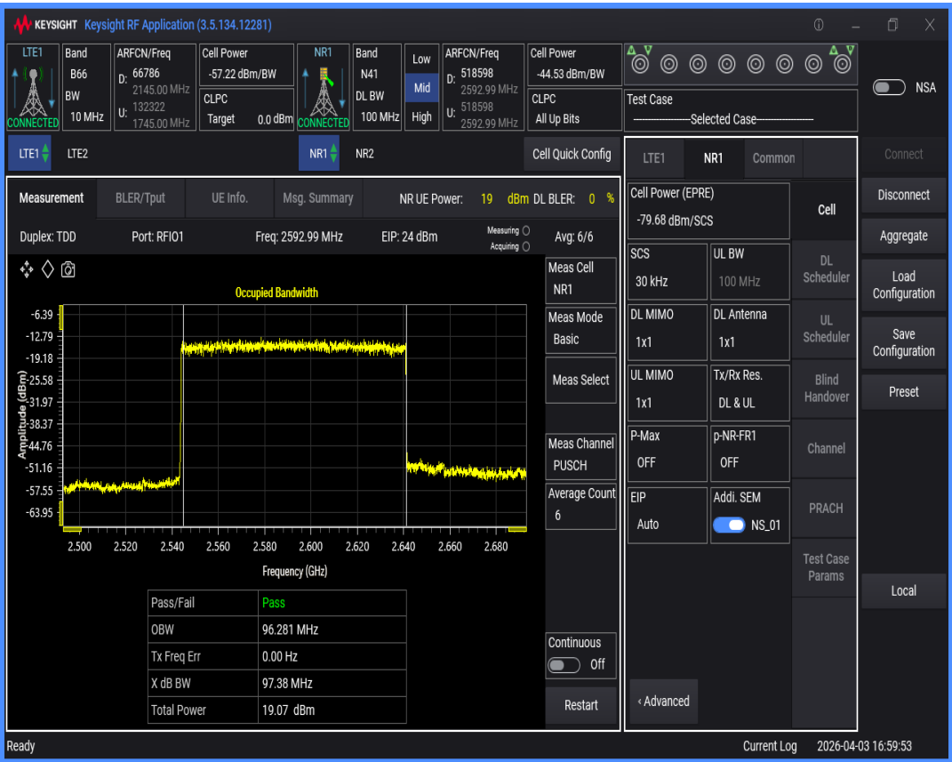
n41 SCS=30kHz DFT_QAM64 BW=80MHz Channel=518598 RB=216@0
