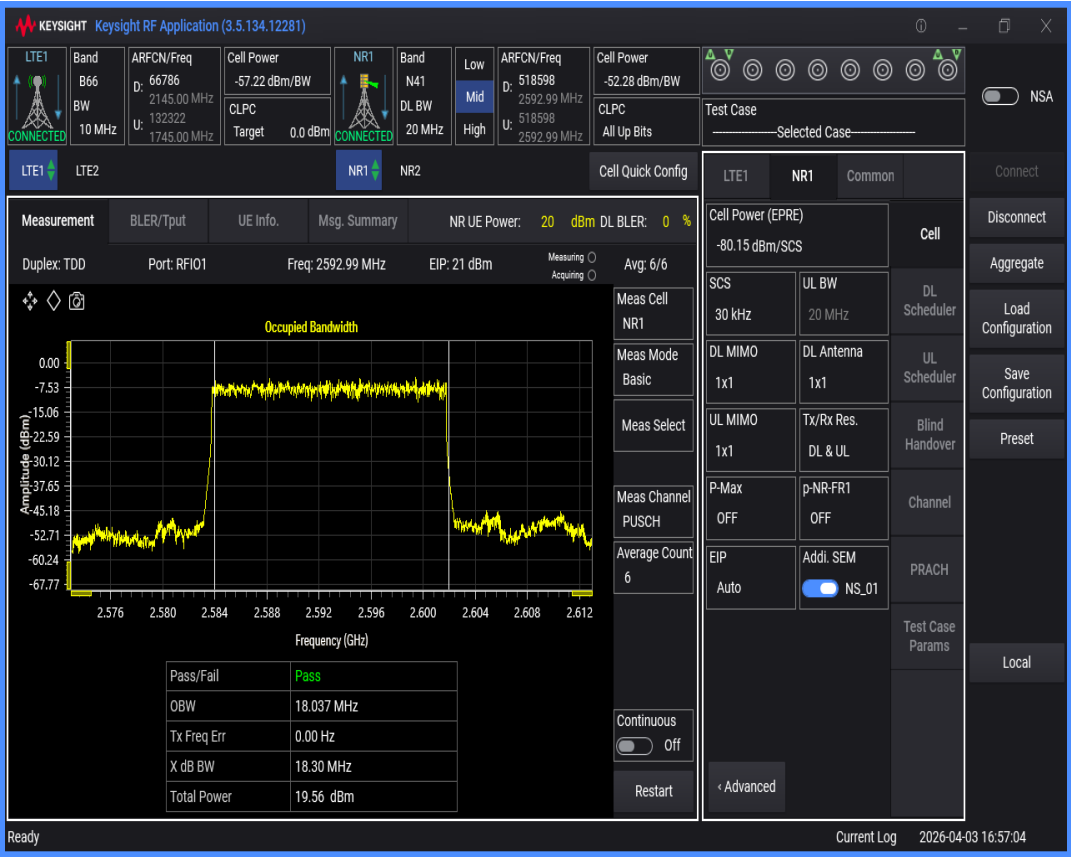
n41 SCS=30kHz DFT_QAM16 BW=100MHz Channel=518598 RB=270@0
