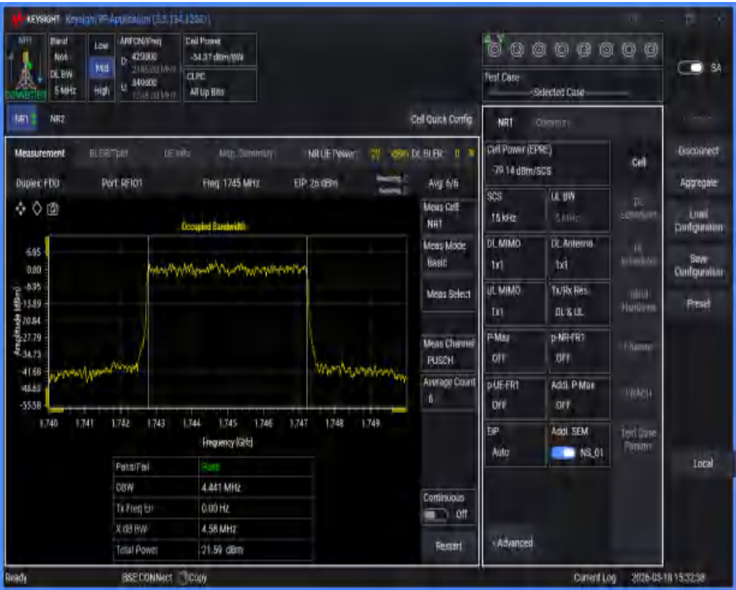
n66 SCS=15kHz DFT_QAM16 BW=40MHz Channel=349000 RB=216@0
