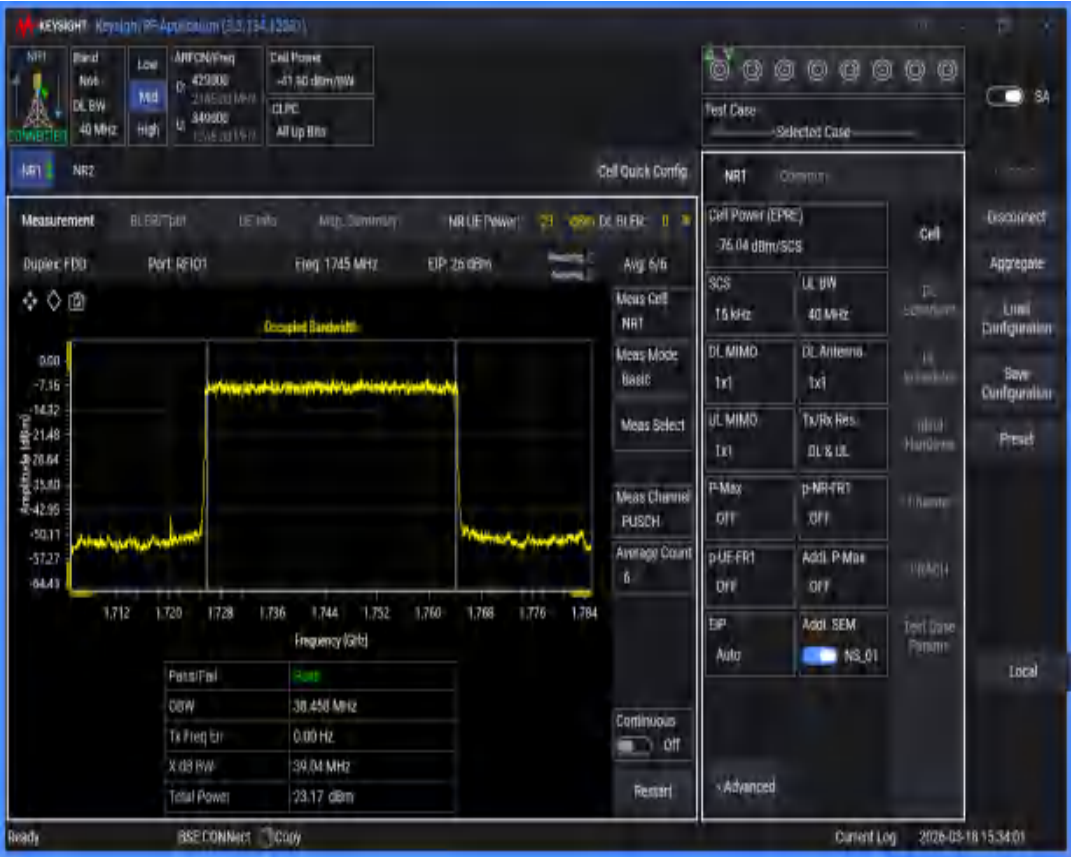
n66 SCS=15kHz DFT_QAM16 BW=20MHz Channel=349000 RB=100@0
