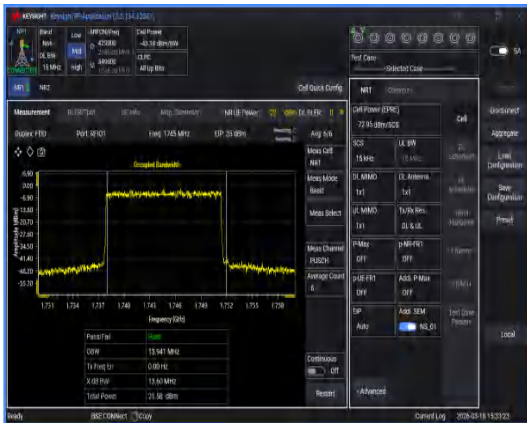
n66 SCS=15kHz DFT_QAM16 BW=5MHz Channel=349000 RB=25@0
