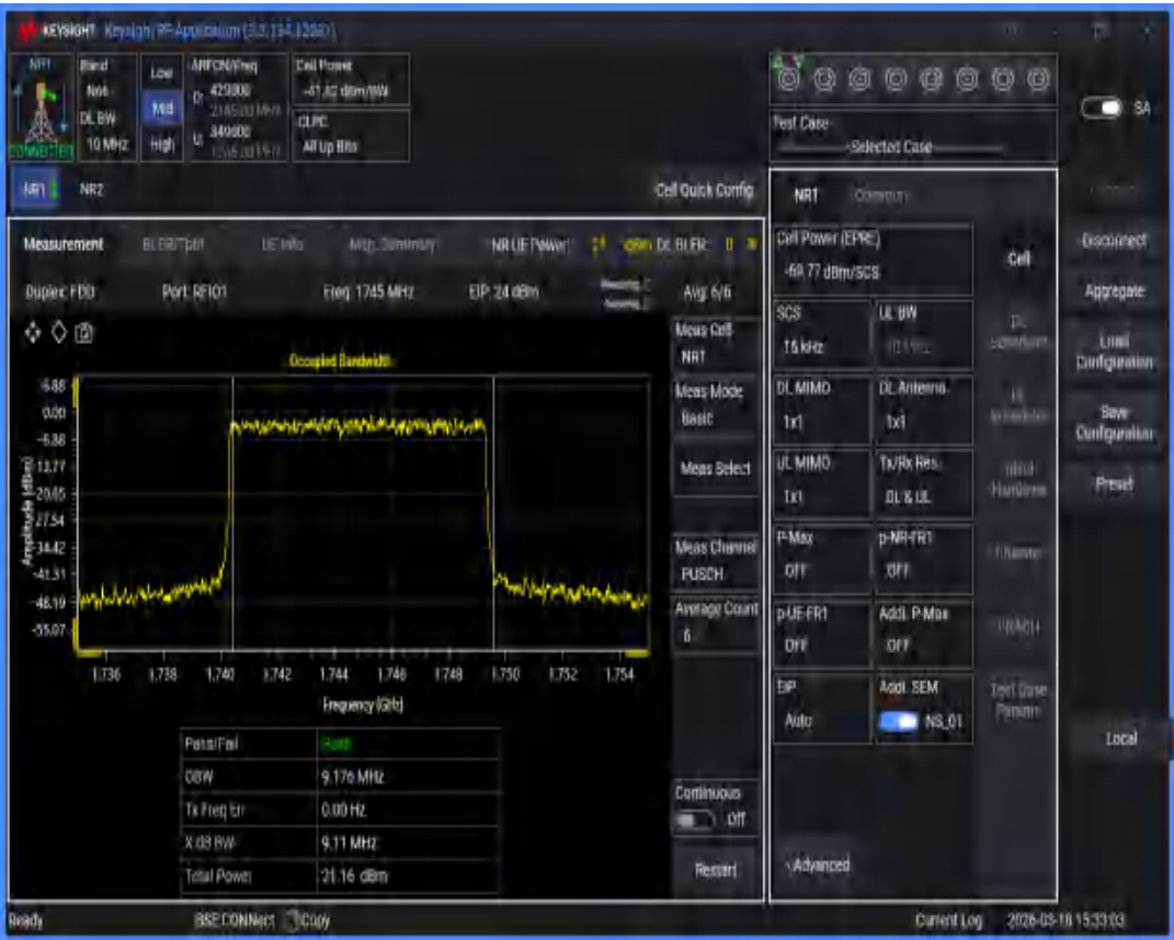
n66 SCS=15kHz DFT_QAM64 BW=5MHz Channel=349000 RB=25@0
