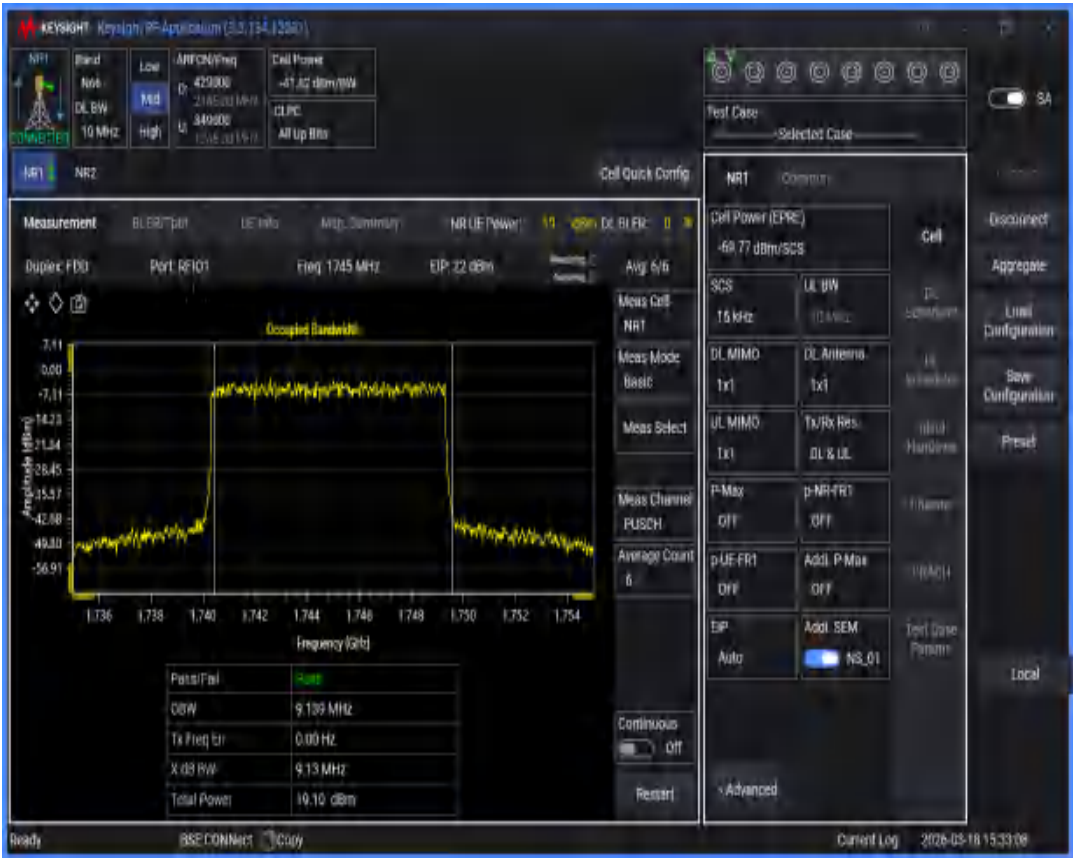
n66 SCS=15kHz DFT_QAM256 BW=15MHz Channel=349000 RB=75@0
