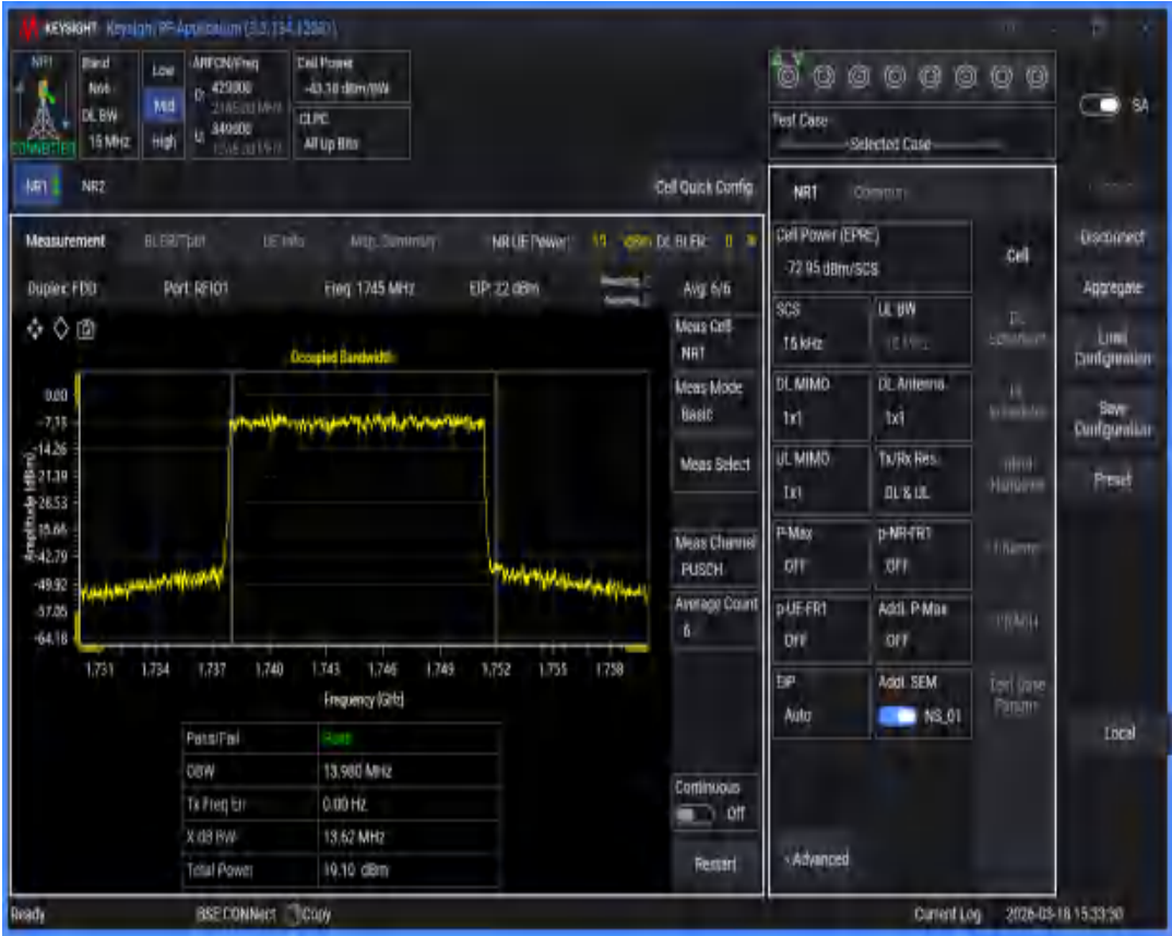
n66 SCS=15kHz DFT_QAM256 BW=40MHz Channel=349000 RB=216@0
