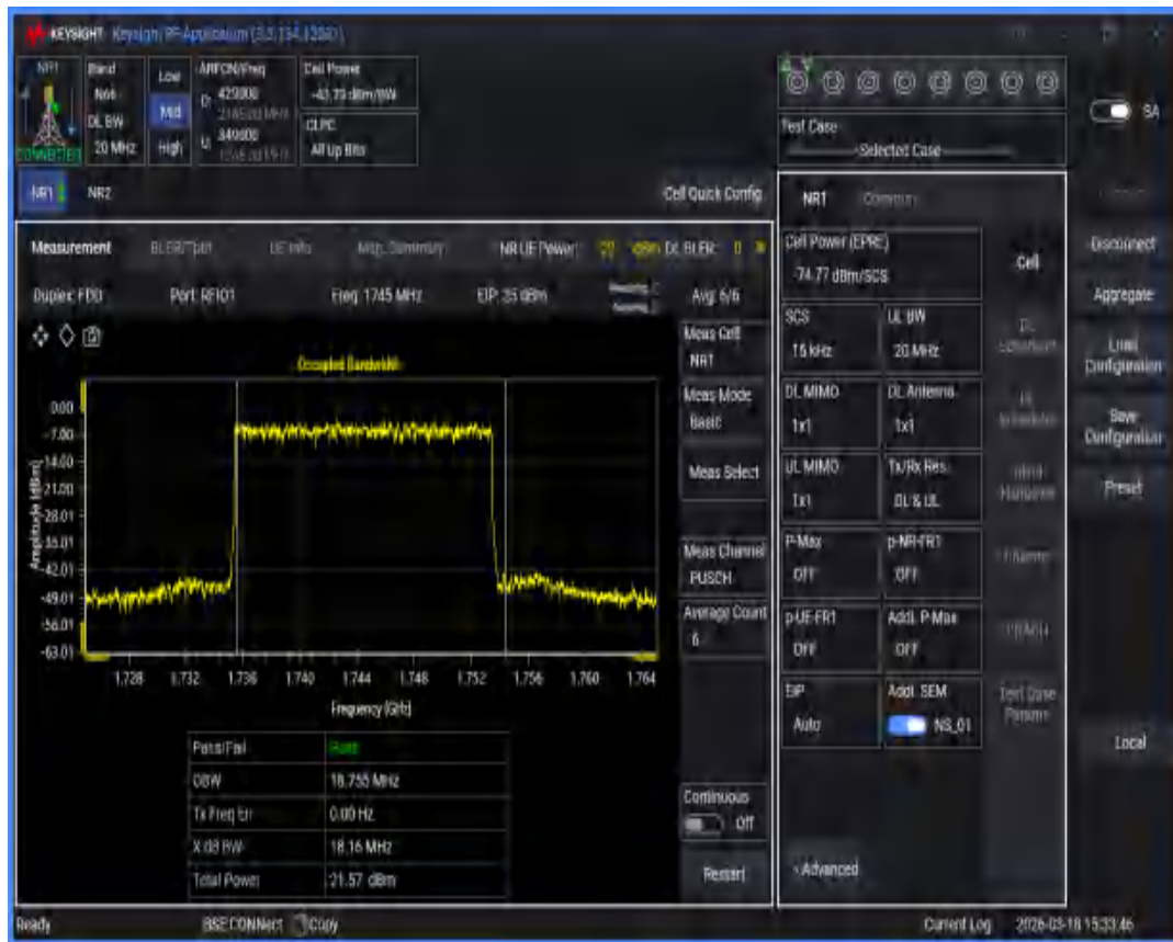
n66 SCS=15kHz DFT_QAM16 BW=15MHz Channel=349000 RB=75@0
