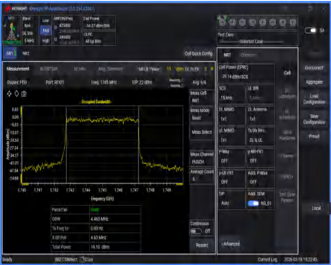
n66 SCS=15kHz DFT_QAM64 BW=15MHz Channel=349000 RB=75@0
