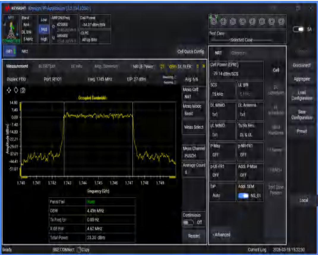
n66 SCS=15kHz DFT_BPSK BW=40MHz Channel=349000 RB=216@0
