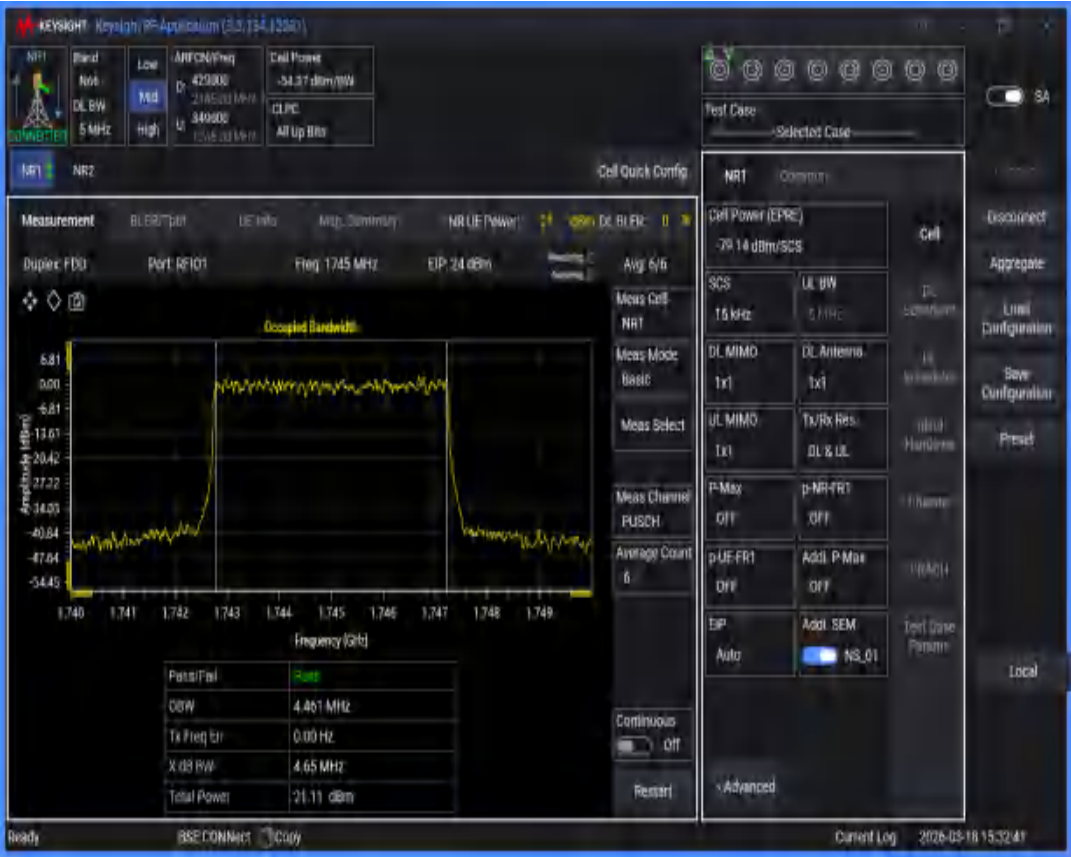
n66 SCS=15kHz DFT_QAM64 BW=40MHz Channel=349000 RB=216@0
