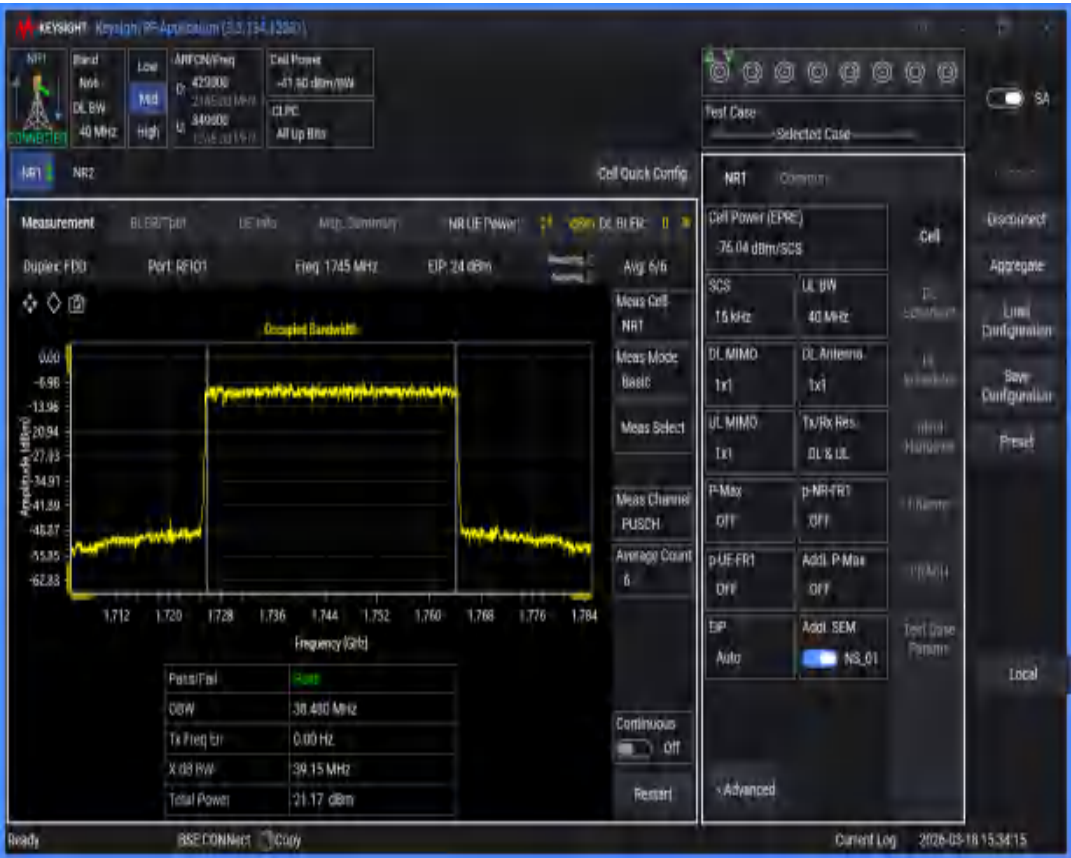
n66 SCS=15kHz DFT_QAM64 BW=20MHz Channel=349000 RB=100@0
