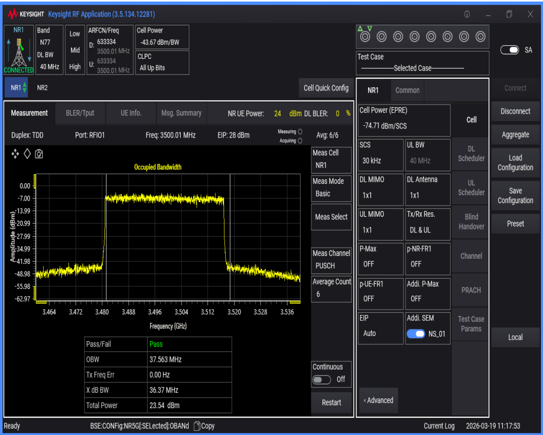
n77(3450-3550) SCS=30kHz DFT_QAM64 BW=30MHz Channel=633334 RB=75@0
