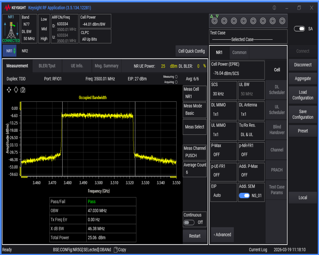
n77(3450-3550) SCS=30kHz DFT_QPSK BW=90MHz Channel=633334 RB=240@0
