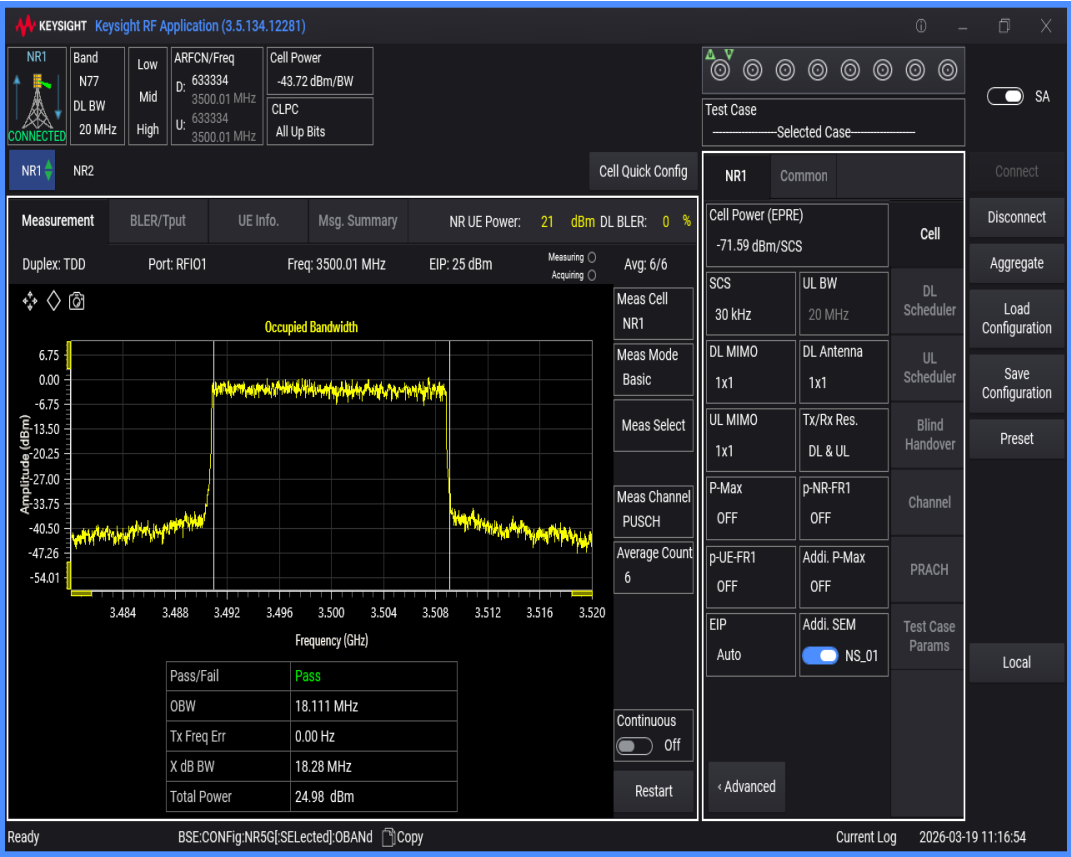
n77(3450-3550) SCS=30kHz DFT_QPSK BW=15MHz Channel=633334 RB=36@0
