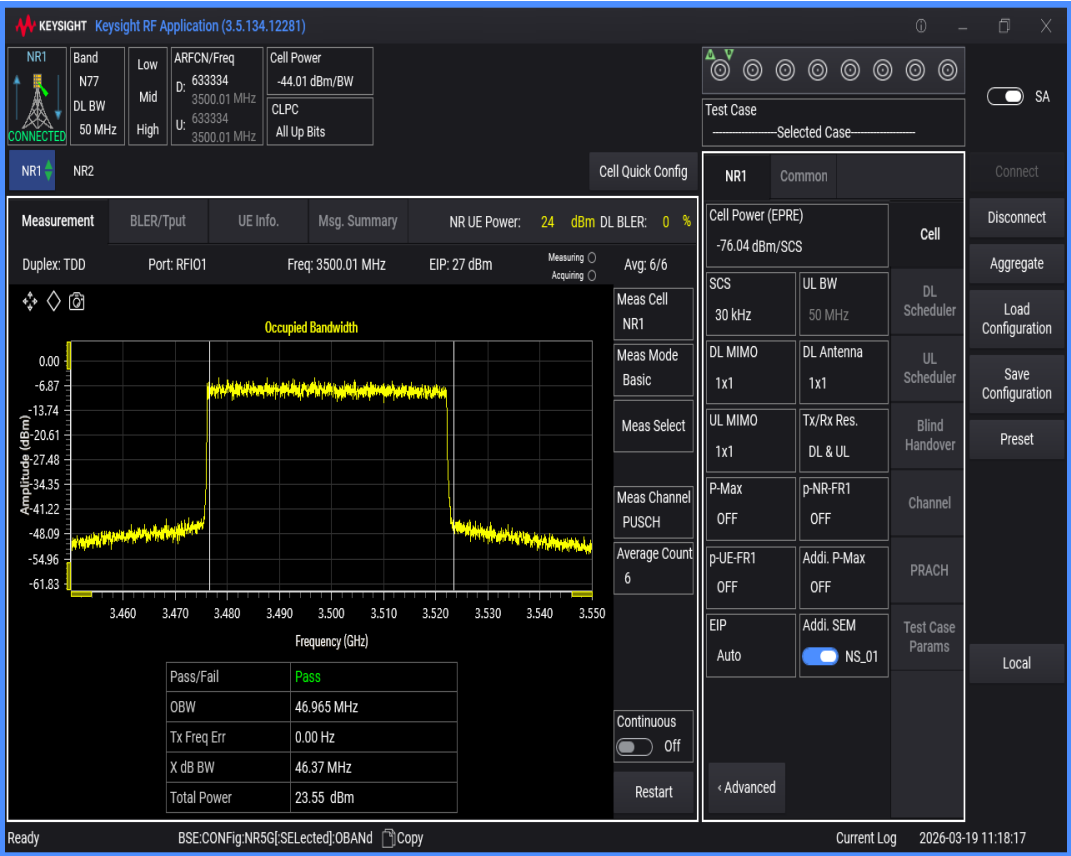
n77(3450-3550) SCS=30kHz DFT_QAM64 BW=80MHz Channel=633334 RB=216@0
