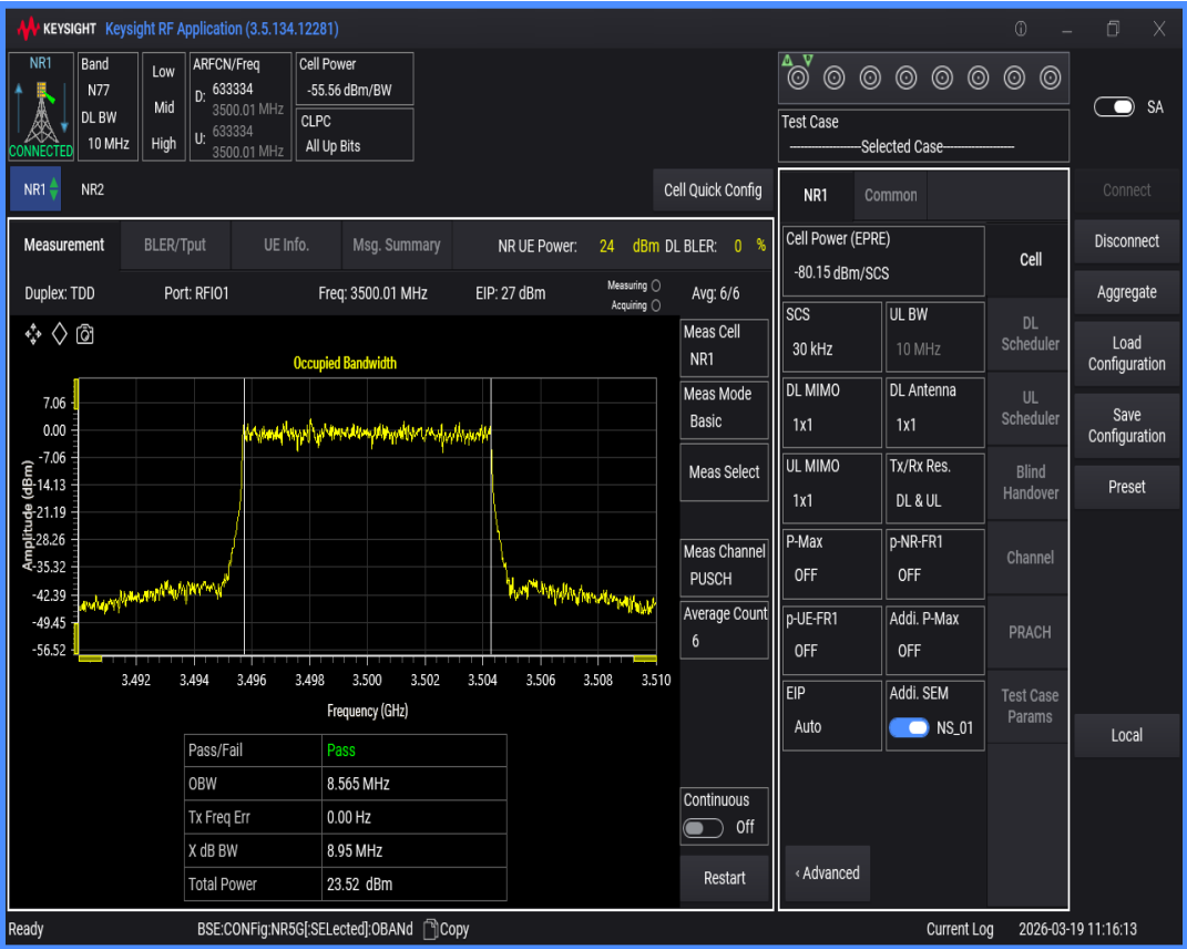
n77(3450-3550) SCS=30kHz DFT_QAM64 BW=40MHz Channel=633334 RB=100@0
