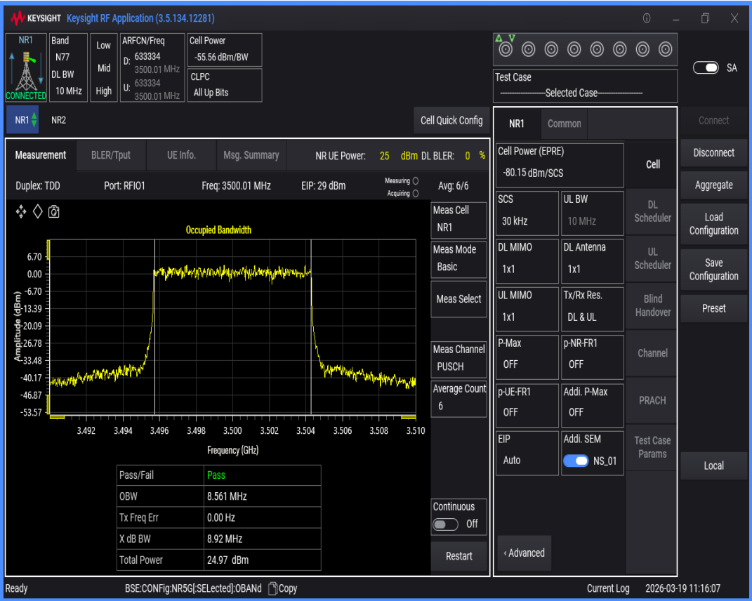
n77(3450-3550) SCS=30kHz DFT_QPSK BW=100MHz Channel=633334 RB=270@0
