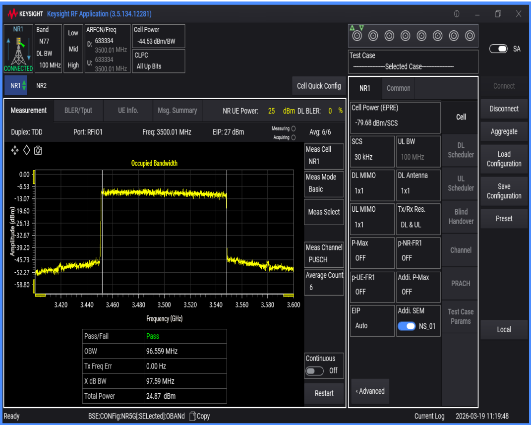
n77(3450-3550) SCS=30kHz DFT_QAM64 BW=90MHz Channel=633334 RB=240@0
