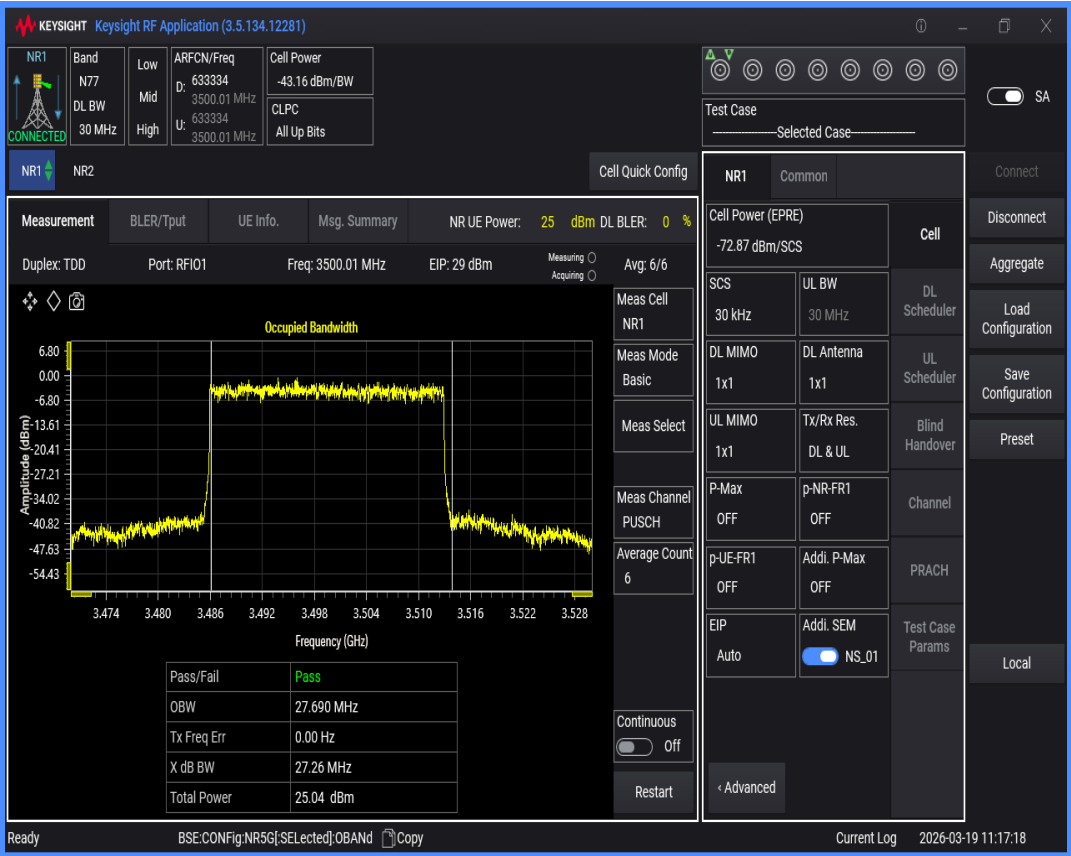
n77(3450-3550) SCS=30kHz DFT_QPSK BW=60MHz Channel=633334 RB=162@0
