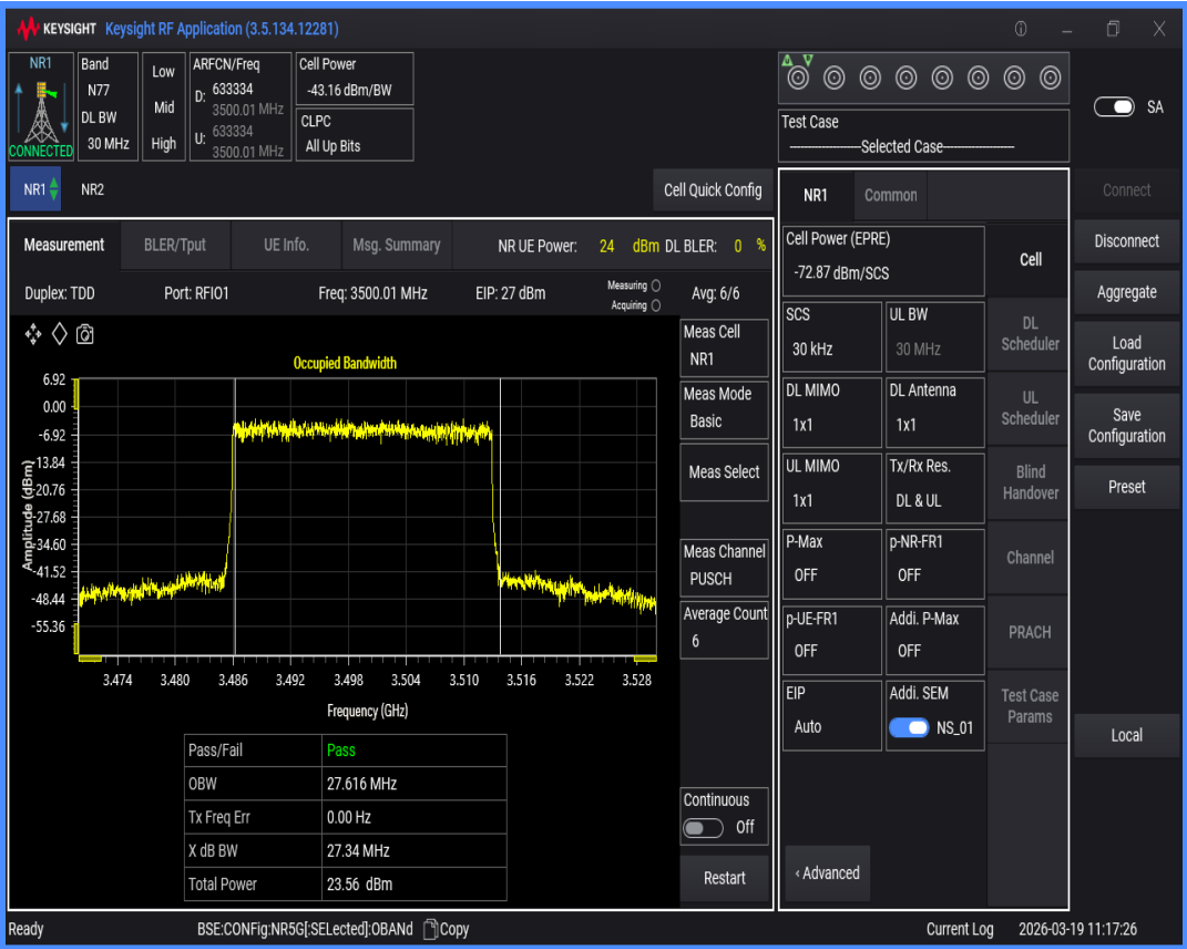
n77(3450-3550) SCS=30kHz DFT_QAM64 BW=60MHz Channel=633334 RB=162@0
