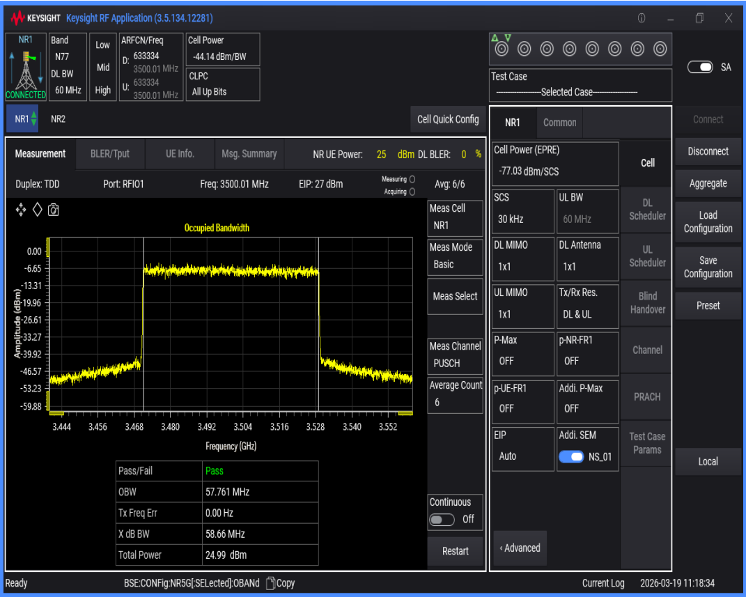
n77(3450-3550) SCS=30kHz DFT_QPSK BW=50MHz Channel=633334 RB=128@0
