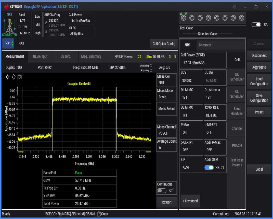
n77(3450-3550) SCS=30kHz DFT_QAM64 BW=50MHz Channel=633334 RB=128@0
