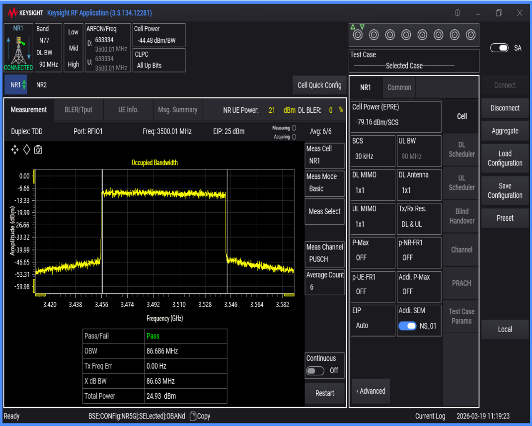
n77(3450-3550) SCS=30kHz DFT_QPSK BW=80MHz Channel=633334 RB=216@0
