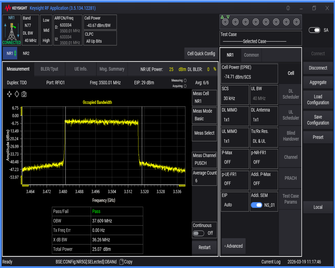
n77(3450-3550) SCS=30kHz DFT_QPSK BW=30MHz Channel=633334 RB=75@0
