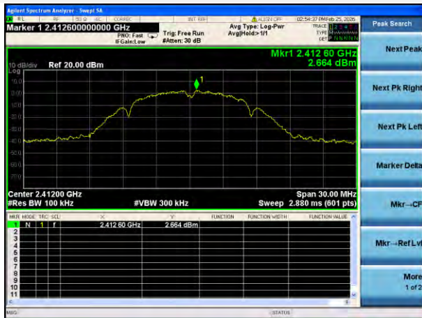
802.11b LOW CHANNEL, CARRIER LEVEL
