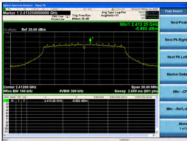
802.11g LOW CHANNEL, CARRIER LEVEL
