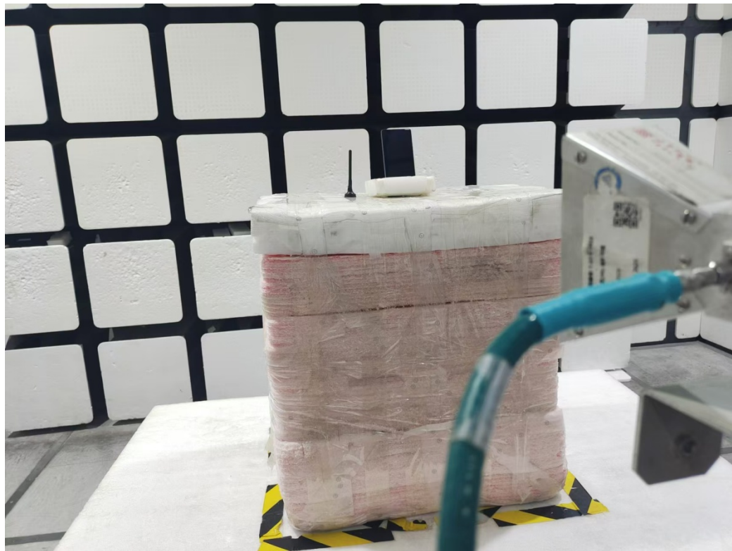
Radiated Emissions View (25-40 GHz)
