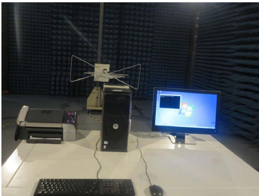
2 Photo of Radiation Emission Test
