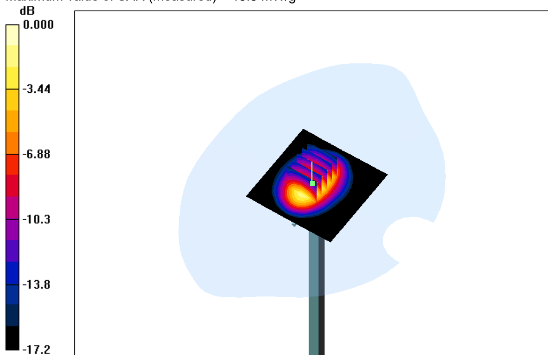
System Performance Check 1900MHz Body 1000mW
