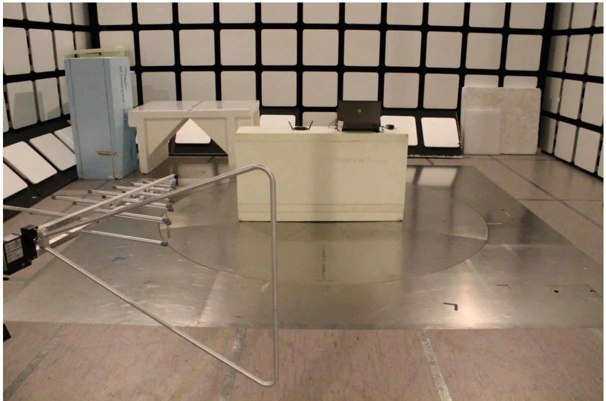
Picture 4. The EUT and the test set-up for radiated emission test 30MHz-1GHz.
