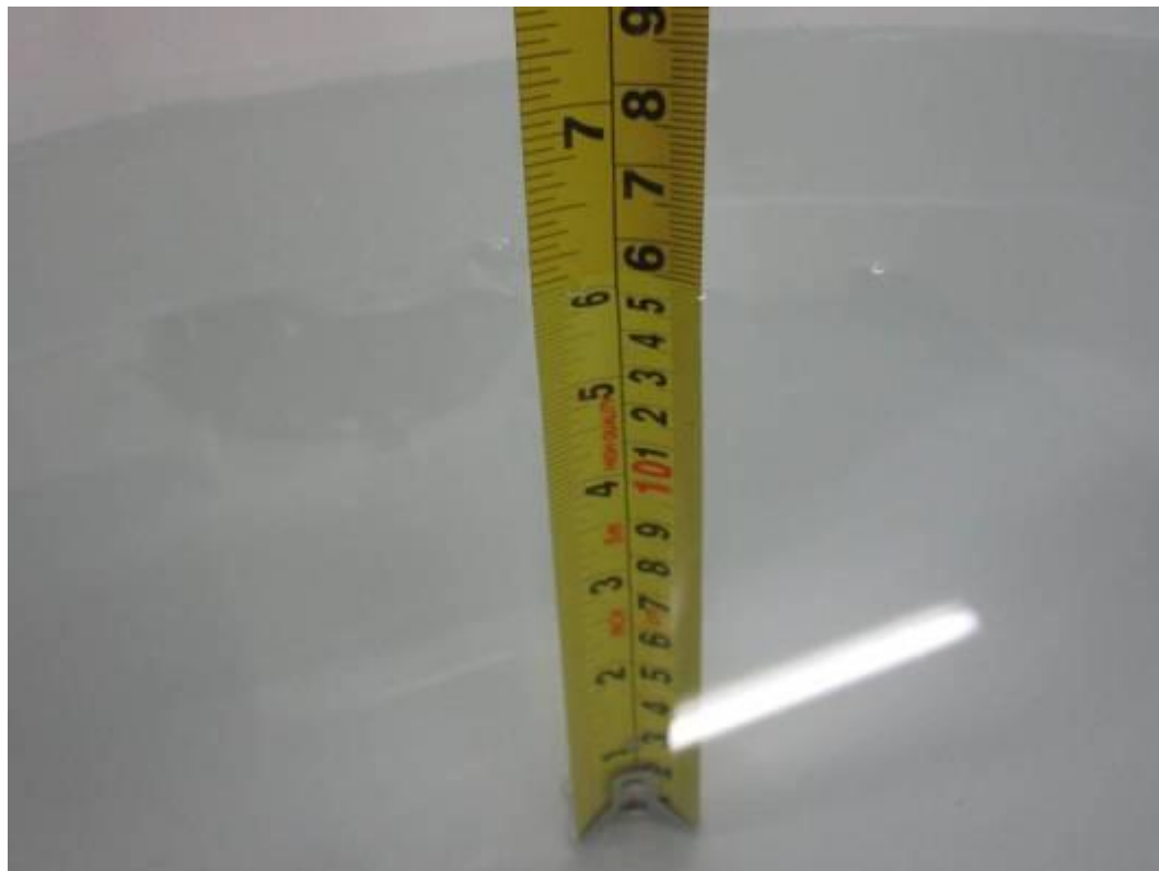
Liquid depth \geq 15\text{cm}
