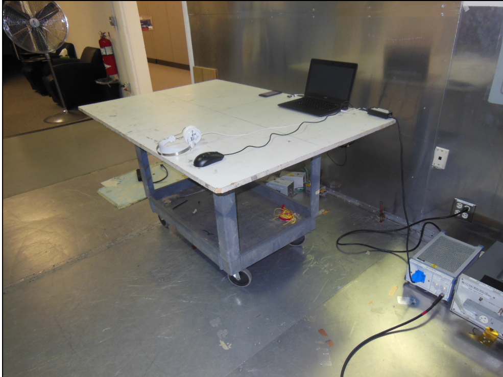
Figure 8: AC Power Line Conducted Emissions
