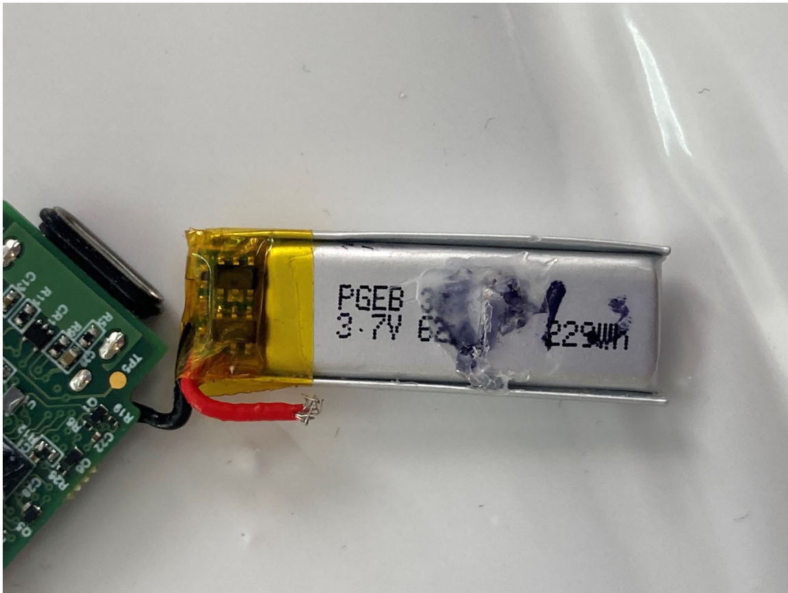
Figure 4. Battery pack markings
