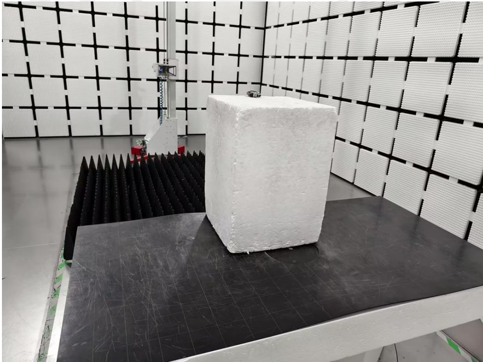
Spurious Radiation Emissions Test (>1G)
