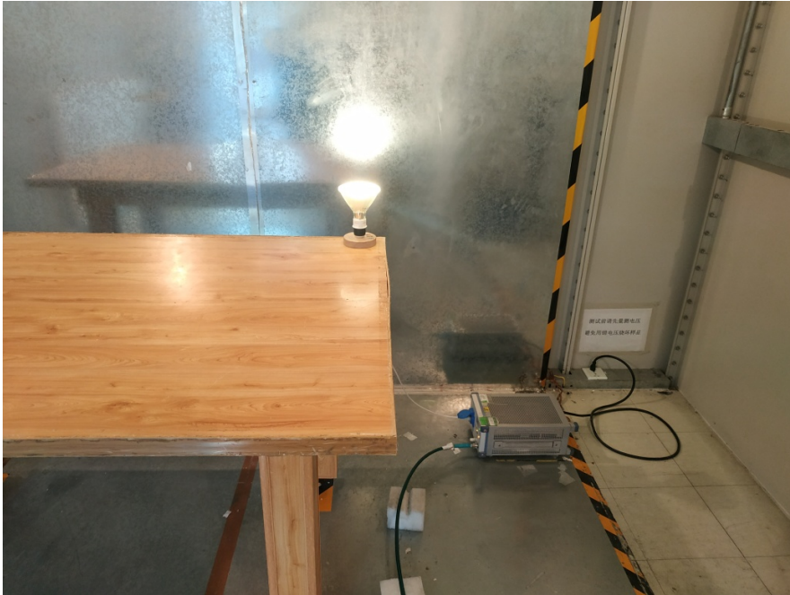
Conducted Emissions (Side View)
