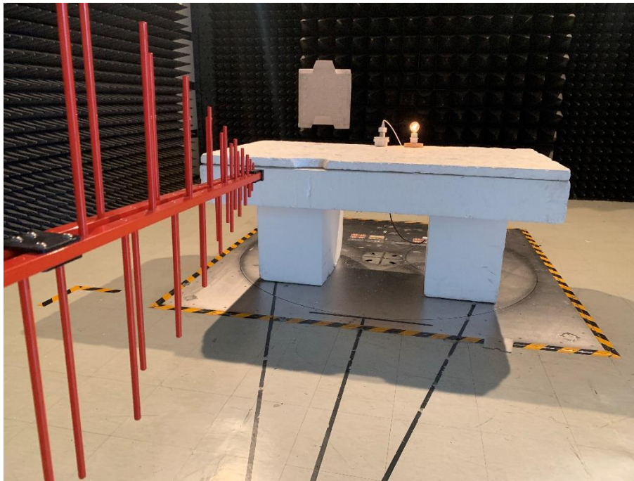
Radiated Emissions -Front View (Below 1GHz)
