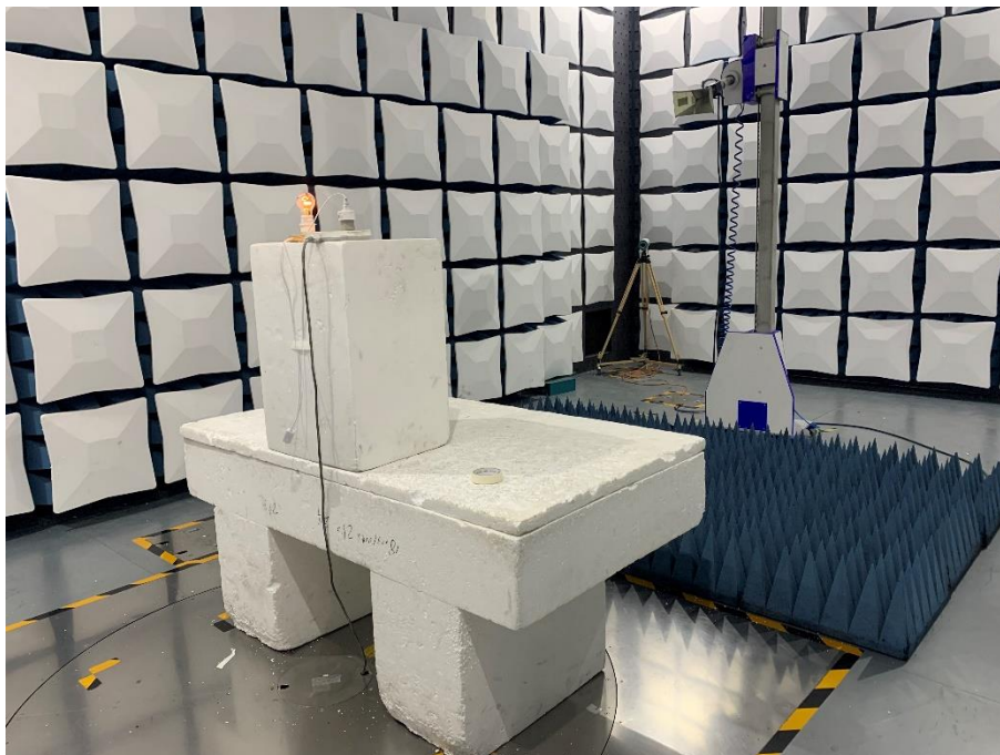
Radiated Emissions - Rear View (Above 1GHz)
