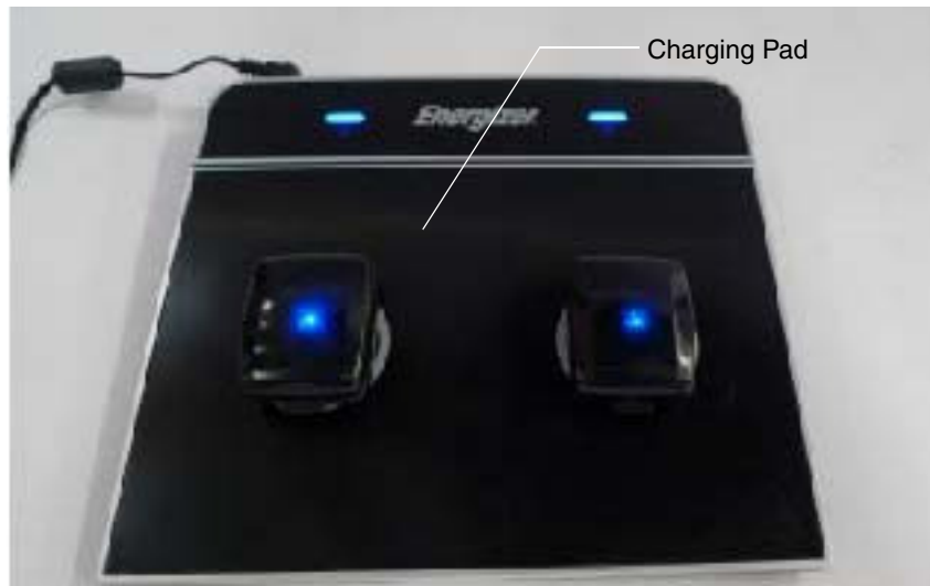
Figure 5. Charging Pad for IMU Battery
