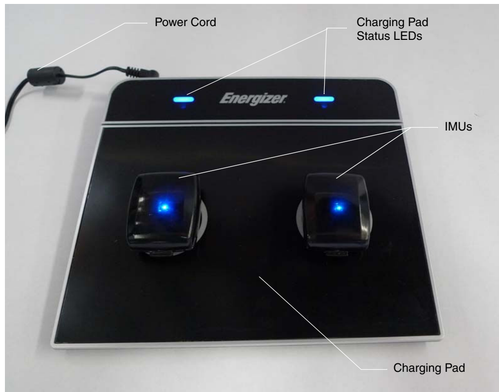
Figure 43. Charging the IMU Battery
