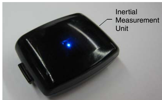
Figure 9. Example Inertial Measurement Unit
