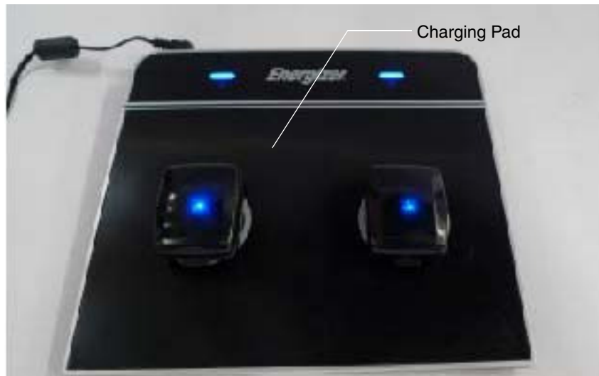
Figure 5. Charging Pad for IMU Battery
