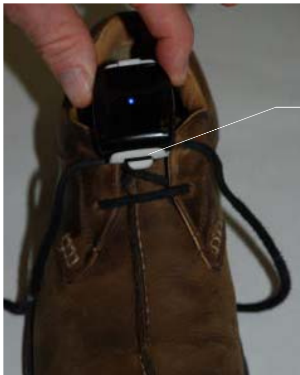
Figure 22. Attaching the Shoe Clip to the Shoe
