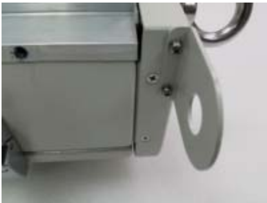
Figure 10. After mounting the GPS bracket to the xFemto unit
