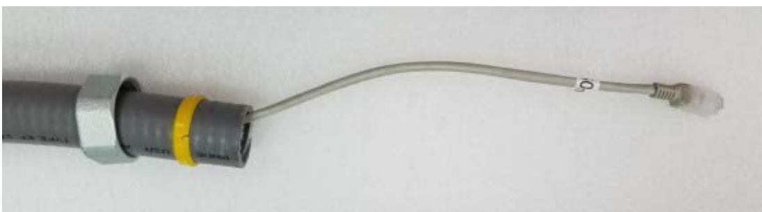
Figure 29. Sealing ring fitted to the conduit
