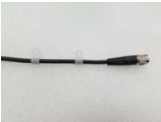
Figure 14. GPS clamps on the cable
