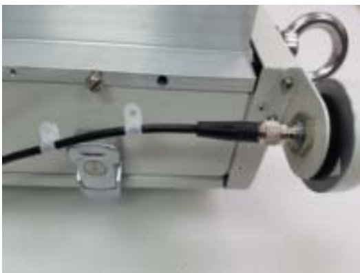
Figure 15. GPS cable connection to the GPS antenna
