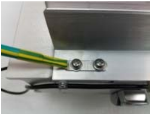
Figure 20. Ground Cable Attachment to the xFemto
