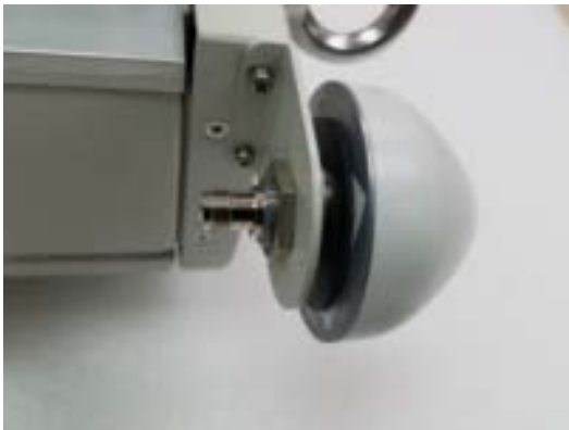
Figure 12. After mounting the GPS antenna to the GPS bracket
