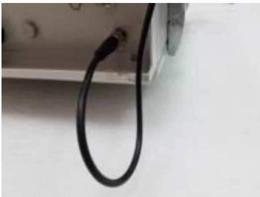
Figure 18. GPS cable connection to the xFemto unit
