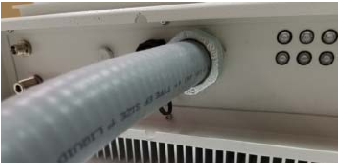
Figure 31. Connecting the conduit to the xFemto
