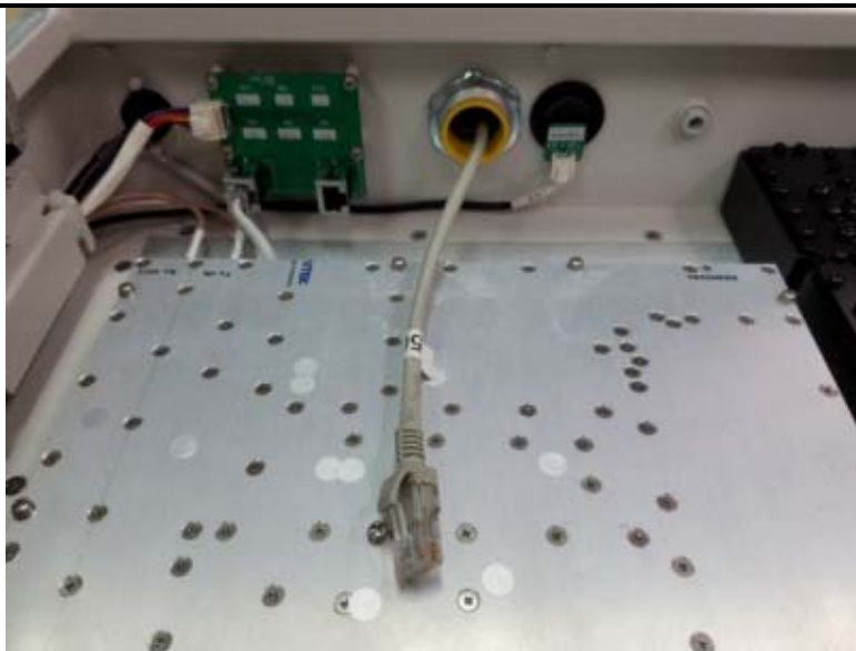
Figure 32. Before connecting the LAN cable to the xFemto
