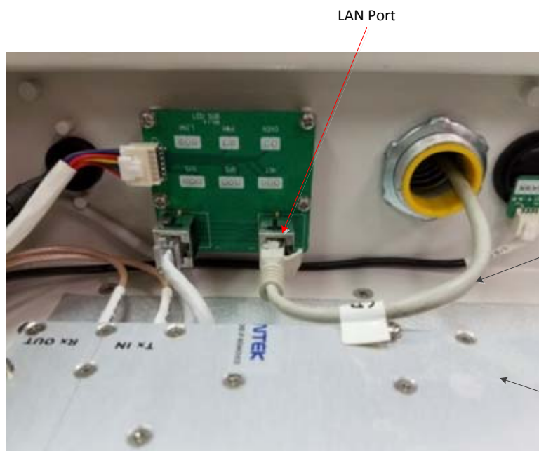
Figure 33 .After connecting the LAN cable to the xFemto
