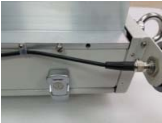
Figure 16. GPS cable attachment - First
