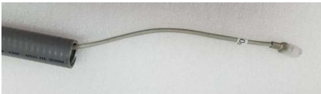
Figure 26. LAN cable in conduit
