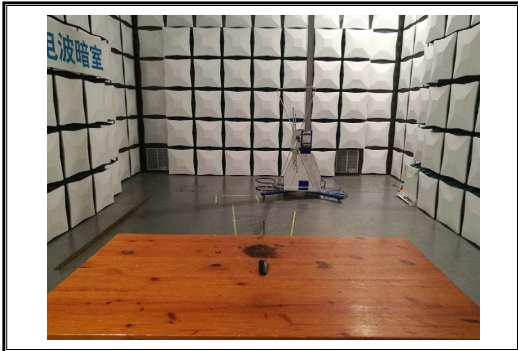
RADIATED RF MEASUREMENT SETUP (BELOW 1GHz)
