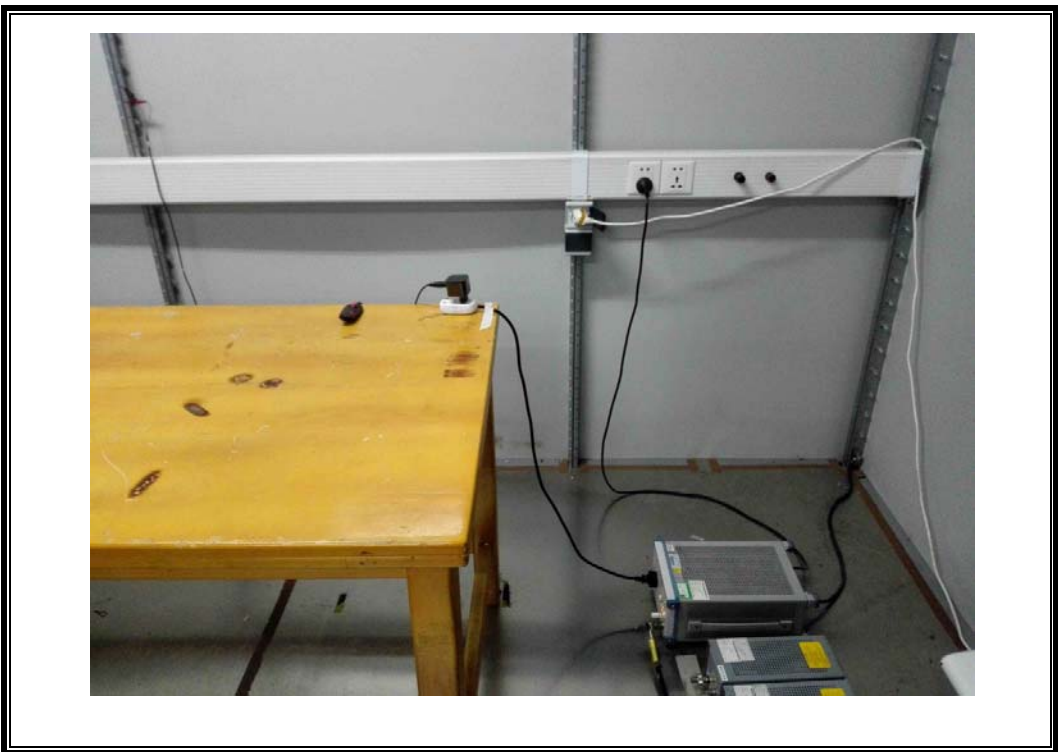
POWERLINE CONDUCTED EMISSIONS MEASUREMENT SETUP
