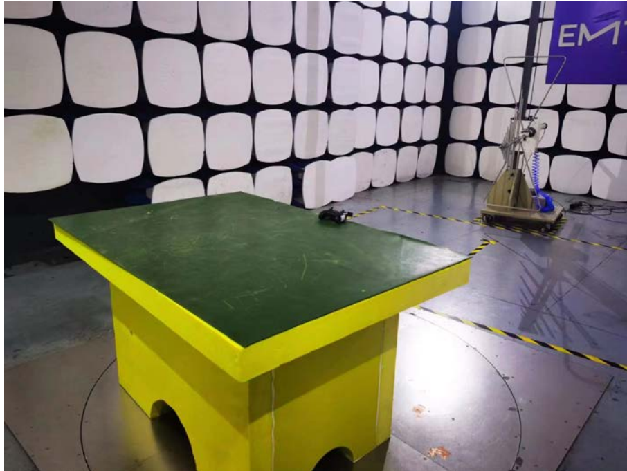
Spurious Emission Test Setup (Above 1GHz)
