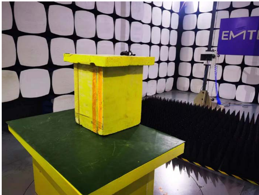
Spurious Emission Test Setup (Above 1GHz)
