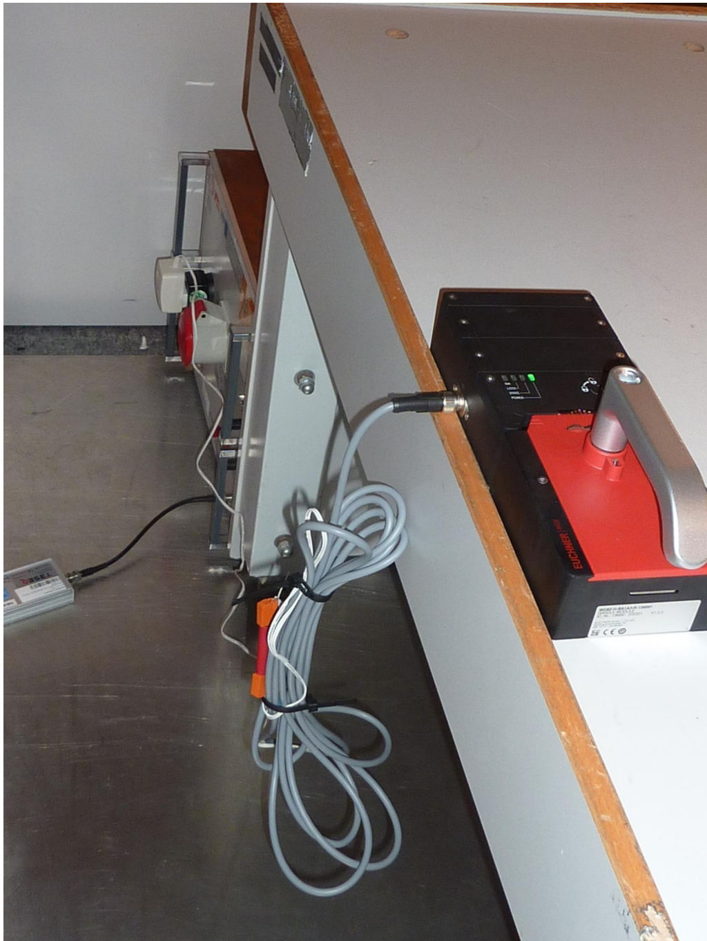
180889_g.jpg: MGB2-L2-MLI-U-Y0000-BJ-156392, test set-up shielded chamber
