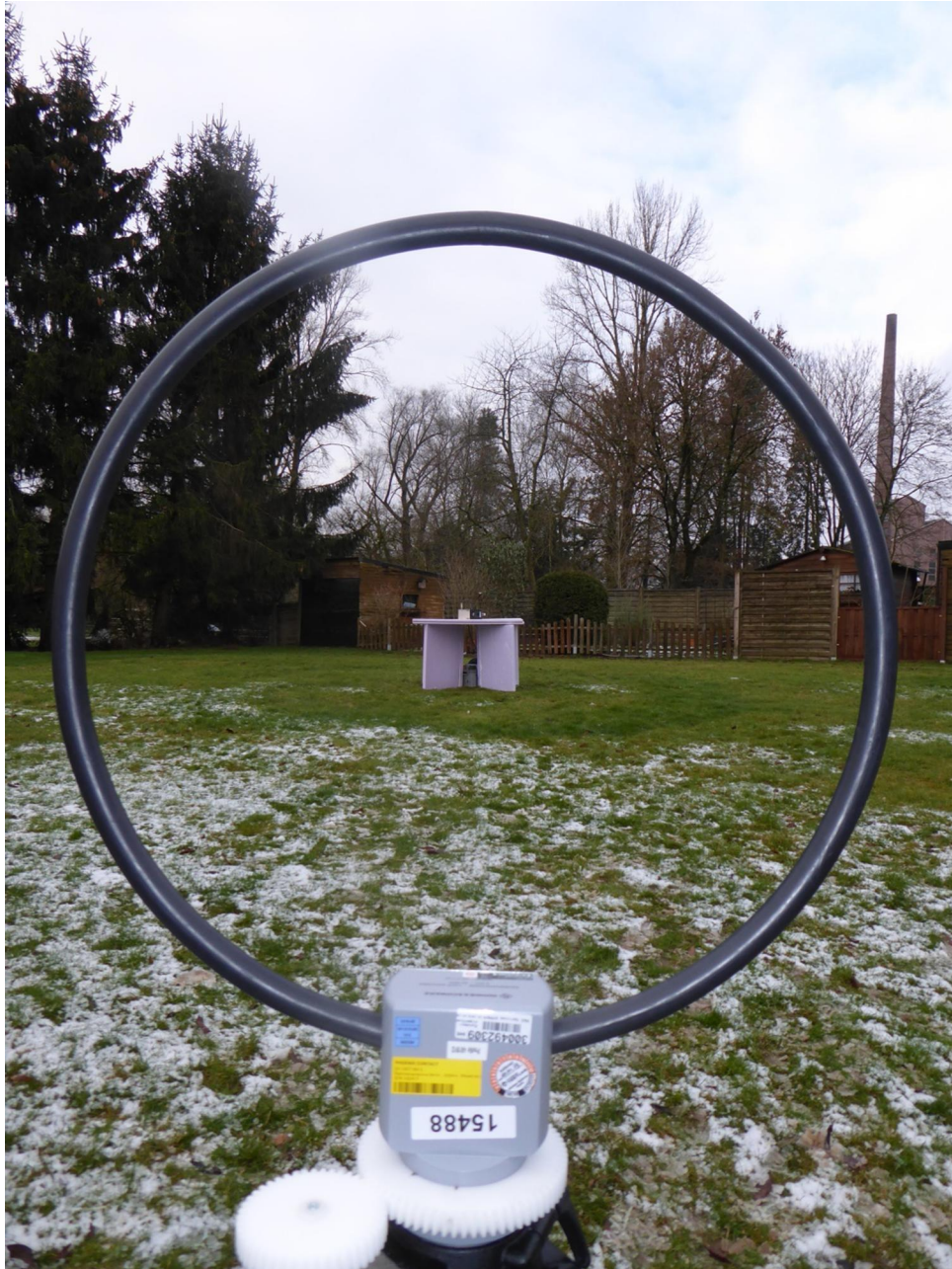
182138_Set10.JPG: Test setup open area test site, 9 kHz – 30 MHz @ 10m
