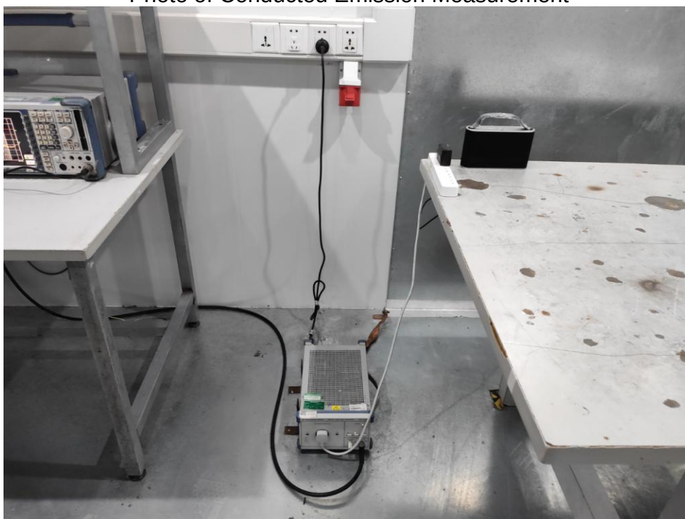
FCC ID: 2AJ5Q-OS447 Photo of Conducted Emission Measurement
