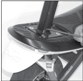
4. Remove four Allen head bolts and lock nuts (tools not included). To perform this operation you will need a six millimeter Allen wrench and a 17 millimeter open end wrench.
