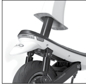
3. Slide up and remove plastic seat tower cover.
