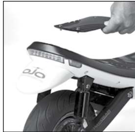
6. Install seat cover plate (included in carton) using the four Allen screws removed in step number two above.
