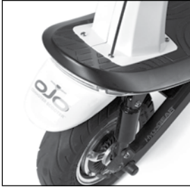
2. Remove four Allen screws that are located at the base of the seat tower.
