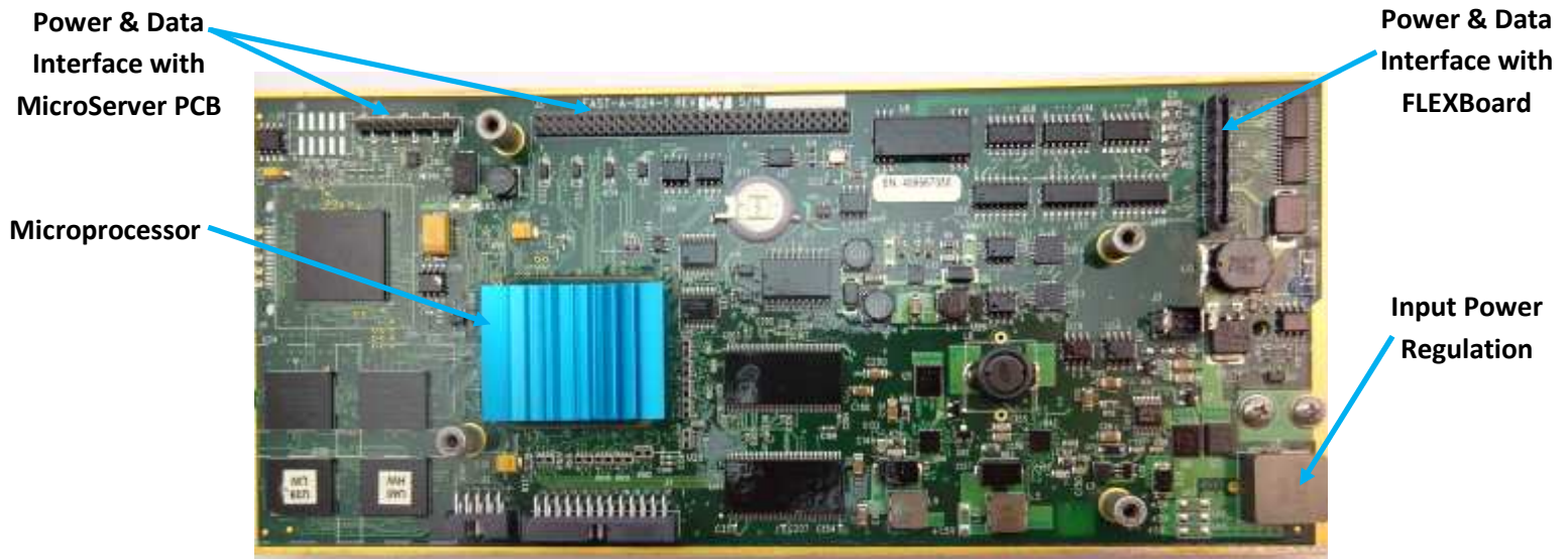
Figure 3: Control Processor Top View
