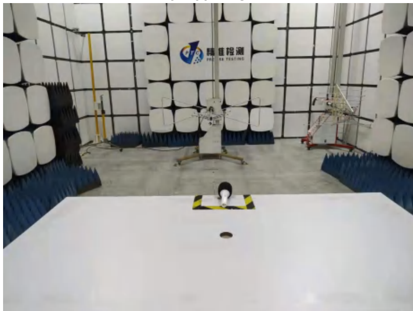
Radiated Spurious Emissions From 30M-1GHz
