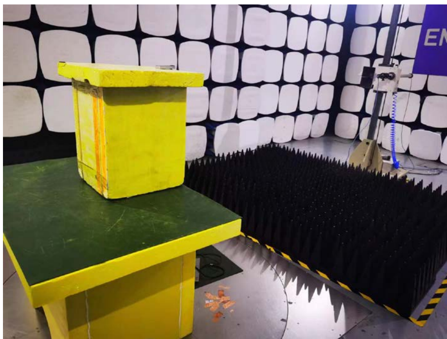
Spurious Emission Test Setup (Above 1GHz)
