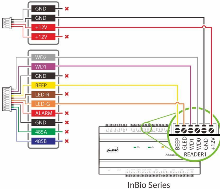
Figure 1-3 InBio Wiring
