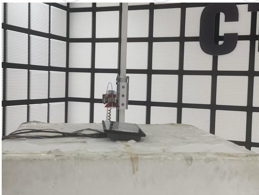
Radiated spurious emission Test Setup-2(1GHz to 18GHz)
