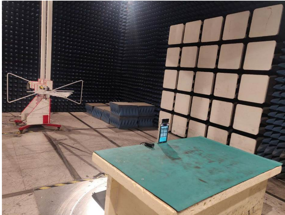
Spurious Emission Test Setup (30MHz-1GHz)
