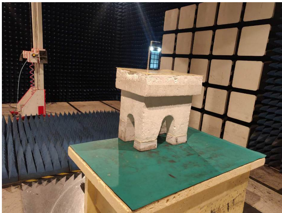
Spurious Emission Test Setup (Above 1GHz)
