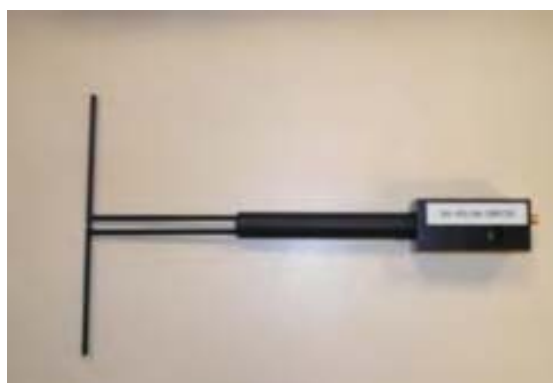
Figure 1 – Satimo COMOSAR Validation Dipole
