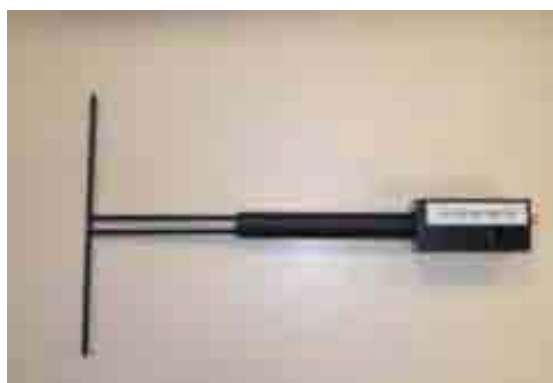
Figure 1 – Satimo COMOSAR Validation Dipole
