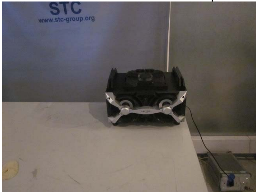
Measurement of Conducted Emission Test Set Up
