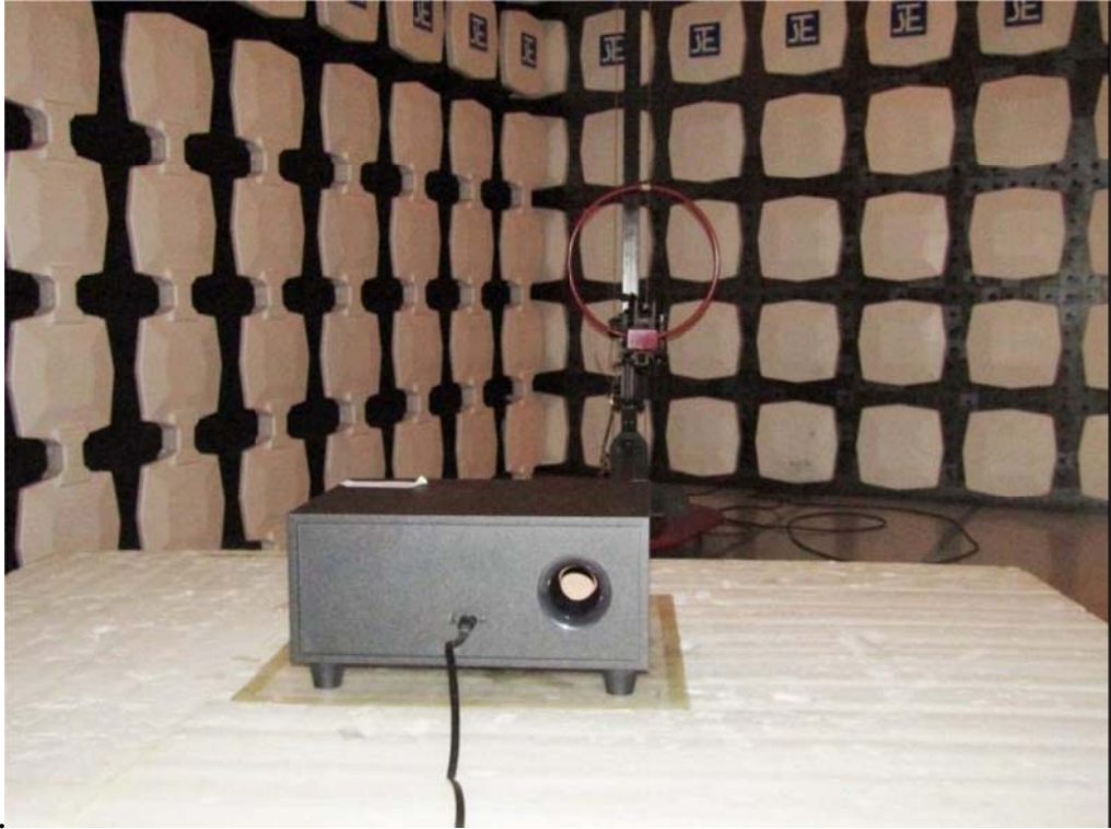
Measurement of Radiated Emission Test Set Up
