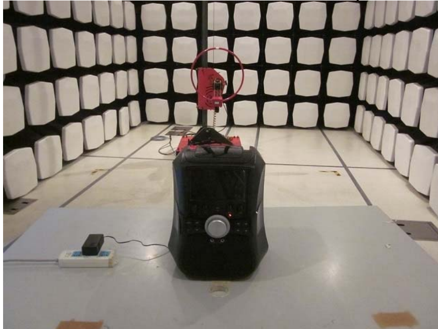
Measurement of Radiated Emission Test Set Up
