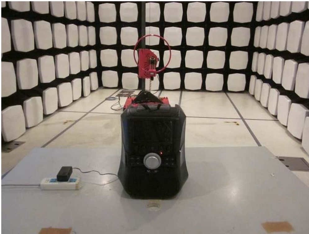
Measurement of Radiated Emission Test Set Up
