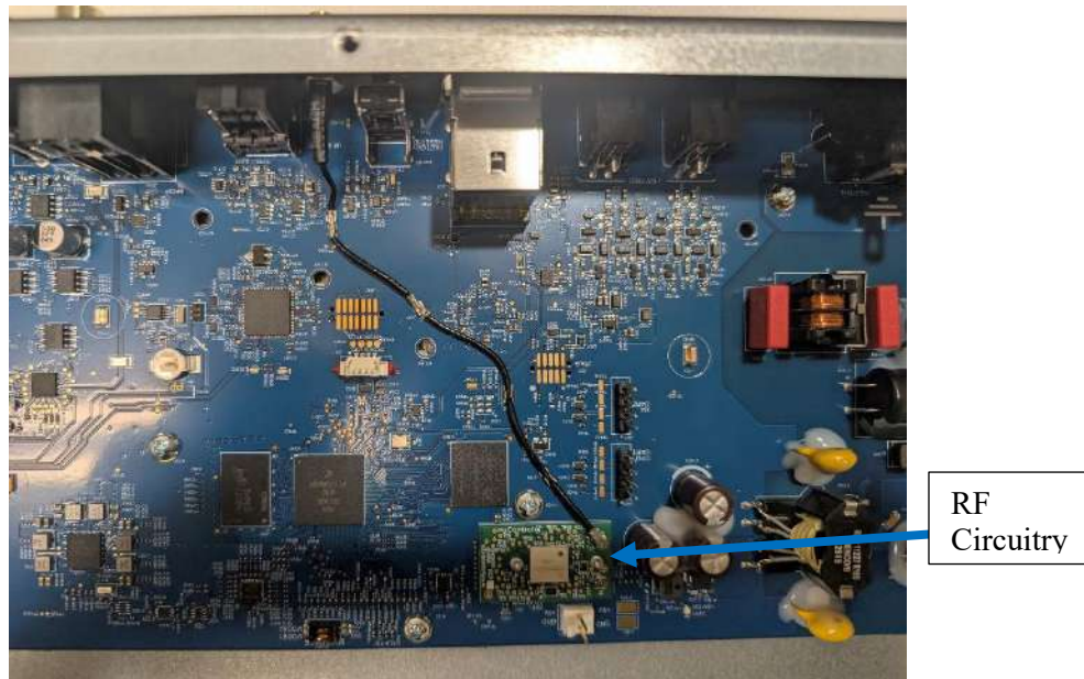
Photograph 16: Close-up View of the RF Circuitry in the Enclosure Showing Antenna Cable Routing
