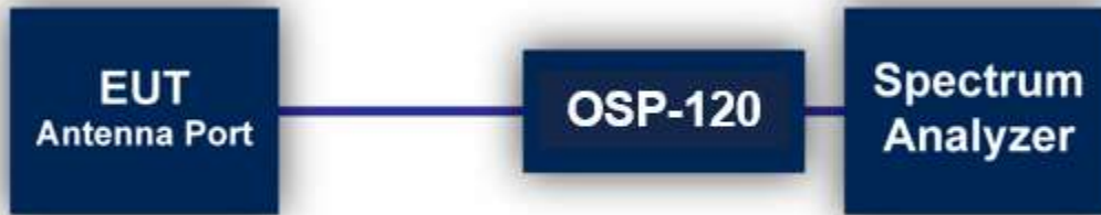
Figure 2: Direct Connection at the Antenna Port Test
