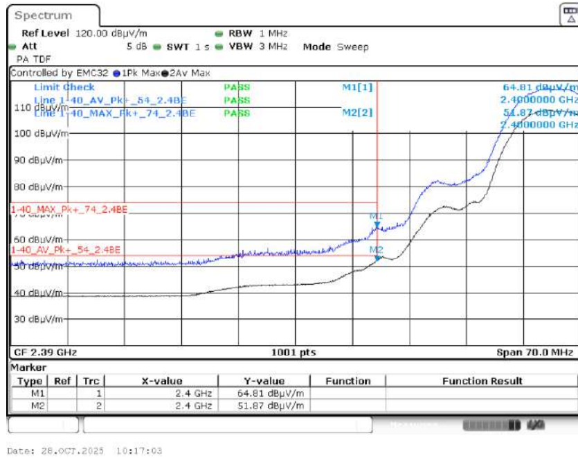
Graph 14: 2422 MHz Radiated Lower Band Edge Plot, Power Level 18
