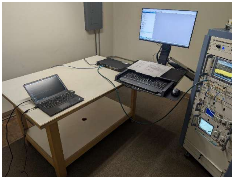
Photograph 7: Antenna-Port Conducted Emissions Configuration
