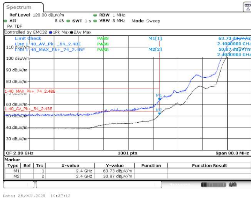
Graph 15: 2427 MHz Radiated Lower Band Edge Plot, Power Level 19
