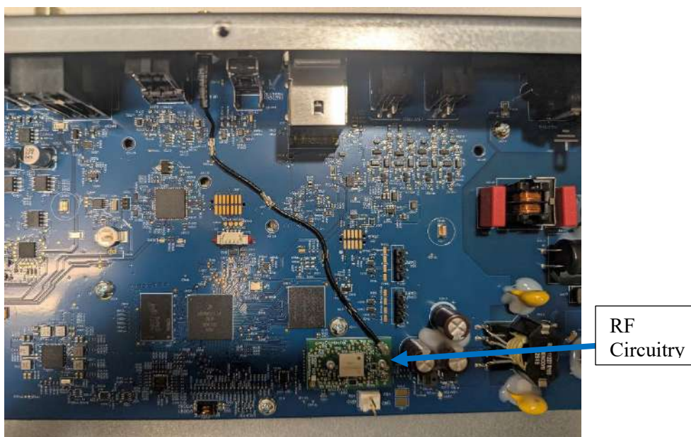
Photograph 15: Close-up View of the RF Circuitry in the Enclosure Showing Antenna Cable Routing
