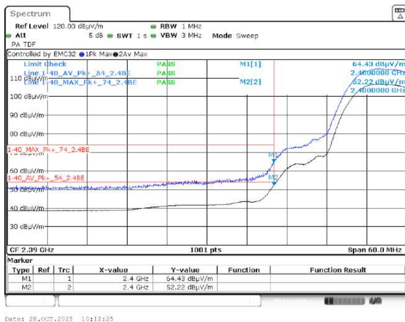
Graph 13: 2417 MHz Radiated Lower Band Edge Plot, Power Level 16
