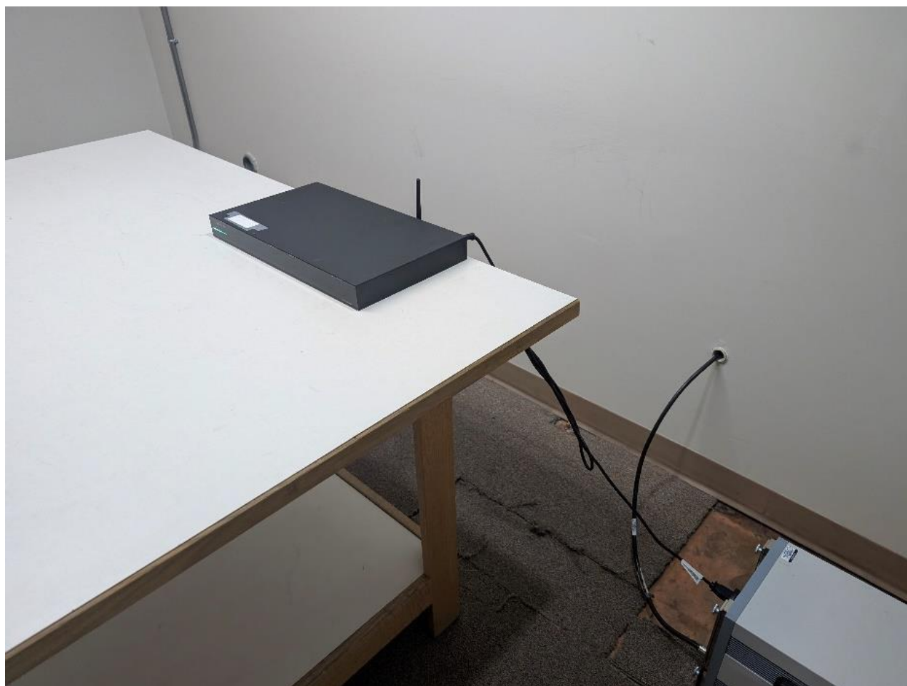
Photograph 5: Front View Conducted Emissions Worst-Case Configuration
