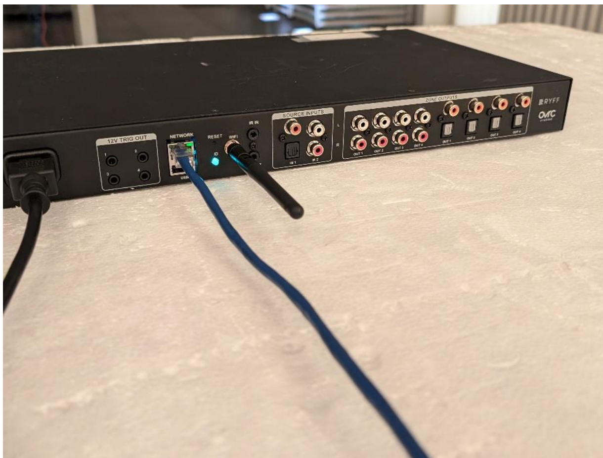
Photograph 4: Maximum coupling antenna position for Horizontal Measurements
