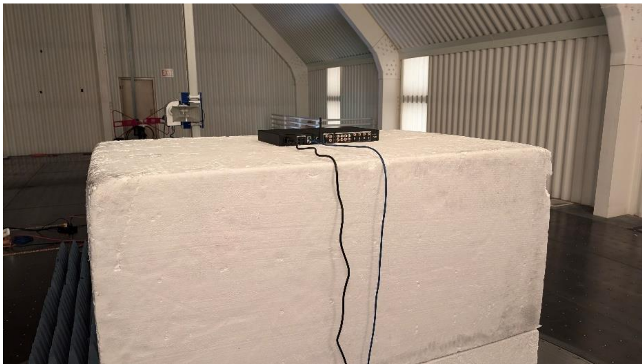
Photograph 2: Back View Radiated Emissions Worst Case Configuration
