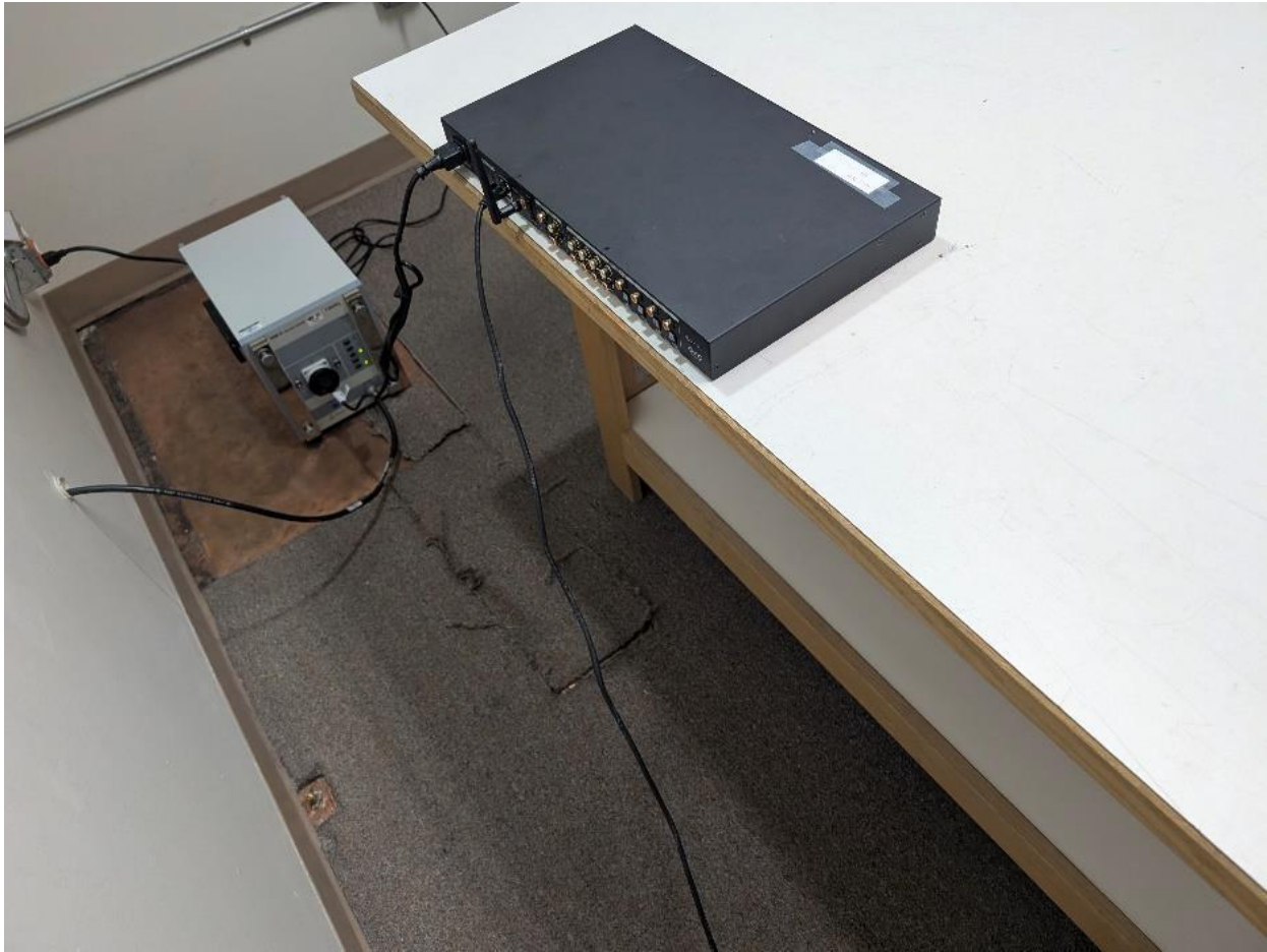
Photograph 6: Back View Conducted Emissions Worst-Case Configuration
