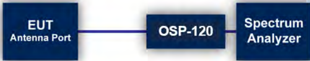
Figure 2: Direct Connection at the Antenna Port Test
