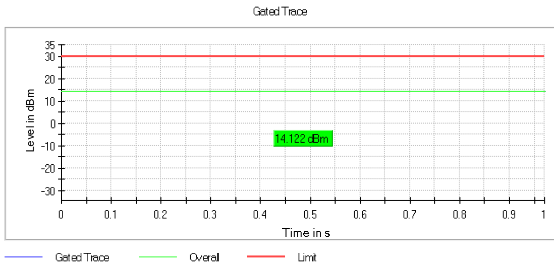
Graph 170: Gated Trace Power Transmitting at 5755 MHz (Power Level 19)
