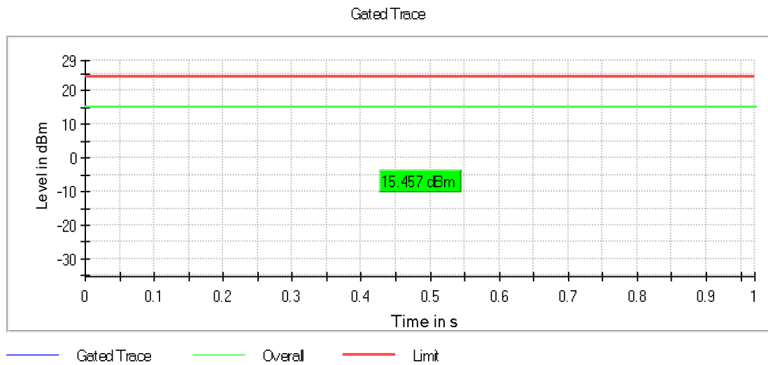
Graph 132: PM-G Power Transmitting at 5590 MHz (Power Level 20)
