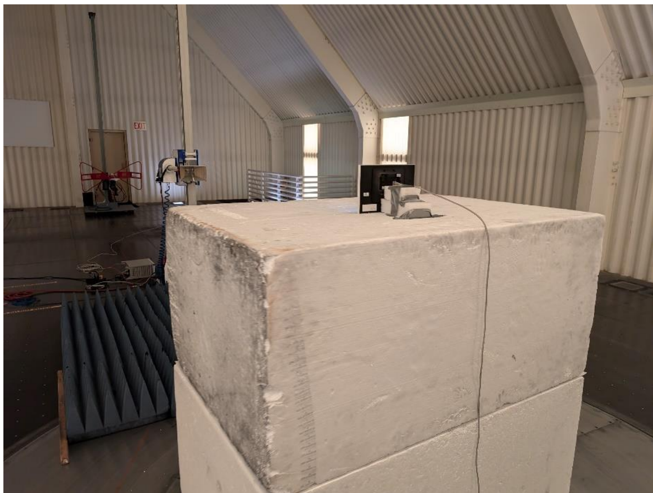
Photograph 2: Back View Radiated Emissions Worst Case Configuration, T5IW11
