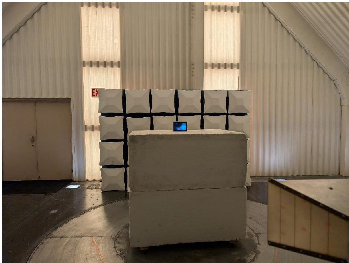
Photograph 1: Front View Radiated Emissions Worst Case Configuration, T5IW8
