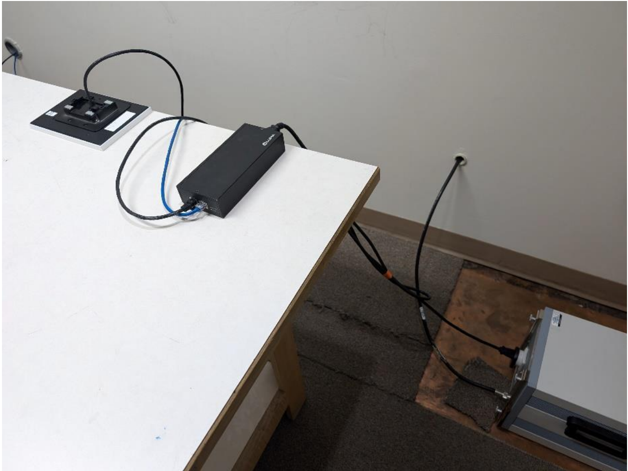
Photograph 3: Front View Conducted Emissions Worst-Case Configuration, T5IW8
