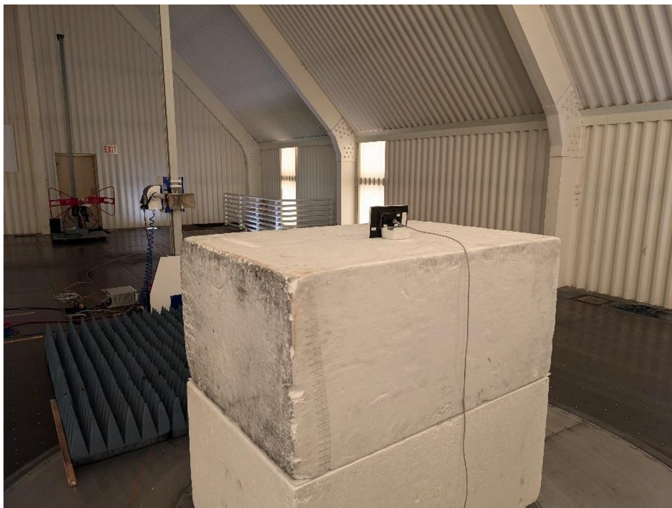
Photograph 2: Back View Radiated Emissions Worst Case Configuration, T5IW8
