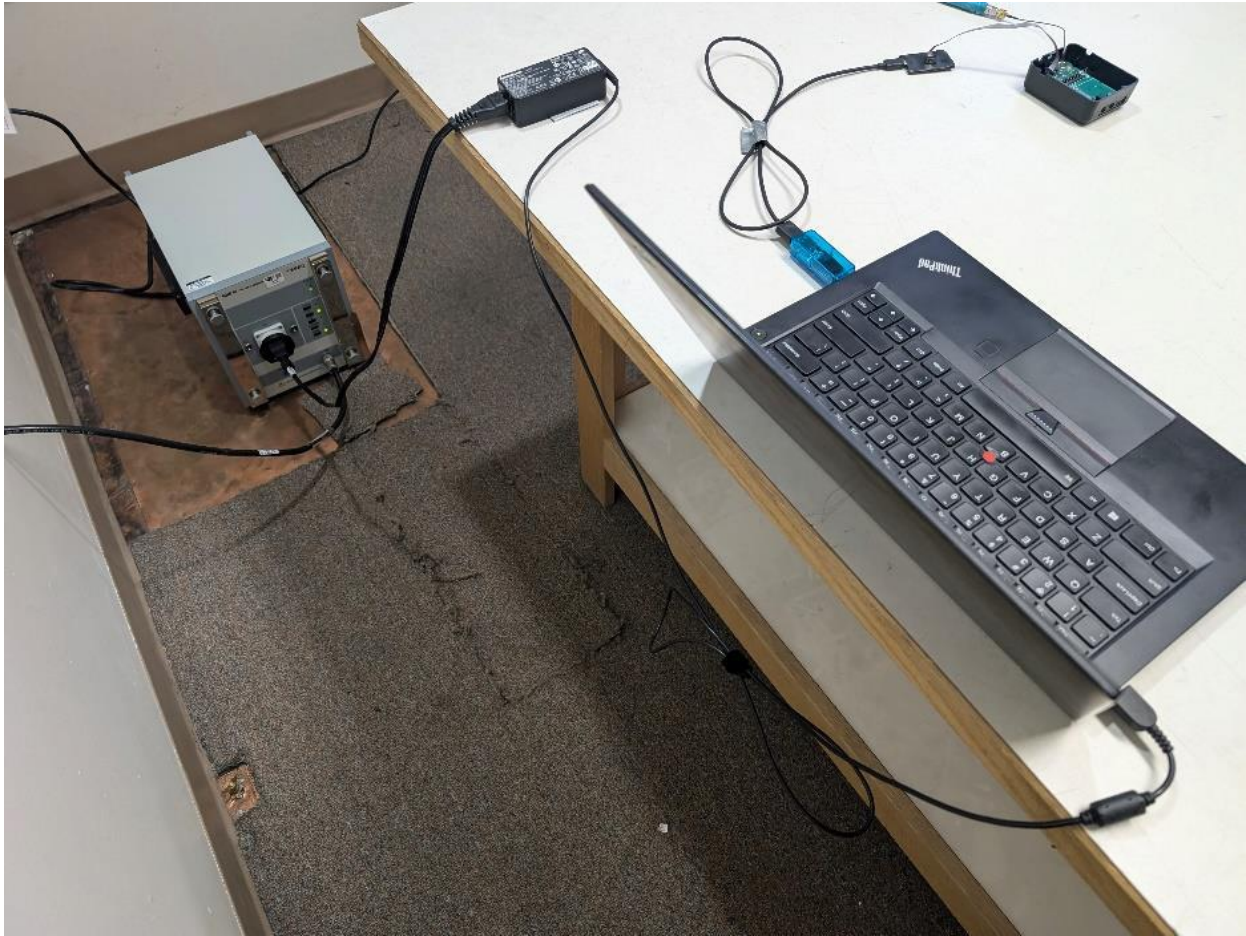
Photograph 8: Back View Conducted Emissions Worst-Case Configuration, C4-Z2C-V3
