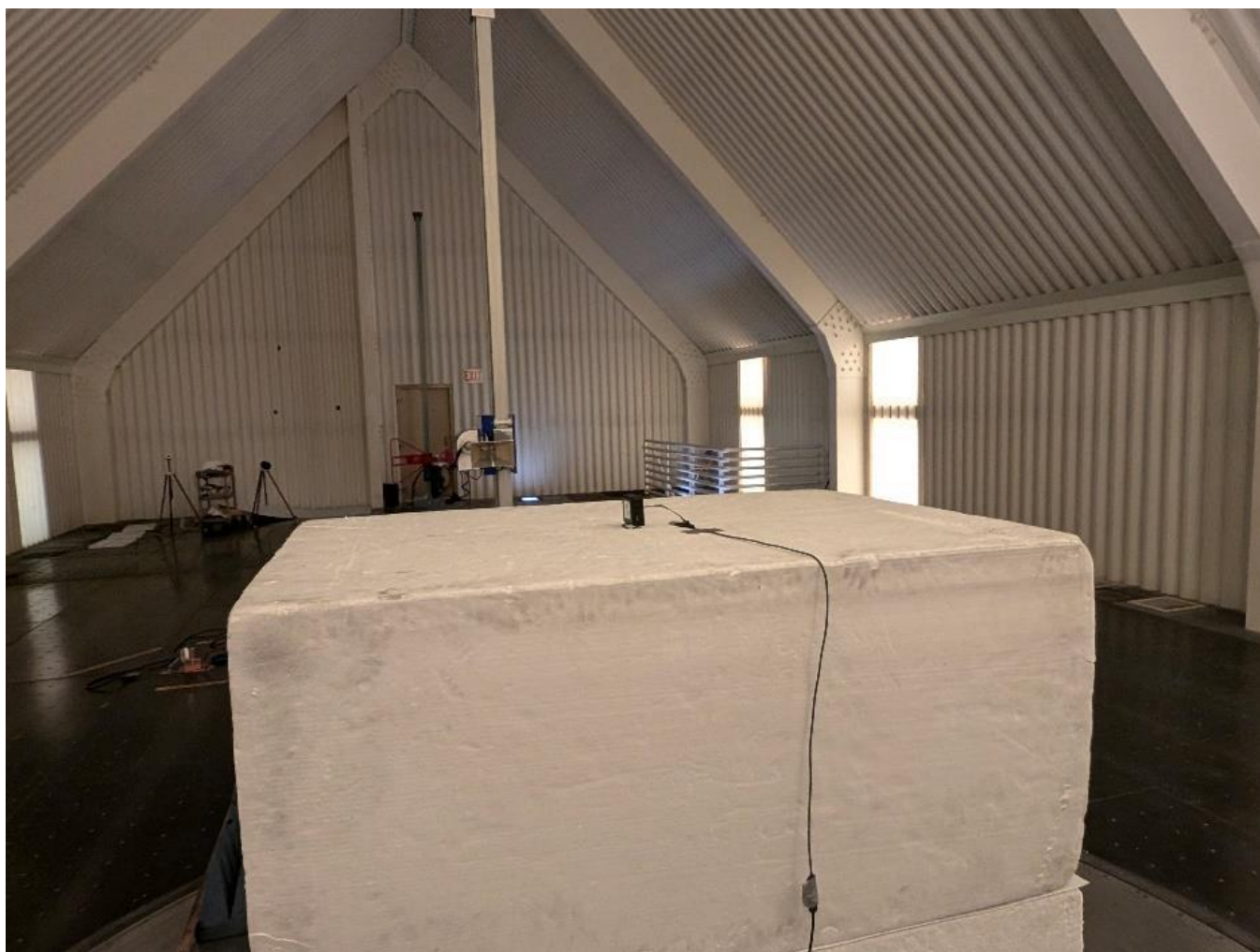
Photograph 2: Back View Radiated Emissions Worst Case Configuration, C4-Z2C-V3
