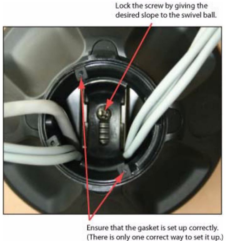
Figure 17 Routing the cables into the swivel
