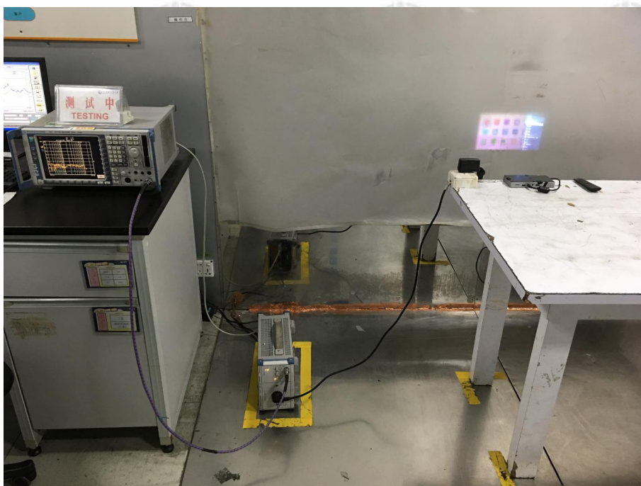
Conducted Emissions Test Setup
