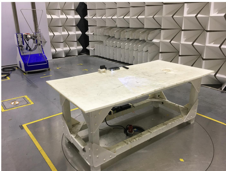
Radiated spurious emission Test Setup-2(30MHz-1GHz)
