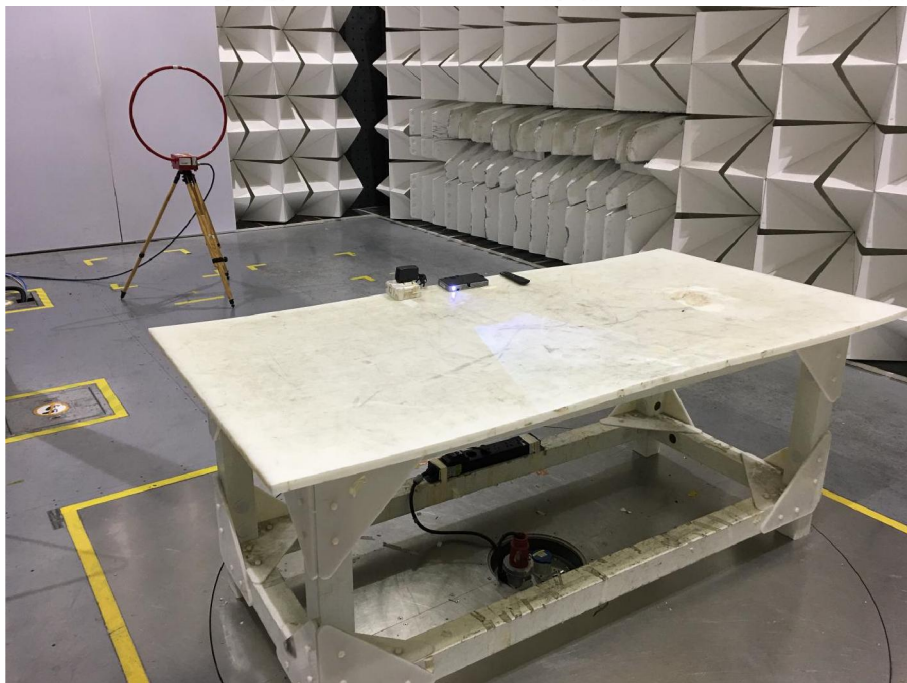
Radiated spurious emission Test Setup-1(Below 30MHz)
