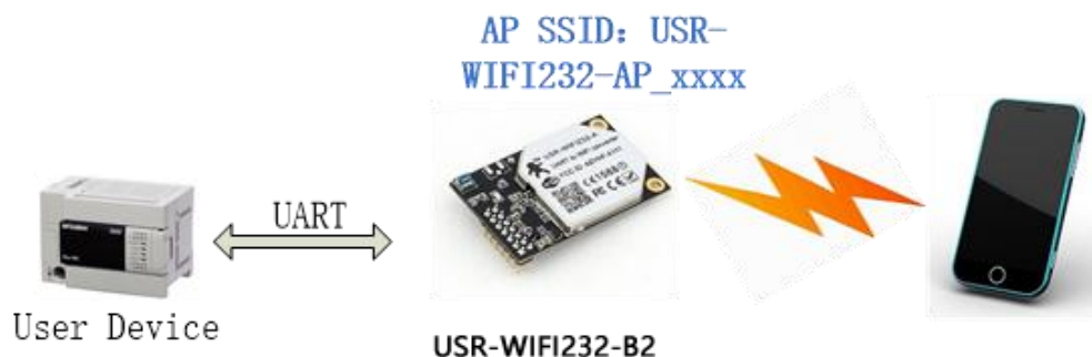
Figure 47 Wireless Control Application
