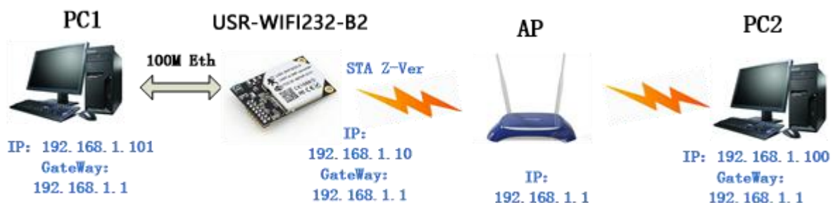
Figure 21 USR-WIFI232-B2 Ethernet Interface Networking (As STA, Z-Ver)
