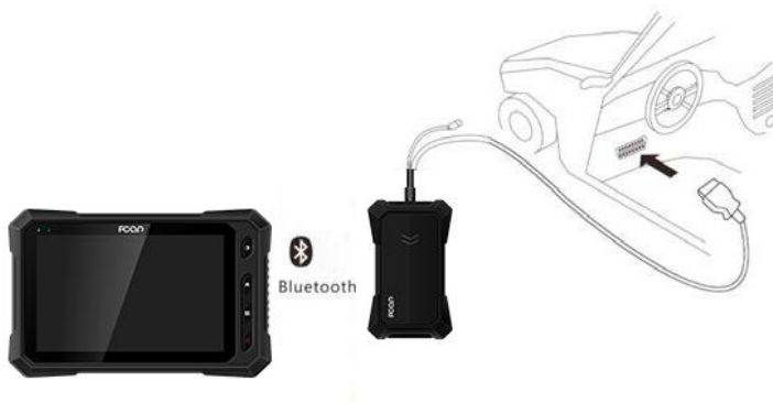
Figure 3.2-1 Connection of standard-OBD-II port
