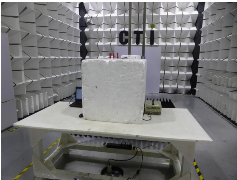
Radiated spurious emission Test Setup-2(Above 1GHz)
